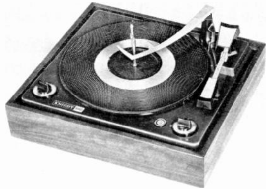
Knight KN-990 is four-speed automatic or manual player that intermixes different size records.
