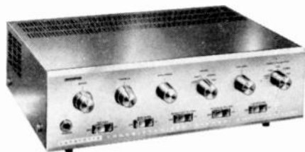
Lafayette KT-900WX is solid-state preamp-power amplifier, 120 watts music power, kit or wired.
