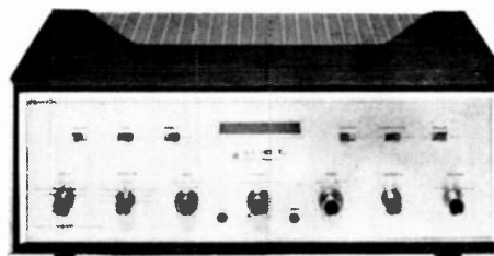
Scott 299D is integrated amplifier, rated at 40 watts per channel music power; below is solid-state type 4270, rated at 30 watts per channel.
