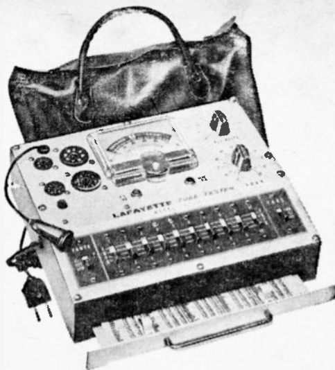
Fig. 22. Book-sized tube tester is inexpensive. This emission tester (Lafayette Radio Electronics) uses four-position slide switches for "free-point" tube-pin connections to prevent arborescence, when new tubes are introduced, over a period of many work years.
