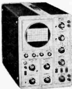
Fig. 21. This 5-inch DC scope by Heathkit has a good many features of scopes used in engineering laboratories.
