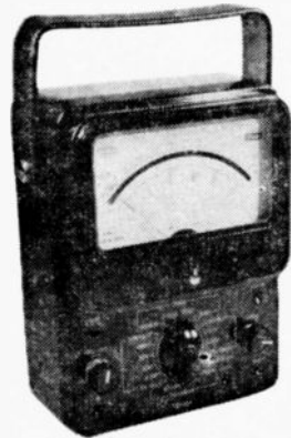
Fig. 12B. The mirrored scale improves accuracy of this Olson Electronics 100,000-ohm-per-volt instrument.
