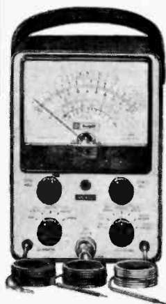
Fig. 16B. Audio (AC) VTVMs have fewer knobs than multimeter type. This EICO unit's low range is 1 millivolt or -60 db across 600 ohms.
