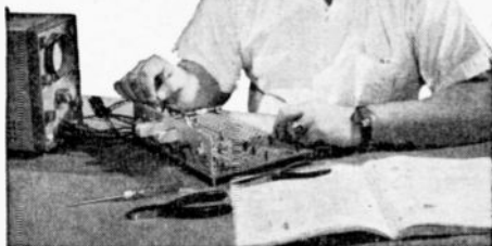
Transistor experiments on programmed breadboard— using oscilloscope.
