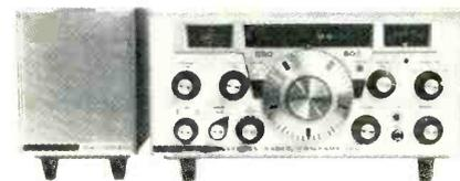
in bandwidth selections including 500, 2500, 5000, and 8000 Hz; r.f. gain control and r.f. input attenuator; selectable tuning ratio of either 10 kHz or 50 kHz per knob revolution; passband tuning of i.f. filter; built-in crystal calibrator; S meter; variable b.f.o.; reception modes; AM, CW, lower and upper
