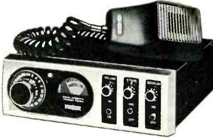
channel rejection -40 dB; selectivity -30 dB at ±11 kHz; image response -45 dB; delta tune ±1 kHz; dual-conversion receiver; audio output 3 W at 10% dist.; spurious emissions -60 dB at all frequencies above 2nd harmonic; spurious response -50 dB; 100% max. modulation; p.a. facilities; a.n.l.; switchable noise blanker; squelch; external speaker jack; S/RF meter; 8" D x 6" W x 2" H ..... \$189.00
