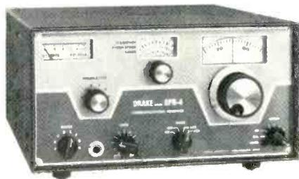
supplied by manufacturer); dual-conversion; direct frequency readout; three built-in bandwidths, corresponding to mode of reception; 400 Hz for CW, 2400 Hz for SSB, and 4800 Hz for AM; built-in speaker; notch filter; 100-kHz calibrator and i.f.-type noise blanker available as optional extras; S meter;
