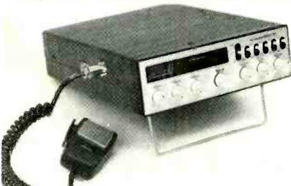
sensitivity 0.5  $\mu$ V (AM), 0.2  $\mu$ V (SSB); selectivity -50 dB (AM), -60 dB (SSB)  $\pm 10$  kHz; adj. channel rejection -60 dB; p.a. capability; adjustable delta tune & squelch; a.n.l.; adj. a.n.l. control; SWR meter; Tx indicator light; 120 V a.c. or 12 V d.c.; 12 7/16" D  $\times$  8 $\frac{7}{8}$ " W  $\times$  2 $\frac{3}{4}$ " H ..... \$279.99
