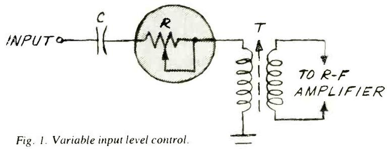
Fig. 1. Variable input level control.
