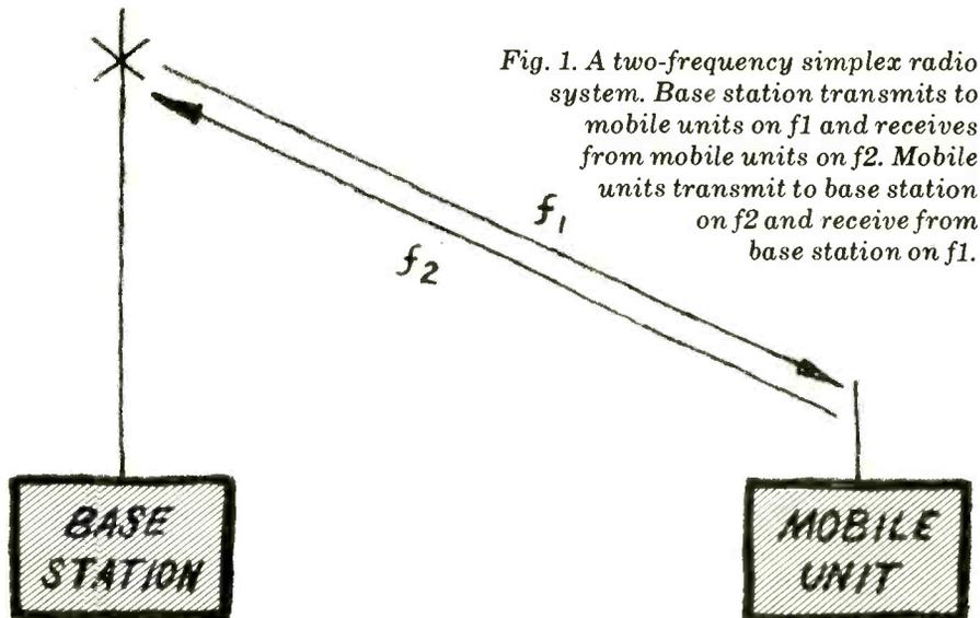
*Fig. 1. A two-frequency simplex radio system. Base station transmits to mobile units on  $f_1$  and receives from mobile units on  $f_2$ . Mobile units transmit to base station on  $f_2$  and receive from base station on  $f_1$ .*
