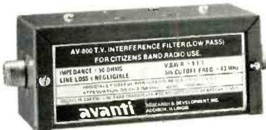
**AV 800 TV interference filter (low pass)** installs in CB antenna line and is especially useful for interference on CH2 and 5 of poorly filtered TV receivers.
