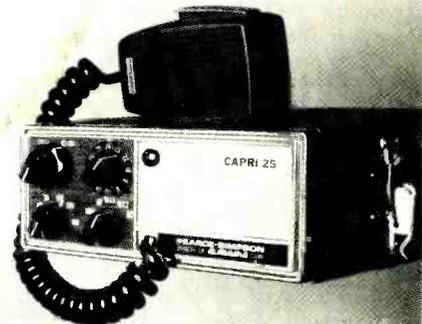
dB; receiver sensitivity 0.7 µV for 12 dB SINAD at 60% system deviation; audio power output 2.5 W at 10% dist.; spurious rejection -50 dB; selectivity ±7.5 kHz at 6 dB down, ±25 kHz at 60 dB down; comes with mounting bracket; 13.6-V d.c. negative ground; 11" D x 6½" W x 3" H ..... \$419.95
