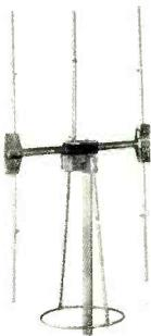
num tubing construction; hubs of weather-resistant Cylolac; forward gain 11 dB over isotropic; rejection 40 dB plus signal drop front-to-back; imp. 50-52 ohms; boom length 10 1/2 ft; vertical beam; v.s.w.r. 1.3:1; turning radius 63 in; power multiplication 12.6 times; light- to medium-duty rotor can be used (including inexpensive TV rotors); weight 14 lbs ..... \$79.95
