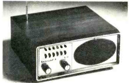
33-48 MHz, 146-174 MHz, 450-470 MHz, 470-512 MHz; electronically switched antenna; LED channel indicators; 20 ch/sec automatic scanning; single manual/scanner switch; quartz crystal filter; lockout switches; front-mounted speaker; sensitivity 0.6 µV for 20 dB S/N on U & T bands; audio output 2 W rms; 117-V a.c., 10 W; 9" D x 7" W x 3 1/2" H ..... \$159.95
