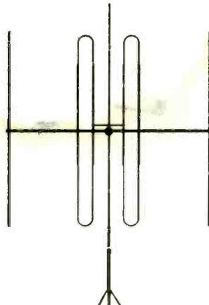
ment; outer director and reflector elements spaced to optimize beam gain; gain 9.3 dB over an isotropic; v.s.w.r. 1.5:1; discrimination 20 dB max. rejection; wind loading 100 mph +; height 20 feet; width 14 feet; mast size 2" o.d.; weight 32 pounds ..... \$119.95
