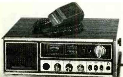
dB; delta tune  $\pm 1.5$  kHz; dual-conversion receiver; audio output 2.2 W at 10% dist.; spurious emissions -60 dB; spurious response -40 dB; 95% max. modulation; p.a. facilities; switchable a.n.l.; squelch; external speaker jack; S/Rf meter; r.f. gain control; on-the-air and Tx indicator lights; 11 1/2" W x 9" D x 4" H ..... \$249.95
