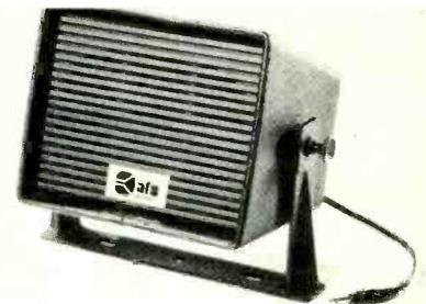
rotation of speaker and/or bracket; 3 $\frac{1}{2}$ " weather-proof-cone speaker; power handling 5 W rms; response 150-10,000 Hz; imp. 8 ohms; 6-ft cord with mini-plug; 5 $\frac{1}{4}$ " W  $\times$  4 $\frac{1}{2}$ " H  $\times$  4 $\frac{1}{4}$ " D ..... \$17.95
