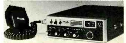
delta tune range ±1.5 kHz; combination meter for power output, SWR or S meter functions; p.a.; a.n.l.; adjustable squelch; r.f. gain; audio output 4 W at 10% dist.; PTT mike; requires 13.8-V d.c. positive or negative ground; 9 1/4" D x 7" W x 2 3/8" H ..... \$250.00
