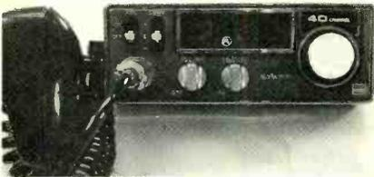
cent channel rejection -50 dB; selectivity -50 dB at 3 kHz, -60 dB at 10 kHz; image response -60 dB; delta tune ±1 kHz; dual-conversion receiver; 3 W audio output at 10% dist.; spurious emissions -60 dB at any frequency; spurious response -60 dB; frequency tolerance ±0.003%; 100% max. modulation; p.a. facilities; built-in a.n.l.; squelch; external speaker jack; S/RF meter; LED digital channel indicator (flashes on Ch 9); 13.8 V d.c.; 7 7/8" D x 5 3/4" W x 2 1/4" H ..... \$149.95
