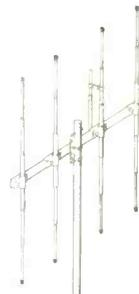
struction, surface area 4.4 sq ft, wind loading 118 lbs at 80 mph, gamma feed, 50 ohm feedpoint imp., gain over isotropic 12.6 dBi, front-to-back ratio 23 dB, front-to-side 30 dB, half-power beamwidth 53 degrees E plane, max. s.w.r. 1.25:1 at 36 ft, polarization same as mounting plane, square boom, self-aligning elements, assembled weight 12.6 lbs ..... \$61.95
