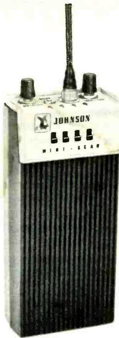
*E.F. Johnson's four-channel portable scanning receiver.*
