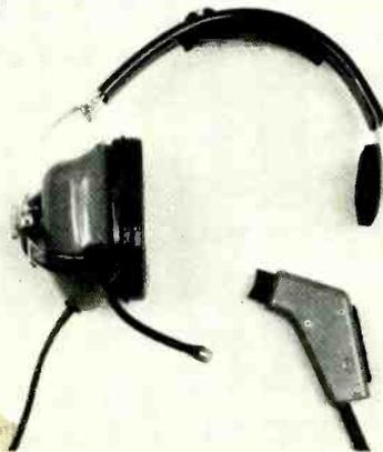
built-in FET transistor amplifier; frequency response 200-6000 Hz; relay or electronic switching capability; palm-held talk switch has Velcro pad for easy mounting; self-adjusting headband with spring-flex hinge; reversible for left or right ear; powered by 7-V TR-175 battery ..... \$69.95
