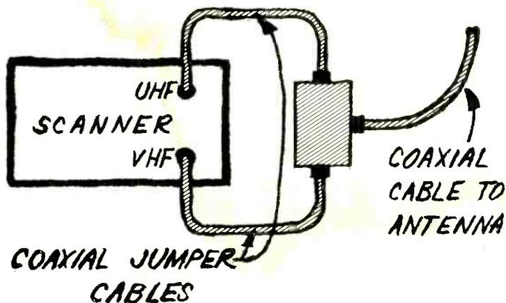
Fig. 2. Splitter permits use of one multi-band antenna with scanner having separate VHF and UHF antenna jacks.
