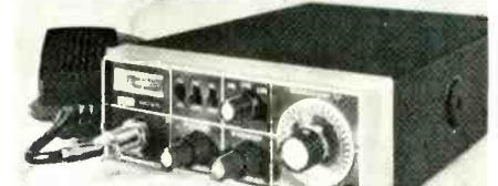
p.e.p. (SSB); receiver sensitivity 1 μV at 10 dB S + N/N, 0.5 μV at 15 dB S + N/N; adj. channel rejection -65 dB; single-conversion receiver; audio output 3 W at 10% THD; switchable noise blanker & noise limiter; clarifier; power out/S meter; r.f. gain control; adjustable squelch; p.a. facilities; PA/Paging function with optional external speaker; 9.1" D x 6.6" W x 2.3" H ..... \$379.95
