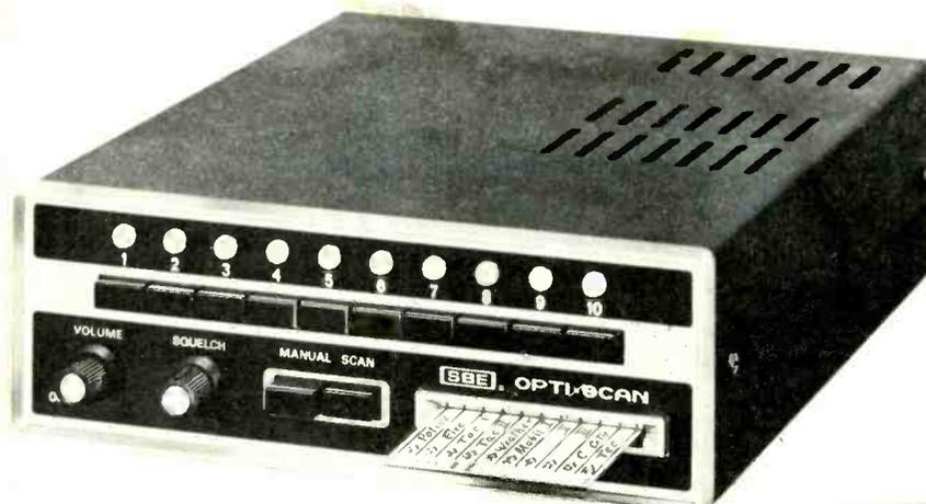
*This 10-channel scanner from SBE can be set to any ten of some 16,000 channels in the 30-50 Mhz, 150-170 MHz, and 49-510 MHz bands. Channels to be scanned are selected with a do-it-yourself programmed card. Other channels can be scanned by inserting a different card into receptacle on front panel.*
