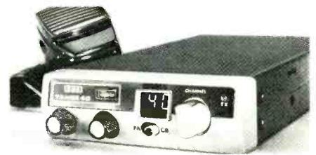
adj. channel rejection -60 dB; dual conversion receiver; digital LED channel readout; a.n.l.; volume and squelch controls; requires 13.8-V d.c.; 7.25" D x 4.5" W x 1.375" H ..... \$179.95
