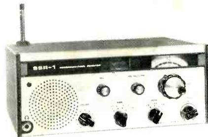
synthesized; selectable sidebands; preselector; clarifier; built-in speaker; S meter; headphone jack; telescoping antenna; coarse and fine tuning controls; built-in 117/234 V a.c. power supply; automatically switches to internal battery pack if a.c. power fails; on-off pushbutton for reduced current drain on d.c. operation; 5 $\frac{3}{4}$ " H  $\times$  13" W  $\times$  10 $\frac{1}{2}$ " D. .... \$350.00
