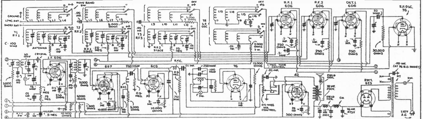
Wiring diagram for the new "Silver" super-het for short and broadcast waves.
