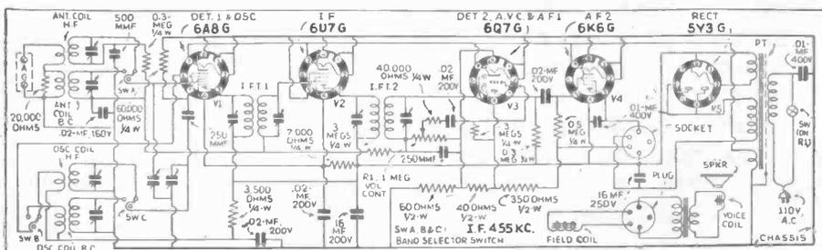
Fig. 2. Schematic diagram of the Crosley "Teletune" Compact Five.
