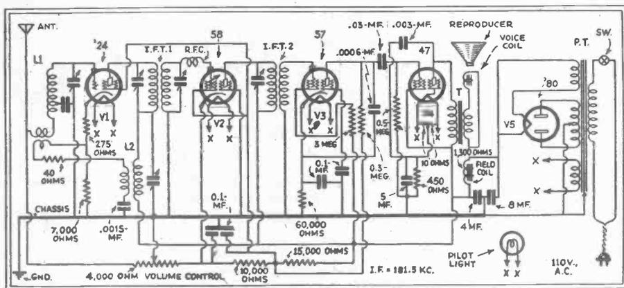
Fig. 1 Schematic circuit of the Crosley Book Case Receiver pictorially illustrated in Fig. A.
