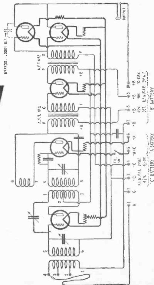
The wiring diagram, showing the connections of the five tubes, illustrates the method of combining R.F. amplification with regeneration.
