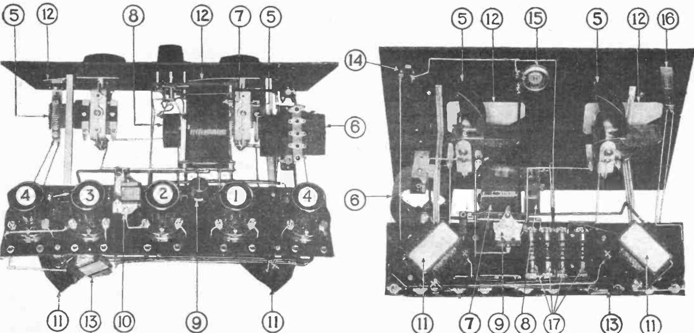
Above are shown two views of this receiving set. No. 1 is the R.F. tube socket; 2, the detector tube socket; 3 and 4, A.F. amplifier tubes, two of which are in parallel; 5, variable condensers .0005- $\mu$ f.; 6, antenna coupler; 7, R.F. transformer; 8, tickler coil; 9, neutralizing condenser; 10, grid leak and condenser; 11, A.F. transformers; 12, shielding; 13, by-pass condenser; 14, filament switch; 15, rheostat; 16, jack; 17, automatic filament adjusters.
