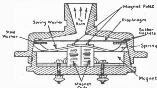
FIG. 26-9.—Cross-section view of a typical horn-type iron-diaphragm loud speaker unit, showing the relative arrangement of its parts. A disassembled unit of this kind is illustrated in Fig. 26-10.
