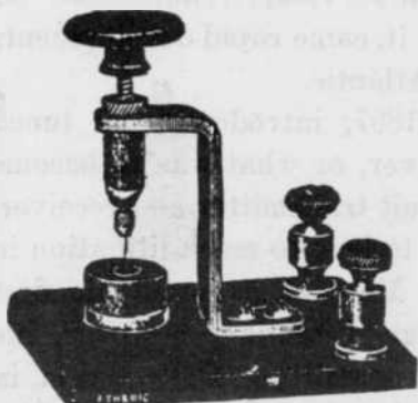
Electrolytic detector invented by Fessenden. It is probably the most sensitive of all detectors excepting the audion and the valve detectors. It consists of a carbon cup connected to a binding post and an adjustable standard which holds a very small hair-like platinum wire which dips into a 20% diluted solution of nitric acid. The high resistance of this acid detector is somewhat reduced by incoming wireless waves and when a telephone is shunted around it, the varying resistance is sufficient to vibrate the diaphragm but not strong enough to work a telegraph relay. When a potentiometer and battery are connected with the electrolytic detector and telephone, the sensitiveness is increased. The electrolytic detector is capable of operation with about three hundred micro-ergs; the magnetic detector is capable of operation with about four hundred micro-ergs; the silicon and most crystal detectors with about one thousand micro-ergs, and the manufactured carborundum detector with about nine thousand micro-ergs. Notwithstanding this very considerable difference in the sensitiveness of the electrolytic and carborundum detectors as measured by the C. G. S. system of units, in the actual practice of wireless telegraphy the receptive difference is hardly perceptible over similar distances. A great deal depends upon the adjustment of the detector which is a "cut and try" procedure until the most sensitive point is arrived at which will best respond to incoming signals.
