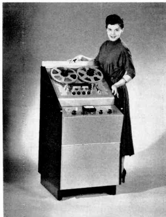
New Ampex tape recorder features 30-degree slope on both tape transport and control sections. The two-speed machine is designed for easy recording and servicing.
