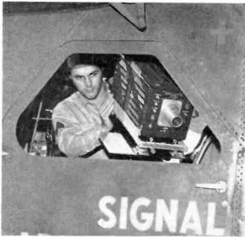
This shows the manner in which television camera is mounted in an L-20 observation airplane for combat aerial reconnaissance.
