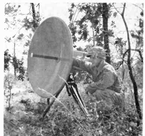
This parabolic reflector is the microwave transmitting antenna used by Tactical Relay Unit to send pictures to the Command Post.
