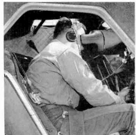
Internal shot of experimental television unit, aboard L-20 aircraft, with cameraman shown monitoring picture in view finder.
