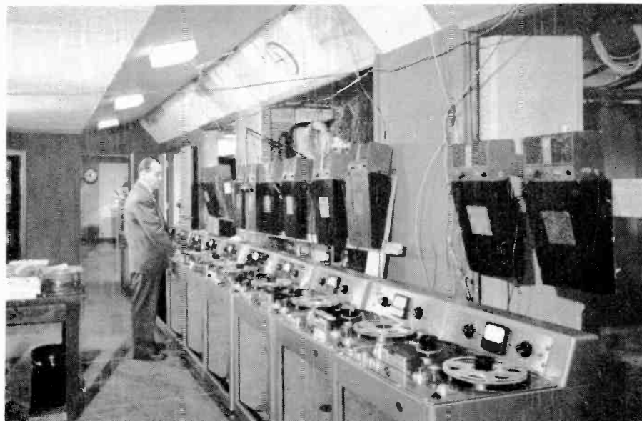
BILL O'BRIEN, recording technician at a bank of Ampex tape recorders, used prior to their permanent installation in recording booths.
