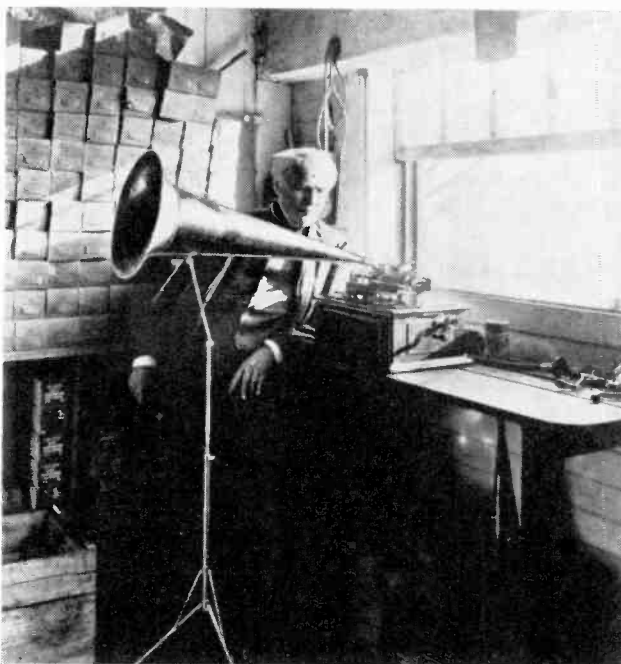
Thomas Alva Edison shown in his lab at Menlo Park, N. J., in 1906, listening to his new Triumph Phonograph. This device was unique in being the first phonograph containing a triple spring motor.
