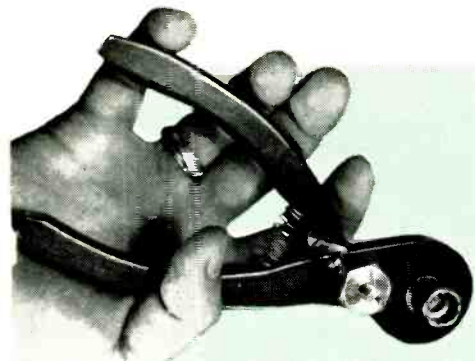
(above) A simple hand squeeze is translated into rotating motion by the ratcheted Plench.
