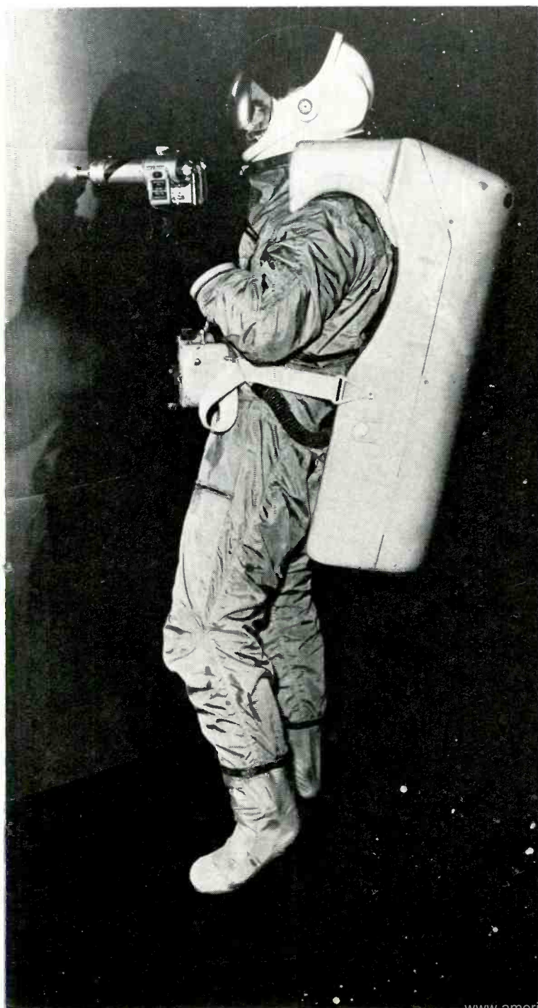
Hanging in a simulated space-world, an engineer demonstrates use of the power Zert. The back pack contains life-support systems to provide oxygen, heat and air conditioning.
