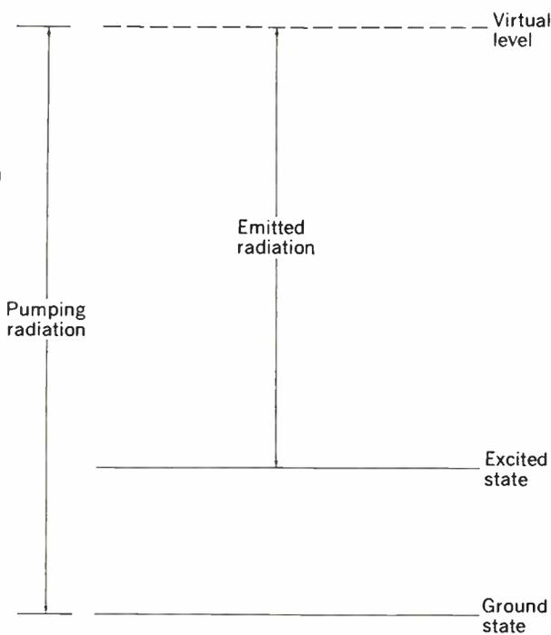
Fig. 6. Representation of energy levels in a Raman maser. This system resembles qualitatively a three-level maser, one of the levels being "virtual," or not characteristic of the molecule, when no field is present.
