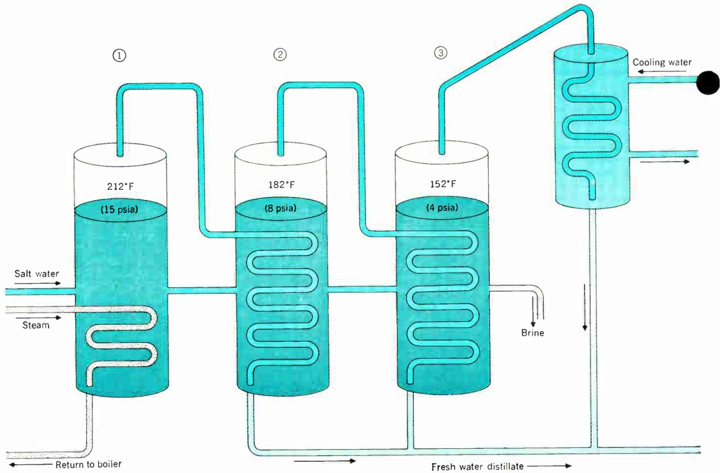
Fig. 3. Flow diagram of a triple-effect distillation system that is commonly used to produce boiler makeup feed.
