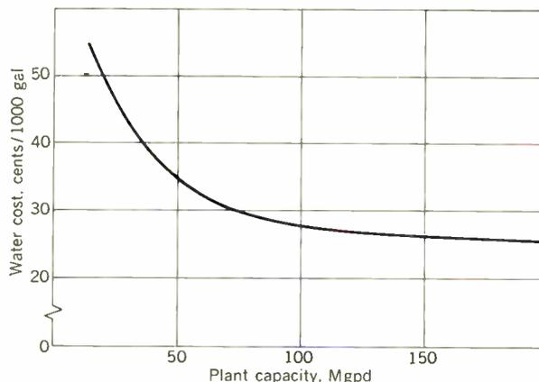
Fig. 12. Graph showing the estimated water costs for a HTGR dual-purpose plant. Mixed plant ownership, an 80 percent capacity factor, full back-pressure turbine, and 250° F brine temperature are assumed.
