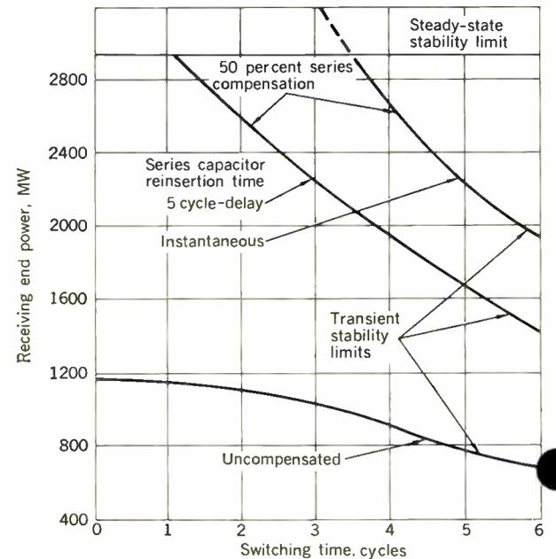
Fig. 8. Increased EHV line loadings with series capacitors.
