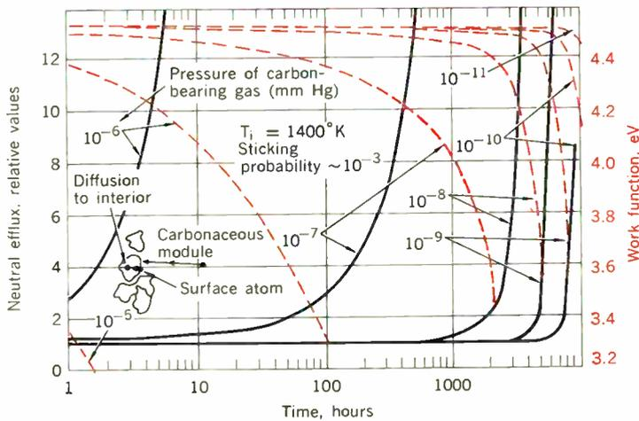
Fig. 18. The effect of a carbonaceous atmosphere on the work function and neutral efflux of a tungsten ionizer, vs. time of exposure of the tungsten to the carbon-bearing gas, with partial carbon gas pressure as parameter.
