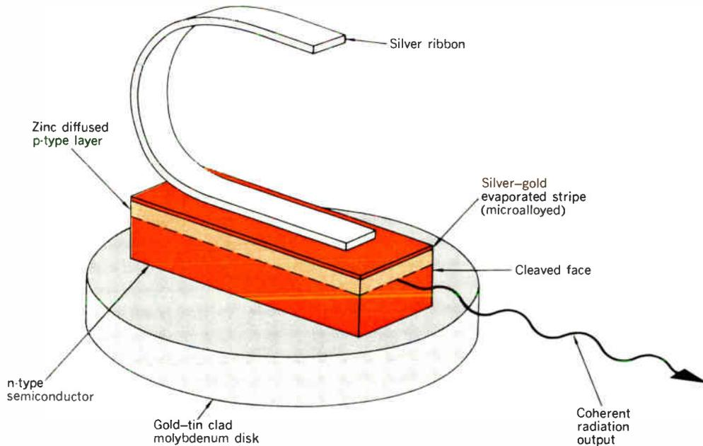
Fig. 5. Schematic diagram of a gallium arsenide (injection, or semiconductor) laser. A small voltage applied between the silver ribbon and the molybdenum disk can produce maser oscillations with resulting emission of coherent infrared radiation.
