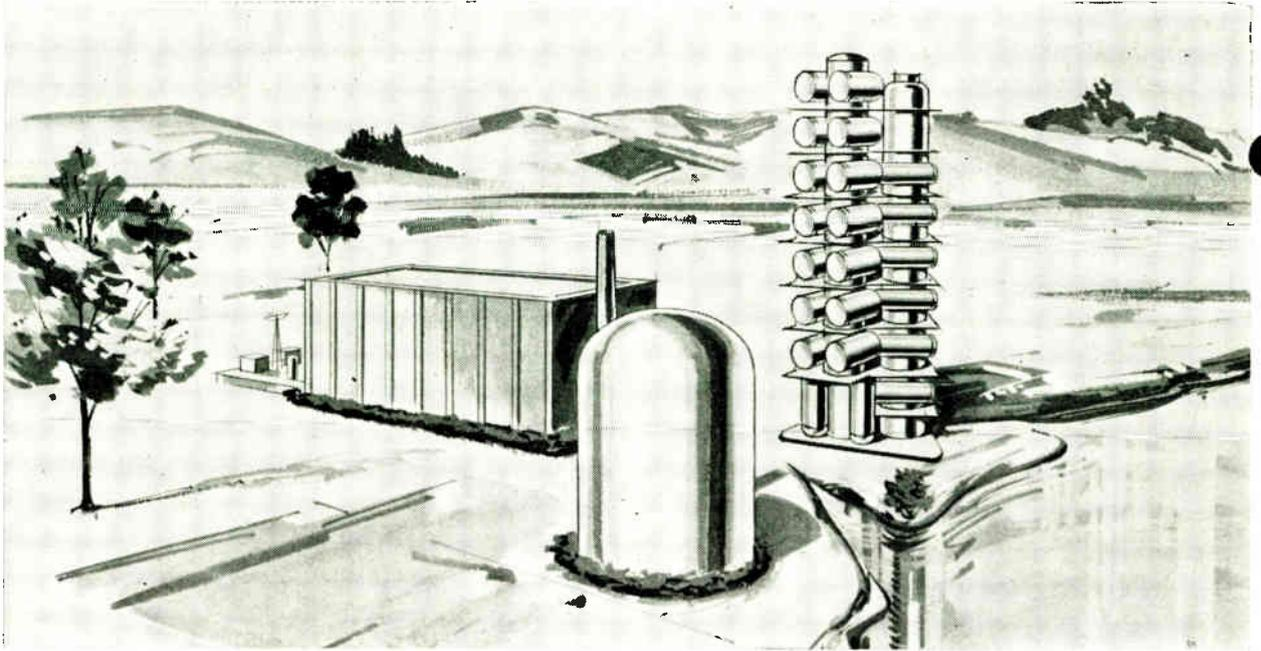
Fig. 13. Architectural rendering of a typical dual-purpose sea water conversion complex. In the foreground is a nuclear reactor which supplies heat for the desalting process. At the left is the power station, and the multistage flash evaporating unit is shown at the right.
