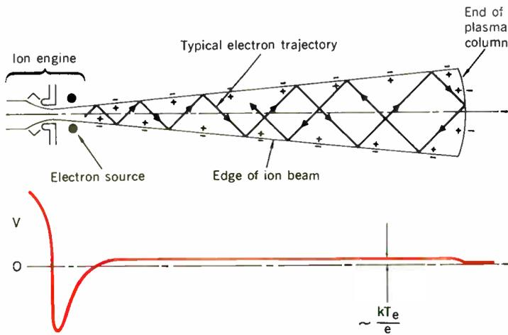
Fig. 16. Diagram of neutralization of an ion beam by electrons. Expected potential diagram is at the bottom.
