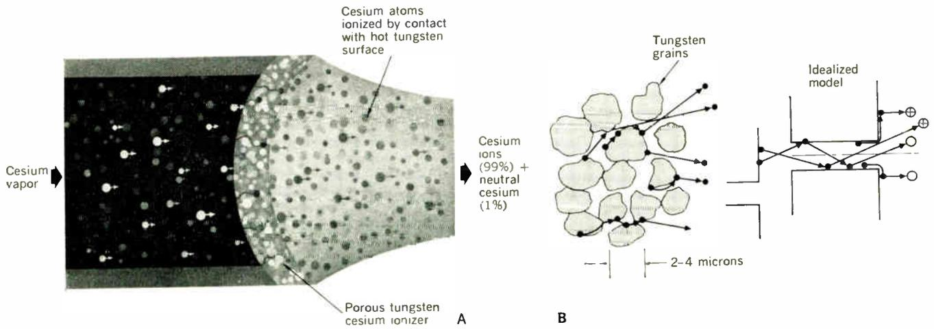
Fig. 4. Cesium contact ionizer, formed of porous refractory metal. A—Typical configuration. B—Surface diffusion and molecular transport mechanisms resulting in ion and neutral atom evaporation from the pore and the surface, using the actual granular structures and an idealized model composed of cylindrical pores.
