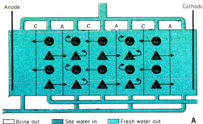
Fig. 6. Sectional view of electrodesialysis cells, showing the ion dissociation of sea water.
