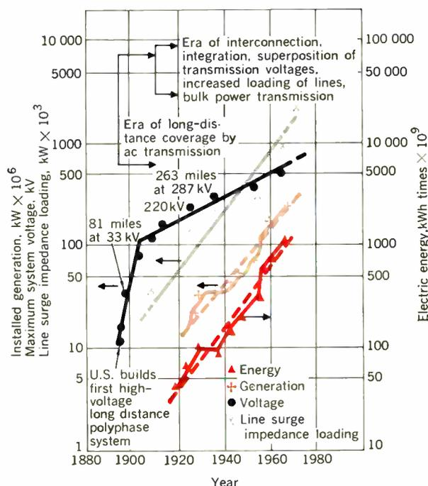
The historical trend of maximum sizes is shown in Fig. 2, which also demonstrates the increasing complexity of manufacture, assembly, testing, and shipment of EHV units. Factory assembly and testing assure the reliability needed in the super sizes now foreseen. Therefore, field assembly should be resorted to only as a last alternative. This requirement will establish a trend to single-phase units in these EHV sizes.
