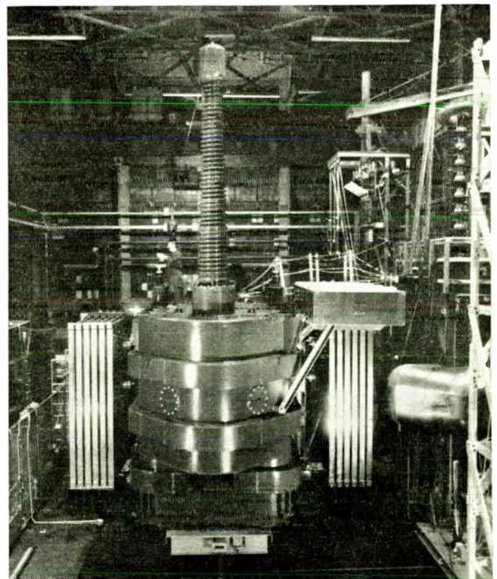
Voltage control will be accomplished by using switched shunt reactors and capacitor blocks at tertiary voltages. This practice provides a coarse control to compensate for the rise and fall of EHV voltage levels with line loading fluctuations.
