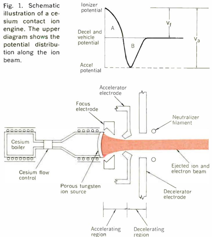
placed at one end of the discharge chamber. In the contact ion engine, ions are created by contact ionization of the propellant (cesium) with a hot ionizer electrode and are accelerated in a geometry of electrodes roughly similar to conventional electron guns used in traveling-wave tubes.
