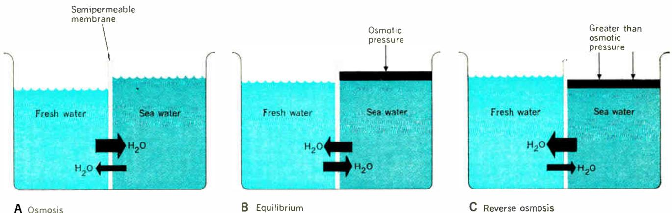
Fig. 8. A—Illustration of a simple osmotic system in which diffusion proceeds through a semipermeable membrane that separates solutions of sea water and fresh water. B—An equilibrium condition exists when pressure equal to the osmotic pressure is applied to the more concentrated solution. C—When pressure greater than the osmotic pressure is applied on the salt solution, reverse osmosis occurs.
