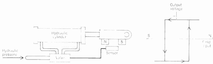
FIGURE 3. Stroke adjustment of a hydraulic cylinder.
