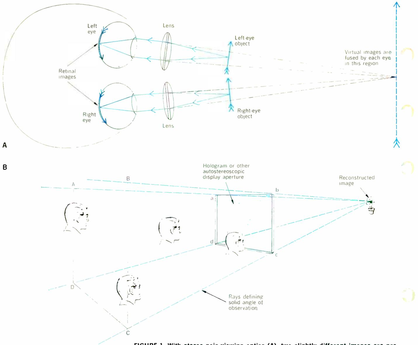
**FIGURE 1.** With stereo-pair viewing optics (A), two slightly different images are projected by two lenses into the eyes that fuse the images at some point in space. Autostereoscopic display (B) allows viewers to see the reconstructed image from anywhere within the viewing "cone."
