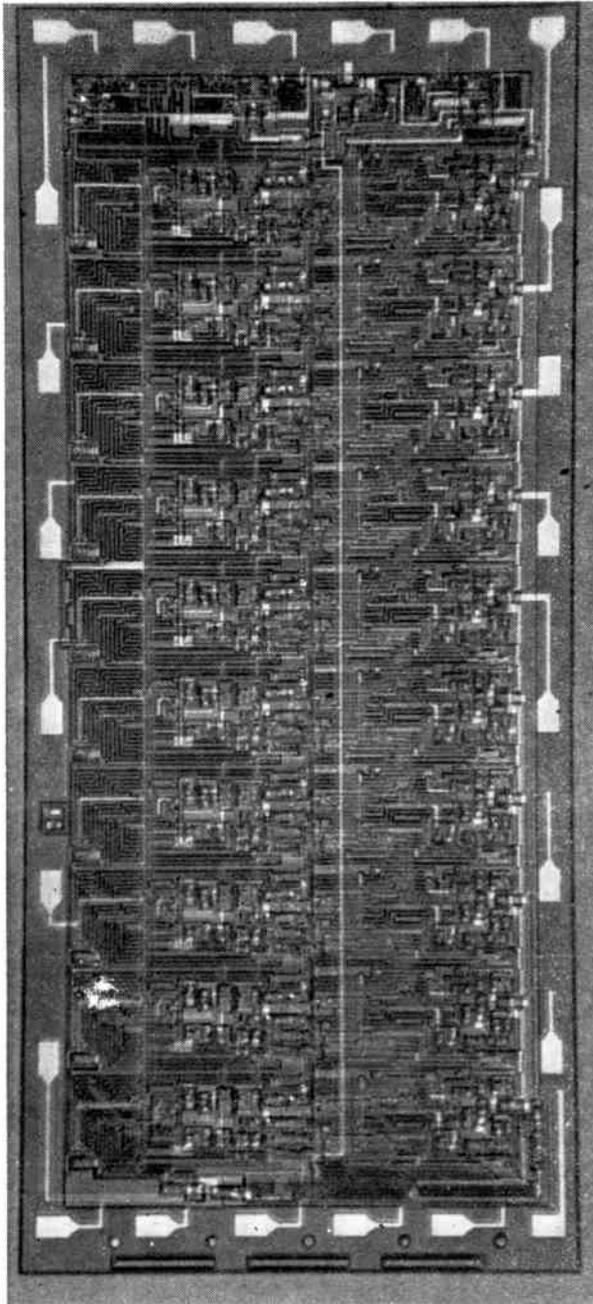
**FIGURE 2.** This monolithic subsystem can be used as a ten-stage counter or shift register. About 65 percent of the chip area is taken up by passive resistors.
