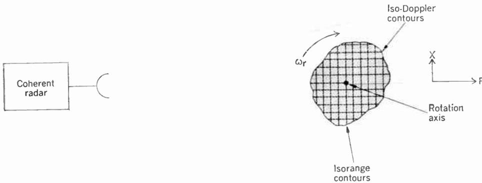
**FIGURE 5. Using a range-Doppler technique, it is possible to get a two-dimensional image of the radar reflectivity from a rotating body.**
