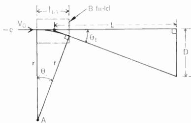
FIGURE 2. The force acting on an electron moving in a magnetic field is perpendicular to both its direction of motion and the direction of the magnetic field. In the diagram, L is the perpendicular distance from the center of deflection to the flat faceplate of the CRT, D is the deflection distance, and  $\theta$  is the deflection angle. Box text explains remaining symbols.
