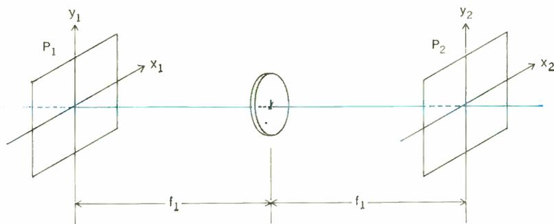
FIGURE 8. Light distributions at the front and back planes of the lens are related by a Fourier transform.
