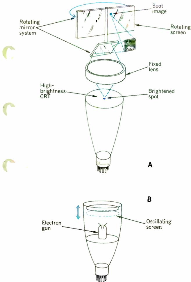
**FIGURE 3.** Autostereoscopic display system using a rotating screen (A),<sup>12</sup> and using an oscillating screen (B).<sup>15</sup>
