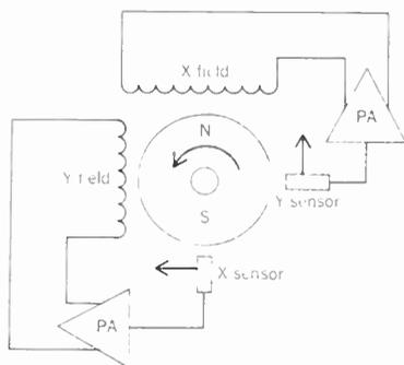
FIGURE 2. Two sensors used to detect rotating field of dc motor rotor.
