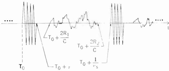
**FIGURE 12.** Delay relationships exist between outgoing and incoming side-looking radar pulses.  $R_1$  and  $R_2$  represent the nearest and farthest slant range probed.
