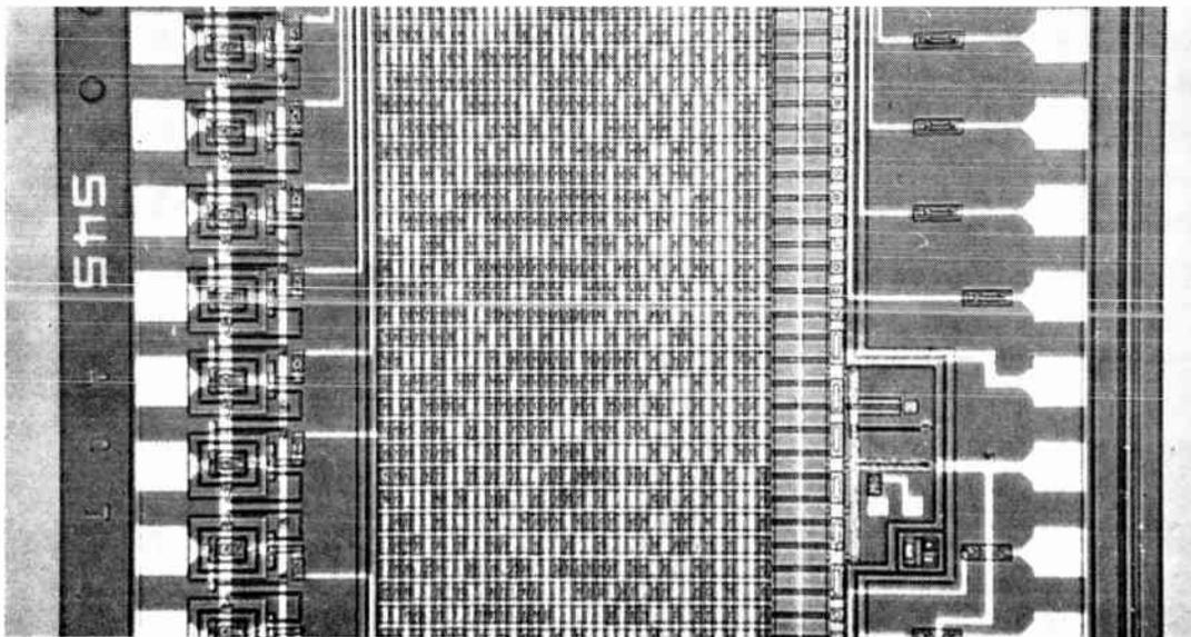
**FIGURE 1.** Portion of an LSI digital word translator that contains more than 12 650 active components per square centimeter. The integrated subsystem translates a 6-bit input word to 64 24-bit output words.
