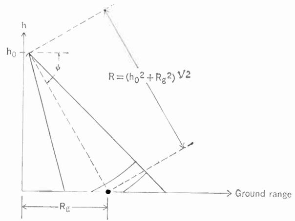
FIGURE 3. Behind side-looking radar resolution are pulsing and time-delay sorting.
