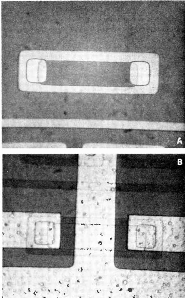
FIGURE 8. Typical n tunnel shown (A) before metalization and (B) after the metalization has been completed.
