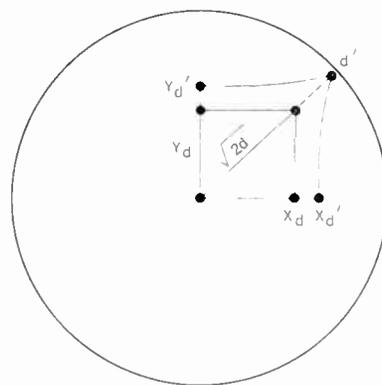
FIGURE 5. This is a schematic front-view of a flat-face CRT with variously deflected spot positions:  $Y_d$  is the desired or correct location of a vertically deflected spot;  $Y_d'$  is its actual position owing to a nonlinear sweep.  $X_d$  and  $X_d'$  are the horizontal counterparts of the Y's.
