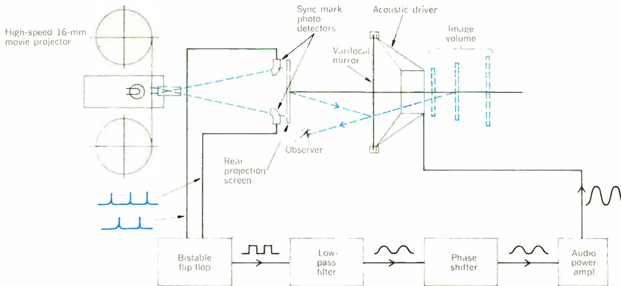
**FIGURE 6. Schematic diagram of a 3-D computer-generated movie projection system. Photodetectors are used to detect sync marks and generate the mirror driving voltage.**
