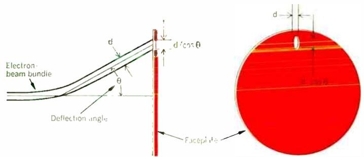
**FIGURE 11. Widening of the electron beam at focal plane is an astigmatic effect. One cause, shown here, is purely geometric.**
