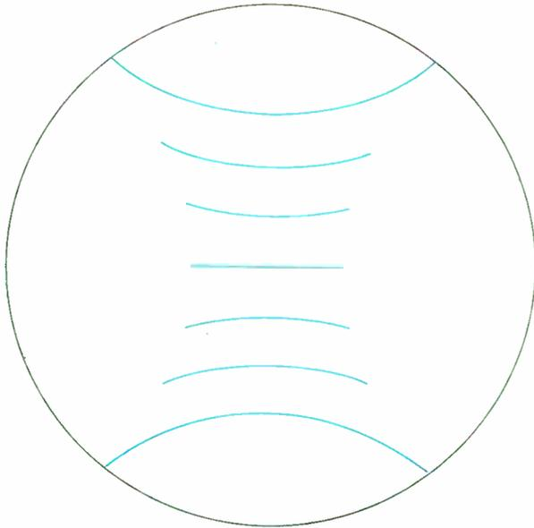
**FIGURE 1.** With pincushion distortion, straight lines take on more and more curvature toward the periphery of the cathode-ray tube.
