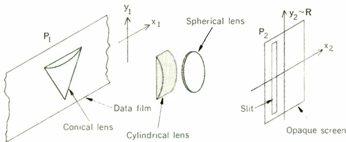
**FIGURE 15.** With this optical arrangement, a view through the vertical slit at  $P_2$  displays output of the synthetic aperture for all ranges with the same along-track dimension.
