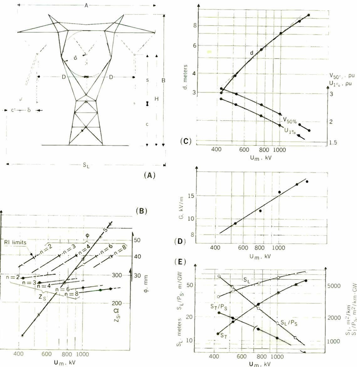
FIGURE 1. Basic characteristics of UHV lines of the traditional type vs. highest system voltage,  $U_m$ . (A) Tower geometry. (B) Conductor characteristics. (C) Insulation characteristics. (D) Voltage gradient  $G$  at ground. (E) Size parameters.
