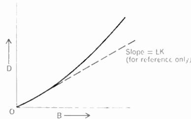
FIGURE 4. The deflection of electron beam across a flat faceplate of a CRT as a function of field strength becomes less linear as the field amplitude increases.
