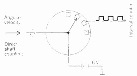
FIGURE 4. Angular velocity measurement.
