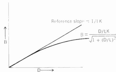
FIGURE 6. The magnetic field may be compensated to provide linearity over the entire CRT faceplate.
