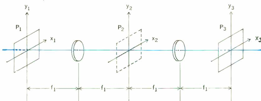
FIGURE 9. A succession of two transformations, achieved with this double lens arrangement, reverses the coordinates of the original amplitude distribution.
