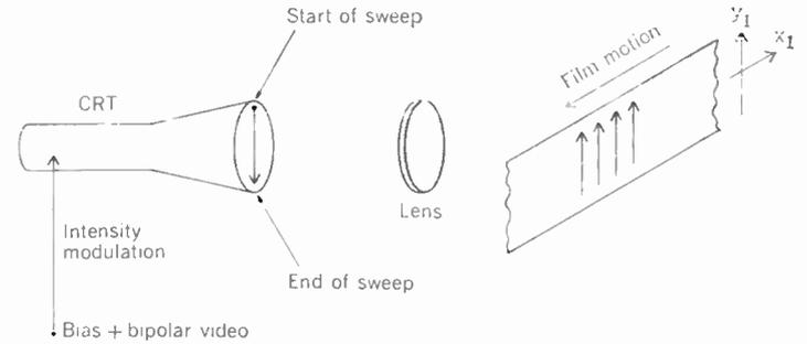
**FIGURE 13.** Radar signals are sent through a biased CRT, and then recorded on film for subsequent optical processing.
