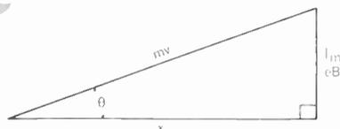
FIGURE 3. The trigonometric relations created by electron deflection in a magnetic field are better visualized in this section expanded from Fig. 2.
