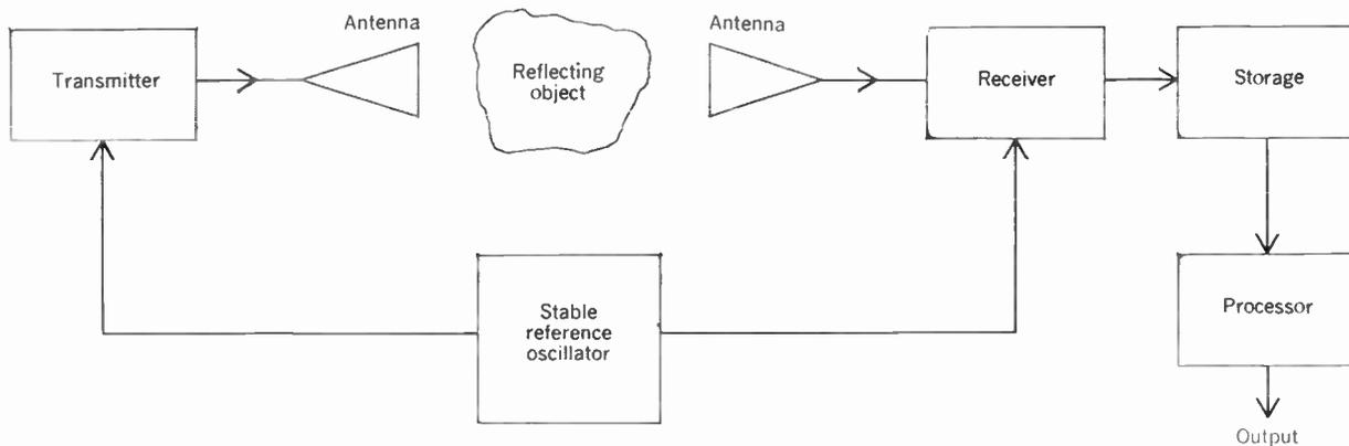
**FIGURE 7.** These pieces collectively constitute a synthetic-aperture radar.
