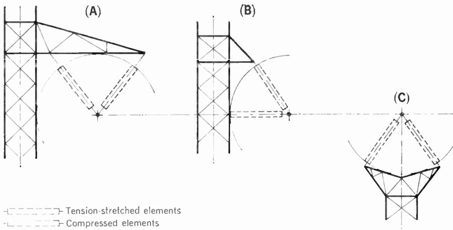
**FIGURE 5.** Bidimensional insulating structures. (A) V string. (B) Insulating cross-arm. (C) Reverse V cross-arm.
