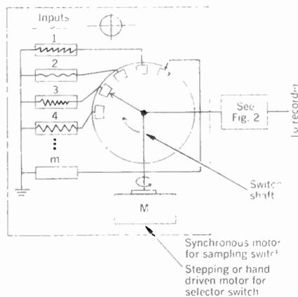
FIGURE 1. Sampling/selector switch.
