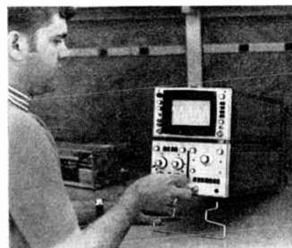
thereby increasing the photographed writing speed (to about 4 cm/ns). It also "fogs" photographic film slightly to increase effective film sensitivity. To simplify single-transient photography, the flood gun can be flashed in synchronism with the horizontal sweep, allowing the camera shutter to be left open for the event. The flood gun turns on only with the sweep.
