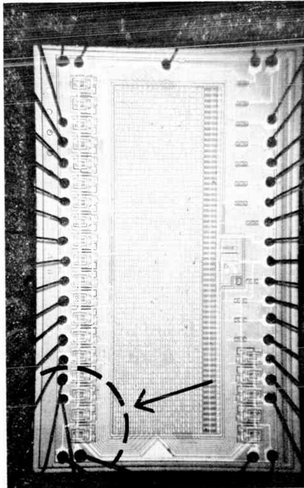
FIGURE 10. Wired digital word translator. The arrow indicates crossing wires caused by bad pad placement.
