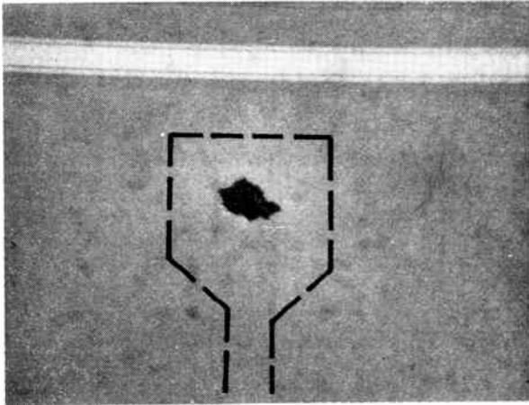
FIGURE 11. Breakdown of oxide due to ultrasonic bonding.
