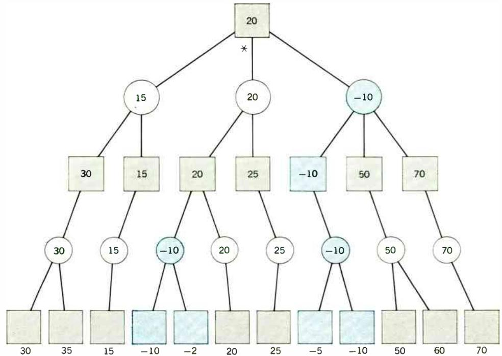
**FIGURE 2.** A computer's life may be just a game of checkers. Here is a simplified model of a segment of a computer program designed to make the computer victorious over its human opponent. The computer's alternatives are indicated by boxes and the man's by circles. Enclosed numbers are subscores. The computer looks ahead and chooses the best route for the highest ultimate score—assuming that its opponent also knows the tree of scores.
