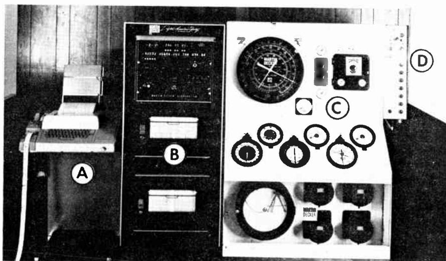
**COMPONENTS OF THE SYSTEM.** A — Teletype with punched tape. B — Digital acquisition reporting technique console with digital logic and presentation component (top) and analog recorders (bottom). C — Driller's instrument panel with complete instrumentation. D — Driller's selection panel for retrieving drilling functions.
