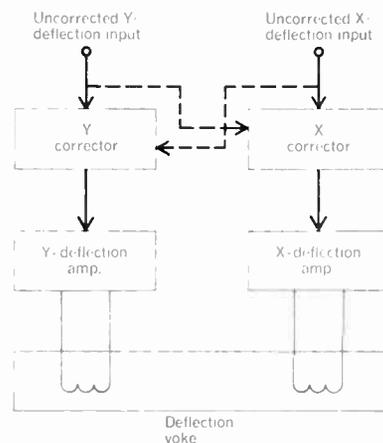
FIGURE 7. Because correction for the X and Y magnetic deflection fields are interrelated, coupling is needed between the two—indicated by the dashed cross-coupling lines.
