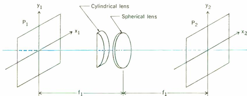
FIGURE 10. Information from each of the coordinates can be processed differently. Here,  $A_2$  is a Fourier transform of  $A_1$  in the  $x$ -direction and simply inverted in the  $y$ -direction.
