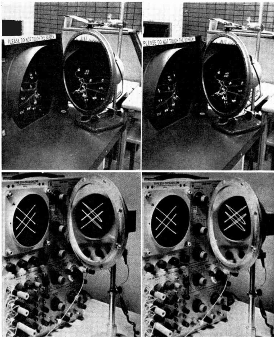
**FIGURE 5.** Stereo pairs (top) showing varifocal mirror displays of Traub's computer simulation of a 3-D radar display, and (bottom) a 3-D Lissajous figure. The stereo pairs can be viewed by hand holding a pair of lenses (of 10- to 30-cm focal lengths) in front of each eye.
