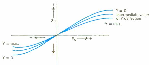
**FIGURE 8.** A family of curves is shown for the corrected magnetic deflection field  $B$  in the  $X$  direction as a function of the distance  $X$  for values of  $Y$  deflection.
