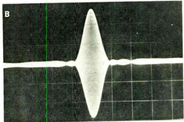
**FIGURE 12.** Advanced form of FM pulse-compression filter in which weighting of tap coupling is employed. (Courtesy R. Tancrell and M. G. Holland, Raytheon Research Division, Waltham, Mass.)
