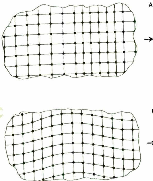
**FIGURE 2.** A—Pattern showing how a uniform square mesh in a material is displaced from its equilibrium configuration in the presence of a longitudinal wave. B—Similar pattern for a shear wave (transverse wave).
