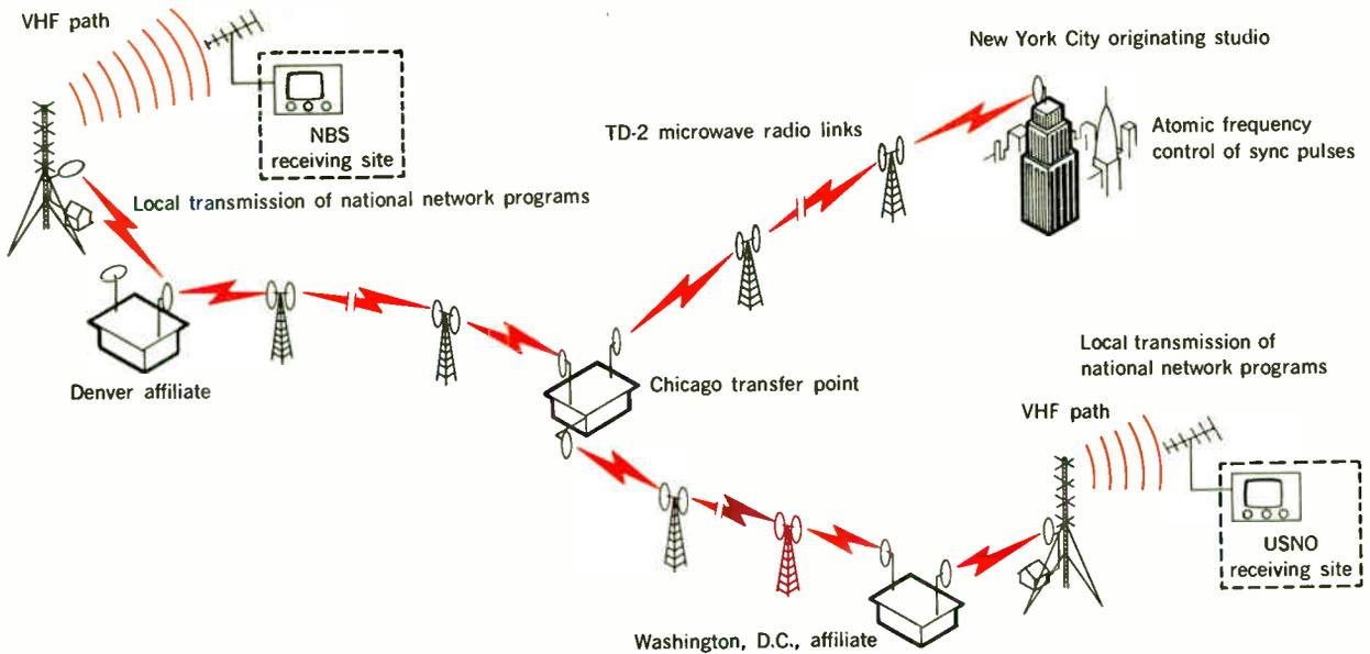
**FIGURE 3. Typical routing of television signals from New York City to distant receivers. Microwave path from New York to Denver  $\approx$  4000–6400 km (depending on network). VHF path from Denver transmitter to NBS  $\approx$  30 km.**
