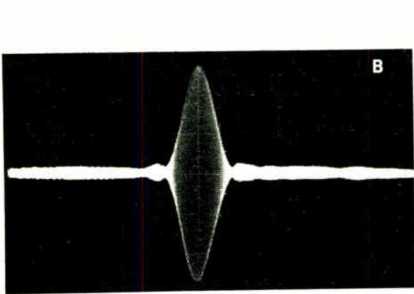
**FIGURE 10.** Surface-wave FM pulse-compression filter with the tap coupling weighted according to a cosine-squared law to reduce sidelobes in the compressed pulse. Scale is in centimeters.<sup>15</sup>
