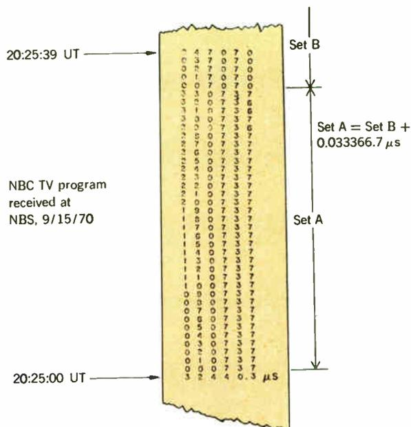
FIGURE 8. Sample printout of TV line-10 (NBS) counter readings in terms of clock 8.
