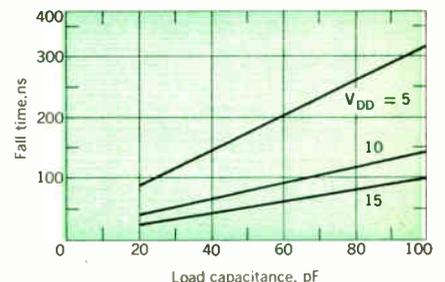
FIGURE 5. Typical fall times.
