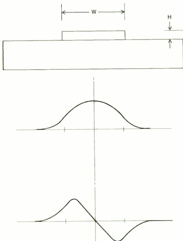
other type, in which the layer is less stiff and more dense than the substrate, the phase velocity *decreases* with increasing propagation constant. Such a layer is said to "load" the substrate. An example is gold on LiNbO<sub>3</sub>. Love waves do not exist in stiffened substrates, but an unlayered substrate will support a type of Love wave if the substrate is piezoelectric or magnetostrictive.<sup>20-22</sup>
