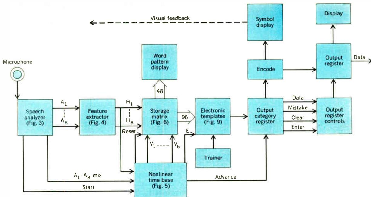
FIGURE 10. Automatic word recognizer.
