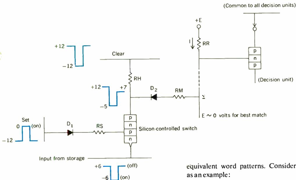
FIGURE 8. Electronic template unit.
