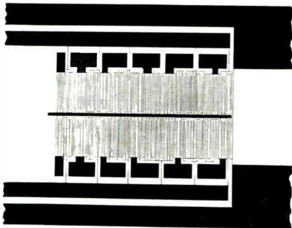
**FIGURE 13.** Input transducer for delay line using Golay-coded complementary sequences. Upper half of transducer generates Golay-coded waveform; lower half generates complement. Output transducer is identical.
