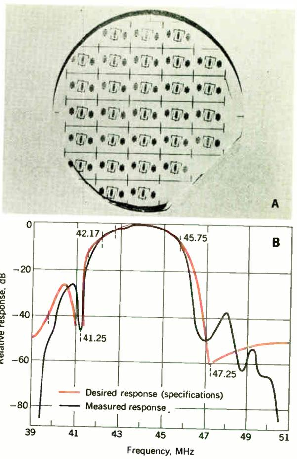
**FIGURE 8. A—Photograph of several surface-wave filters for color television IF circuit on a PZT substrate. B—Response curves. (Courtesy A. de Vries, Zenith Microcircuit Facility, Elk Grove, Ill.)**
