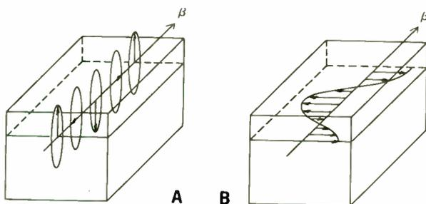
**FIGURE 14.** Polarization of the elastic displacement for the two major classes of surface waves in layered substrates. A—Generalized Rayleigh waves, elliptically polarized. B—Love waves, transversely polarized.
