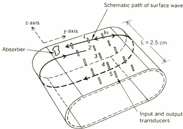
**FIGURE 25.** Method used to obtain long time delays by passing a wave several times around a piece of  $\text{LiNbO}_3$  with rounded ends. Transducer labeled "1n" is input and those labeled 2-5 are used as outputs.<sup>32</sup>
