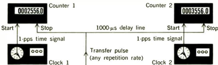
Case 1 (Lab): Counter 2 – Counter 1 = 3556.0  $\mu$ s – 2556.0  $\mu$ s = 1000  $\mu$ s
