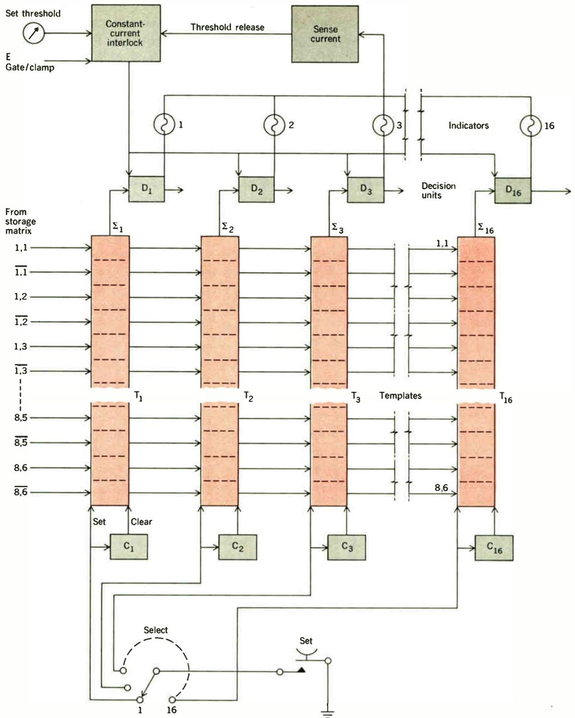
FIGURE 9. Adaptive electronic templates.
