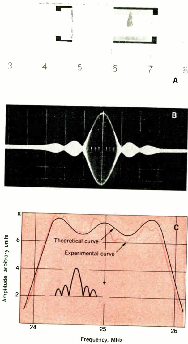
**FIGURE 7. A—Bandpass filter with a broadband transducer on the left.<sup>14</sup> Transducer on right has an active filter length that varies as  $(\sin kx)/x$  with distance. Scale is in centimeters. B—Impulse response of the bandpass filter (amplitude vs. time with a  $\delta$ -function input). C—Frequency response of the bandpass filter.**
