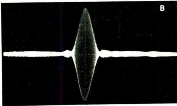
**FIGURE 10.** Surface-wave FM pulse-compression filter with the tap coupling weighted according to a cosine-squared law to reduce sidelobes in the compressed pulse. Scale is in centimeters.<sup>15</sup>
