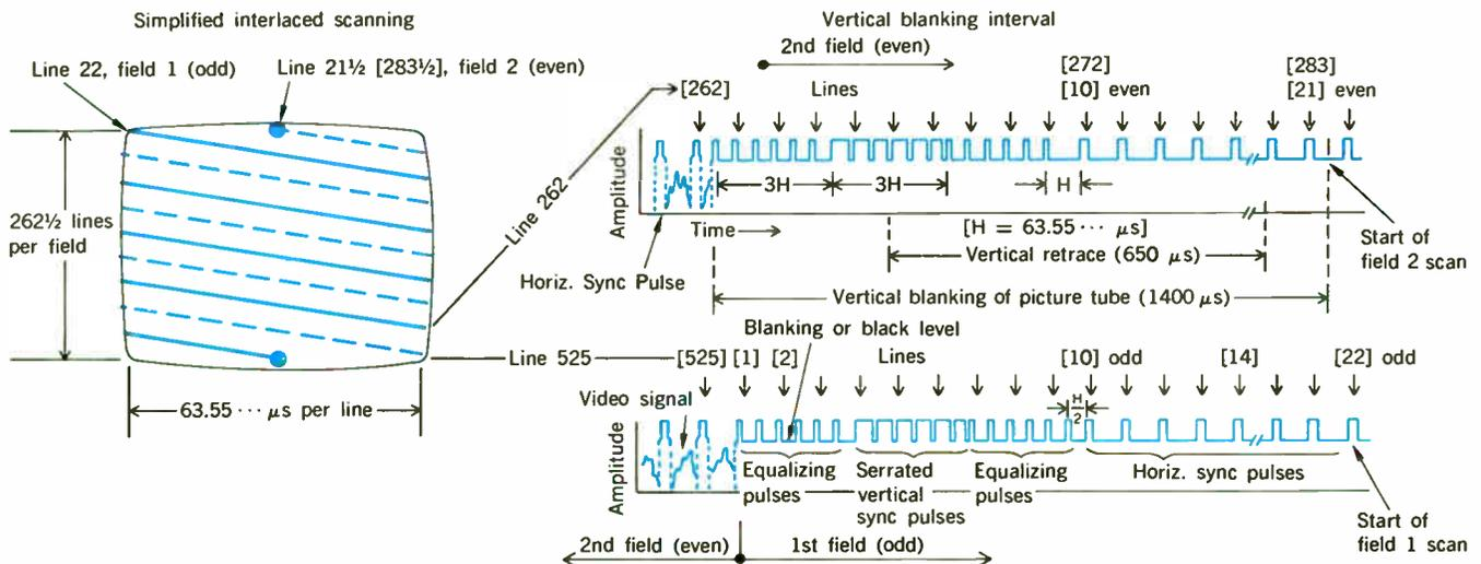
field and, as indicated in Fig. 6, this can be easily accomplished through the time relationship of line 10 to the equalizing pulses of the successive fields.
