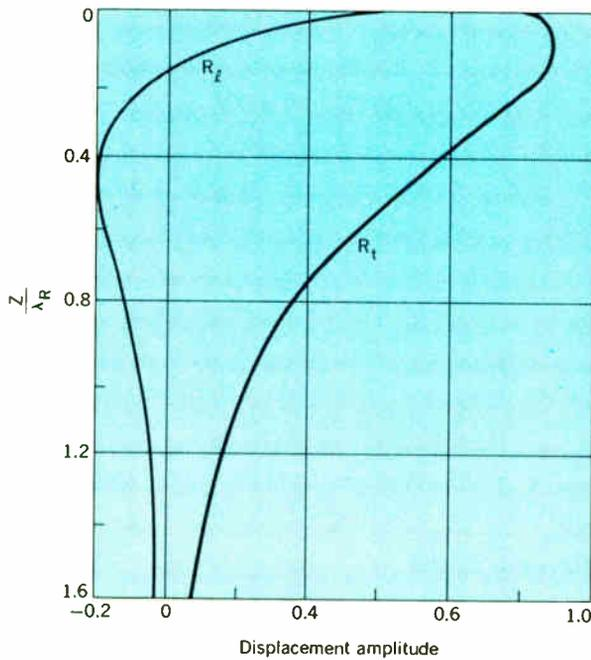
**FIGURE 4.** Variation of elastic displacement amplitudes as a function of depth for a Rayleigh wave in isotropic material;  $\lambda_R$  denotes the propagating wavelength.
