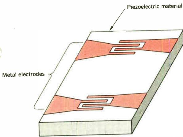
**FIGURE 1.** Schematic representation of a typical piezoelectric surface-wave device with interdigital electrodes.
