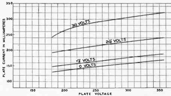
Fig. 8—Plate-Current, Plate-Voltage Characteristics of CX-322.
