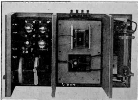
Fig. 6—Standard Oscillator with Cover Removed.
