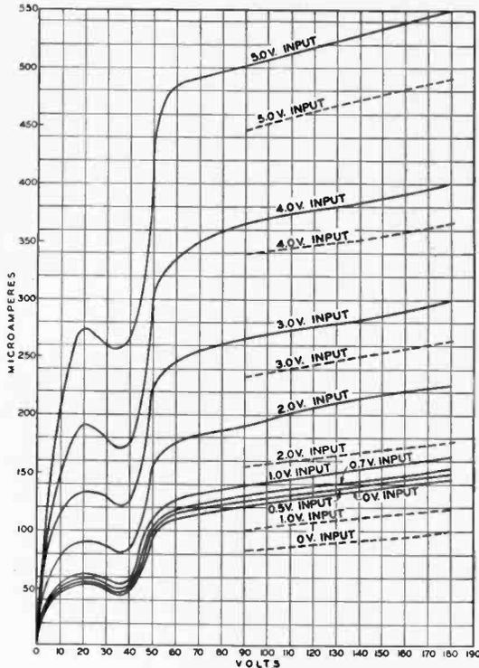
Fig. 6—Plate Current—Plate Voltage Characteristics of CX-322.
