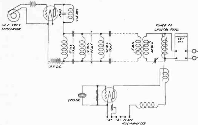
Fig. 10—Crystal Calibrating Circuit.
