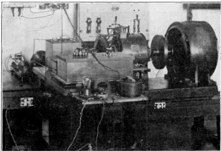
Fig. 7—Apparatus Used in Calibrating Crystal. Motor-Generator at Right, Maxwell Bridge Units in Center, Chronograph Drum at Left Rear.
