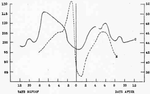
Fig. 4—Comparison of Newton Reception and Boston Temperature Changes.
