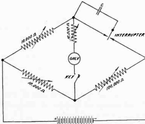
Fig. 9—Maxwell Bridge Circuit.
