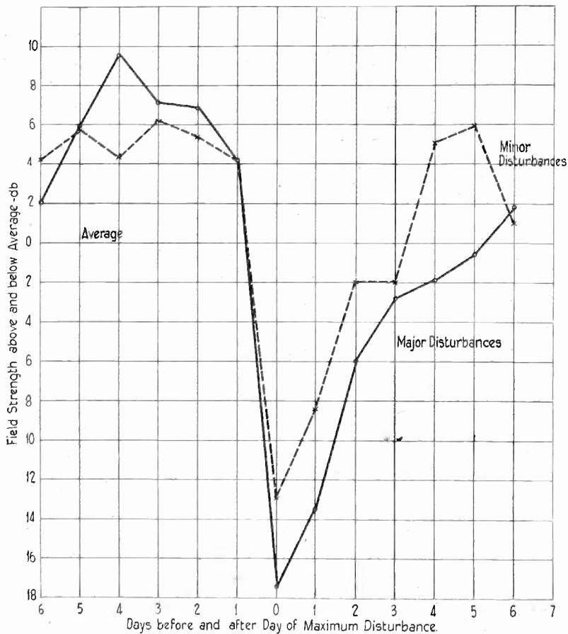
Fig. 15—Average behavior of 18-megacycle field strengths between New York and London during major and minor disturbances of earth potential.
