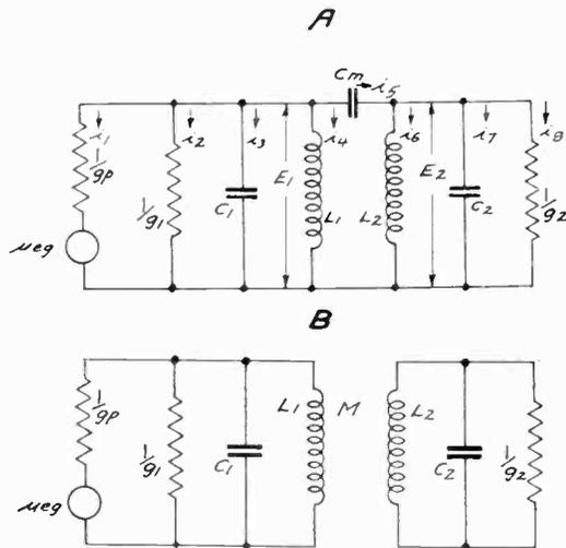
Fig. 2—Coupled circuits.
