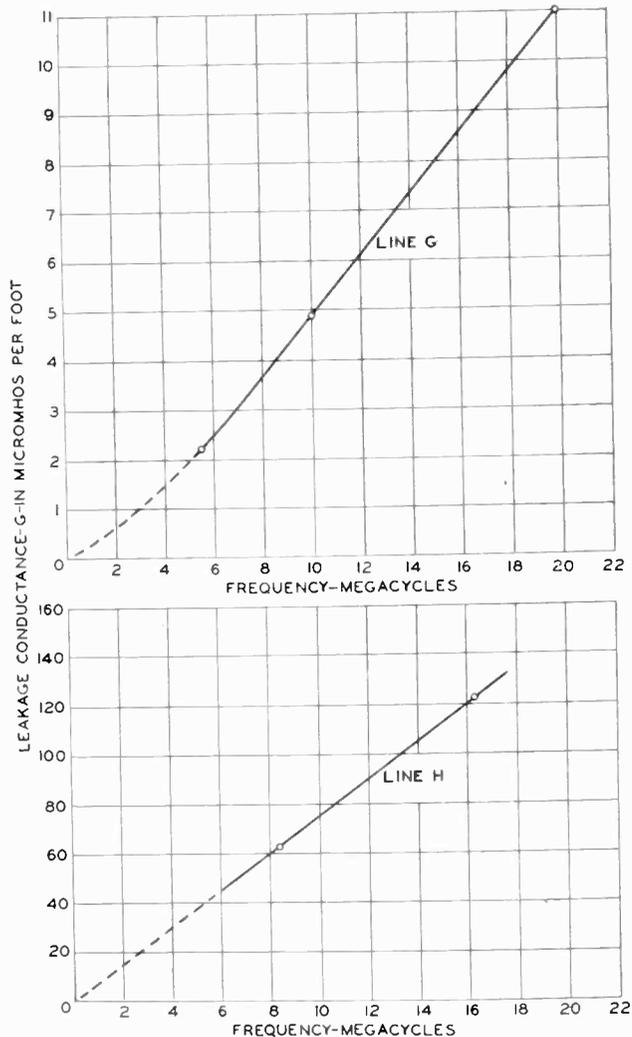
Fig. 3—Derived leakage conductance for the concentric tube lines *G* and *H* of Fig. 1. Line *G* was completely filled with porcelain insulators. Line *H* comprised a No. 18 B and S conductor with rubber insulation and lead sheath.
