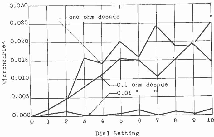
Fig. 10—Change of inductance with dial setting for six-dial shielded box.
