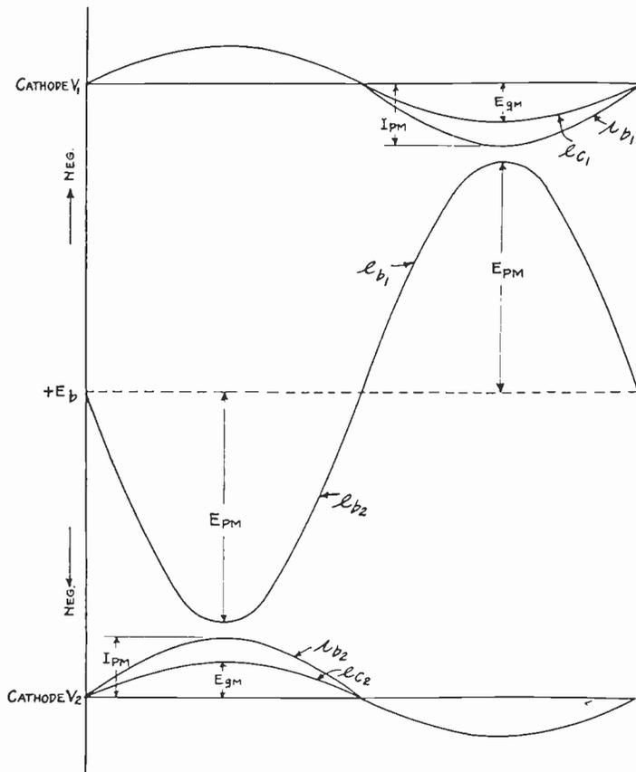
Fig. 5—Diagram of instantaneous voltages and currents for a class B audio amplifier.
