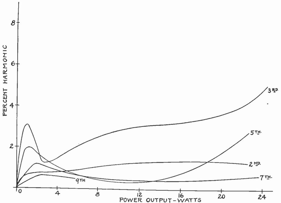
Fig. 6—Distortion curves for an a-c operated amplifier using two RCA-46 tubes and designed for approximately maximum output.
