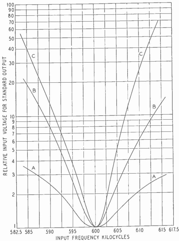
Fig. 6—Measured selectivity curves. Fig. 5 circuits in tune.
