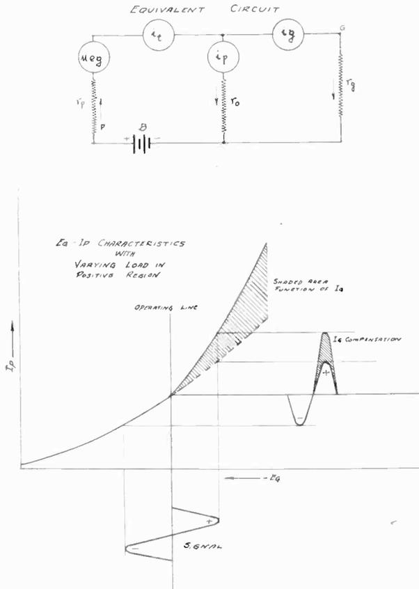
Fig. 2—Equivalent circuit and action of grid current compensation.
