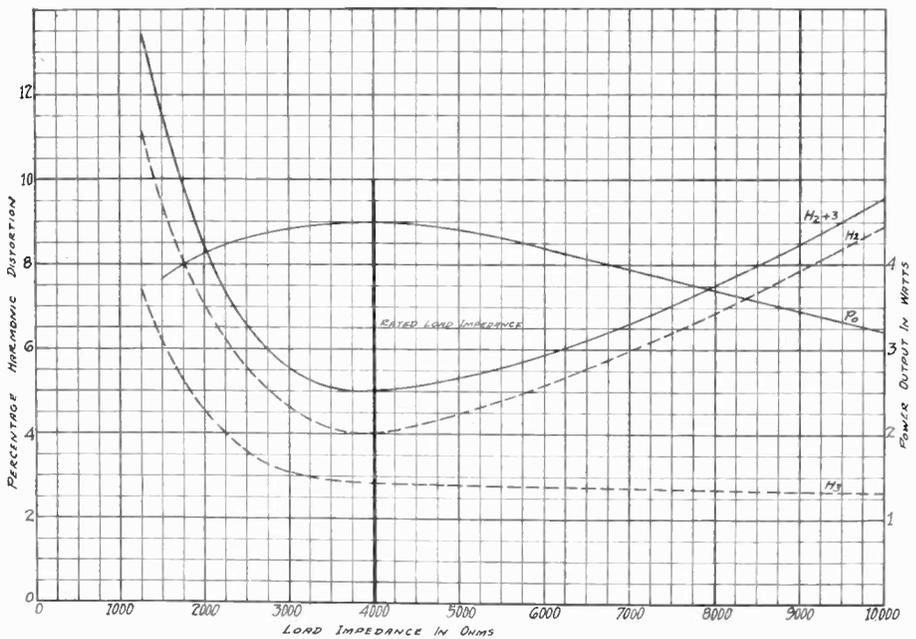
Fig. 7—Curve showing maximum power output occurring at the same load as minimum distortion  $\left(\frac{E_h}{E_f} \times 100\right)$ . Notice predominance of second harmonic. Speed 295.
