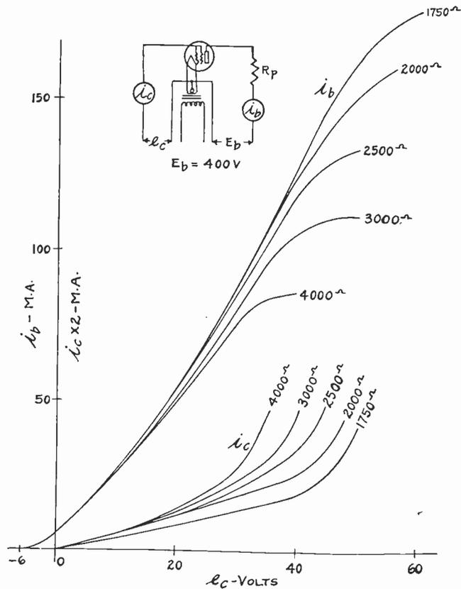
Fig. 1—Load characteristics of an RCA-46 for class B operation.
