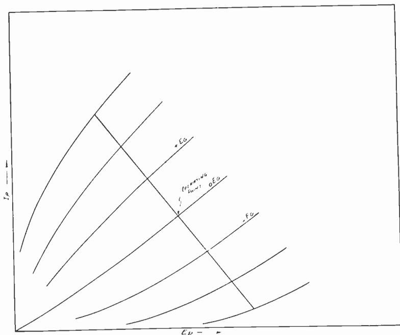
Fig. 6—Explanatory output plate characteristics. Illustrates "fanning" in both positive and negative regions of the output plate characteristics.
