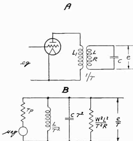
Fig. 1—Single tuned circuit.
