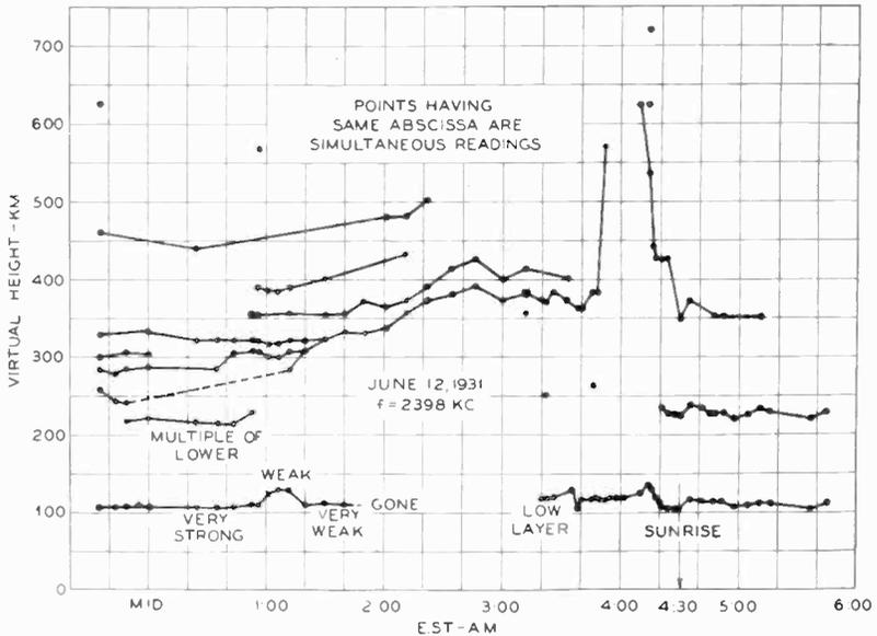
Fig. 3—Virtual-height variations during the early morning of June 12, 1931, for a frequency of 2398 kc. Note the varying intensity of the amplitudes of reflections from the lower layer and the fact that the virtual-height variations are not very great. The virtual-height variations of the upper layer are much greater during the same period. Split peaks are shown for the upper layer as well as a critical period shortly before sunrise.
