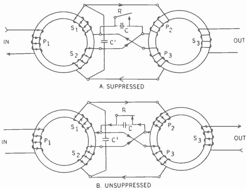
Fig. 3—Repeating coil arrangement for suppressing echoes.
