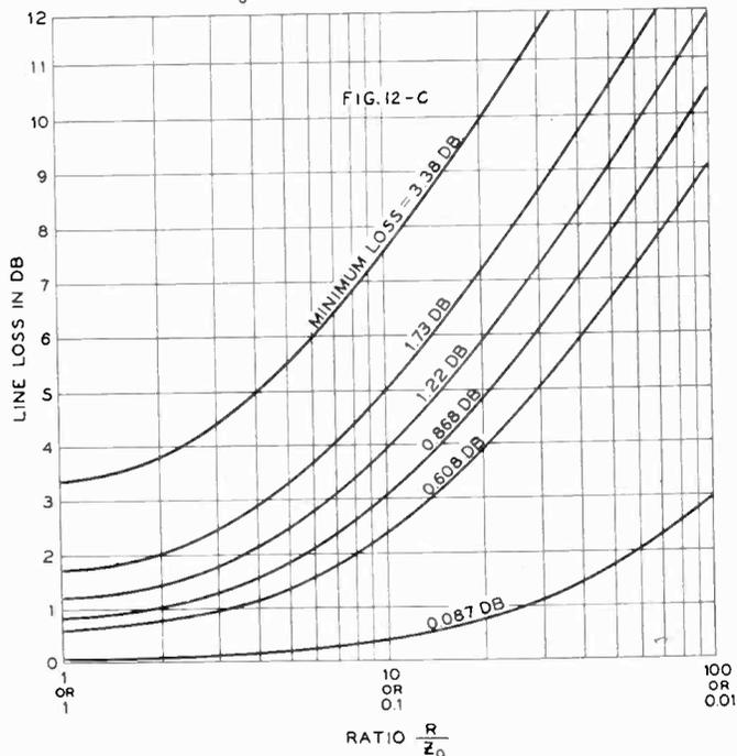
Fig. 12—Line loss as a function of the degree of matching. The several curves are designated in terms of the minimum line loss obtained for the case of a perfect match with the line characteristic impedance.
