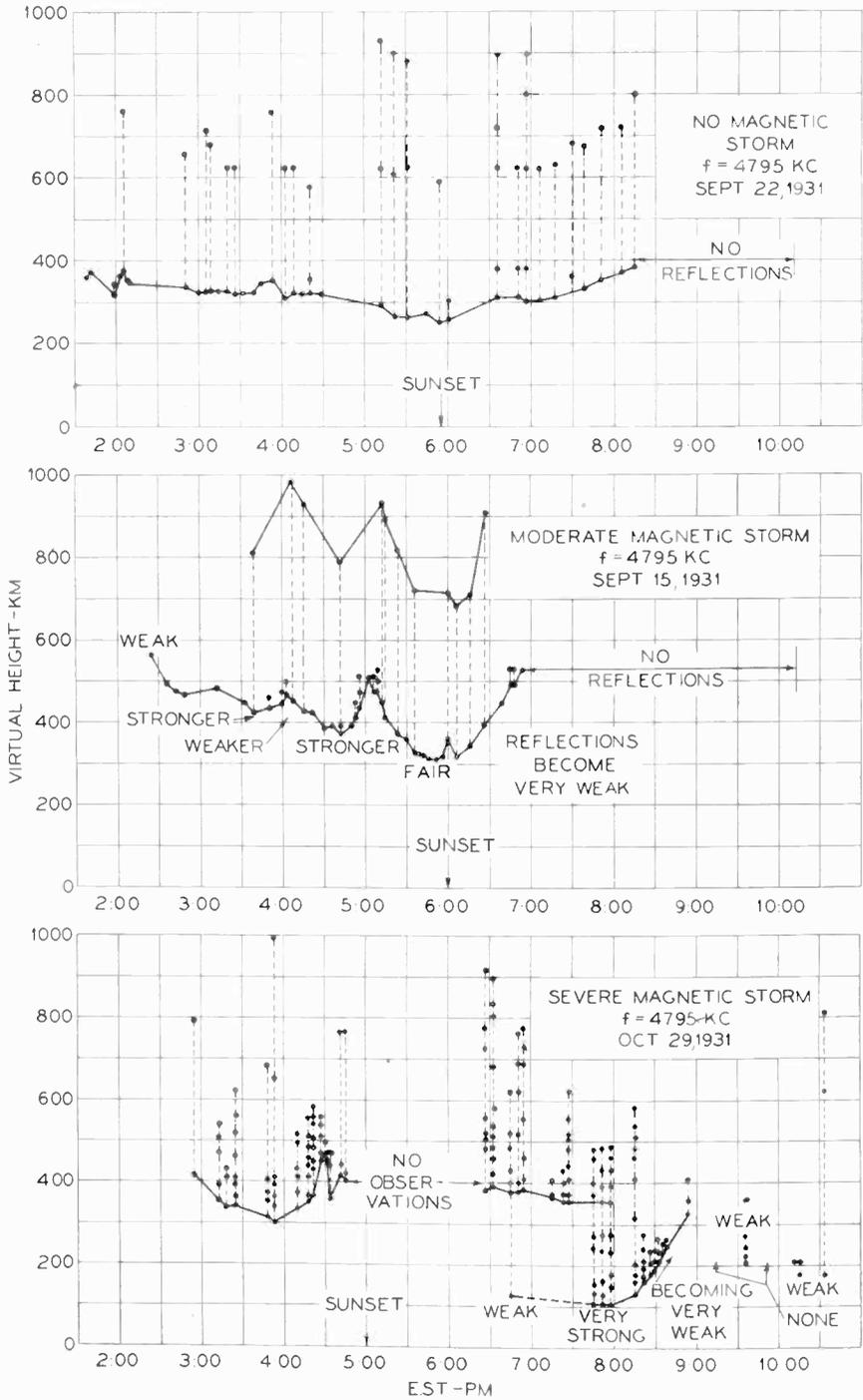
Fig. 5—Virtual-height variations for three days during which the magnetic conditions were different. Note that the virtual heights become much more irregular as the magnetic disturbance increases.
