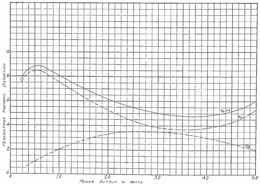
Fig. 5—Typical triple-twin harmonic distortion  $\left( \frac{E_h}{E_f} \times 100 \right)$  versus power output characteristic. Notice predominance of second harmonic. Speed 295.
