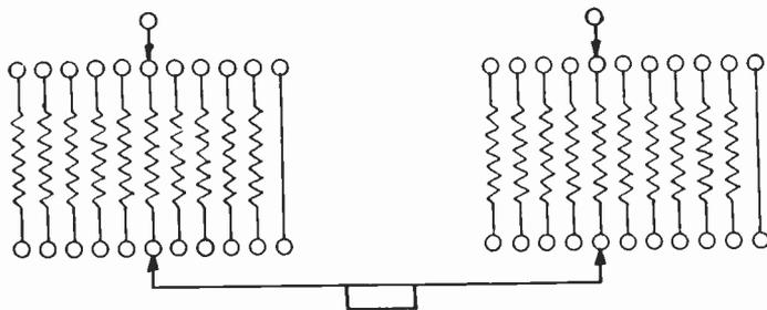
Fig. 7—Decade construction six-dial shielded box.
