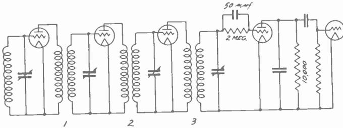
Fig. 5—Amplifier network used in obtaining experimental curves.
