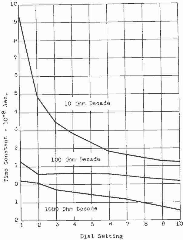
Fig. 9—Direct resistance characteristics of six-dial shielded box.
