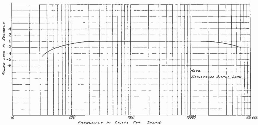
Fig. 8—Triple-twin fidelity curve. Speed 295.
