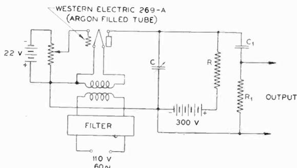
Fig. 1—Circuit of the pulse generator. The pulse generator is a relaxation oscillator in which the number of pulses generated per second is controlled by the time constant  $CR$ , while the duration of the pulses is controlled by the time constant  $C_1R_1$ . The control-frequency voltage is obtained by heating the filament of the tube with 60-cycle alternating current.
