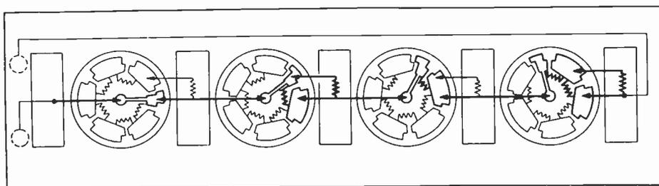
Fig. 2—Four-dial resistance box. Box set for 123. ohms 1000-, 100-, 10-, and 1-ohm decades. 1000-ohm decade at left.
