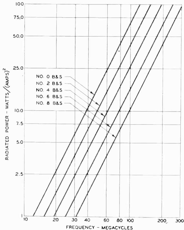
Fig. 9—Calculated power radiated by 600-ohm lines terminated in the characteristic impedance for several common conductor sizes. The line length is a factor of negligible importance for the above spacings and most practical lengths of line.
