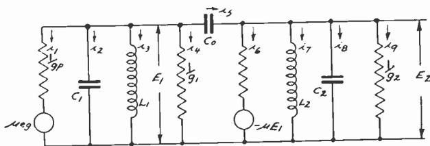
Fig. 3—Two-stage amplifier network, input not tuned.
