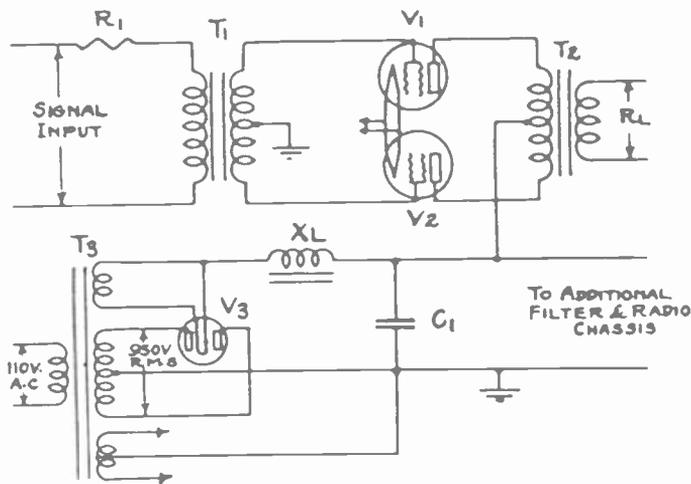
Fig. 4—Circuit for plate voltage supply and for class B audio amplifier.
