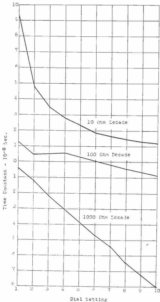
Fig. 8—Characteristics of six-dial shielded box. Shield connected to low terminal.
