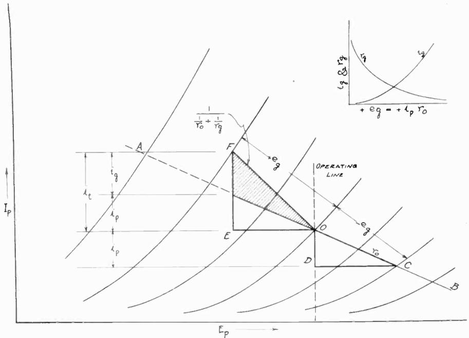
Fig. 3—Grid-current compensation theory. Plate characteristics of input section.
