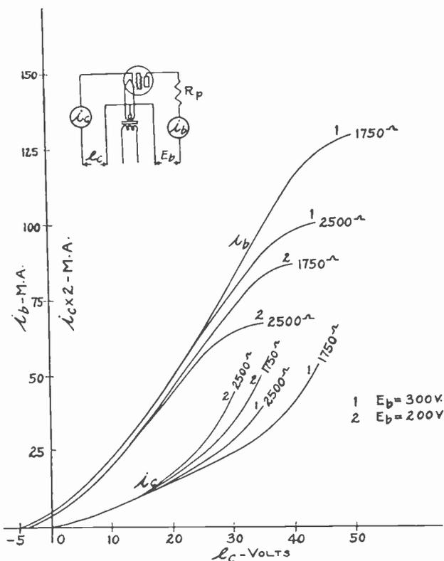
Fig. 2—Load characteristics of an RCA-46 for class B audio amplifier.
