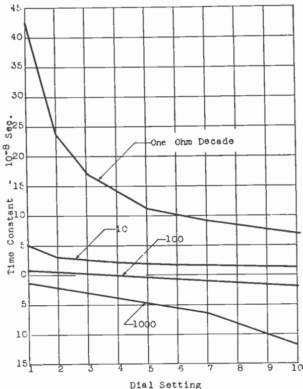
Fig. 4—Characteristics of four-dial shielded box. Shield connected to low terminal.
