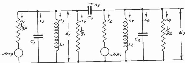
Fig. 3—Two-stage amplifier network, input not tuned.
