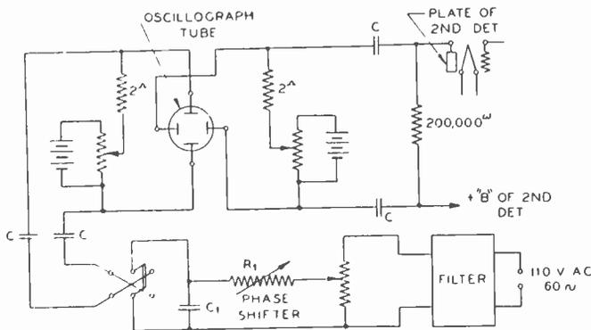
Fig. 2 Circuit of cathode ray oscillograph and output of radio receiver.
