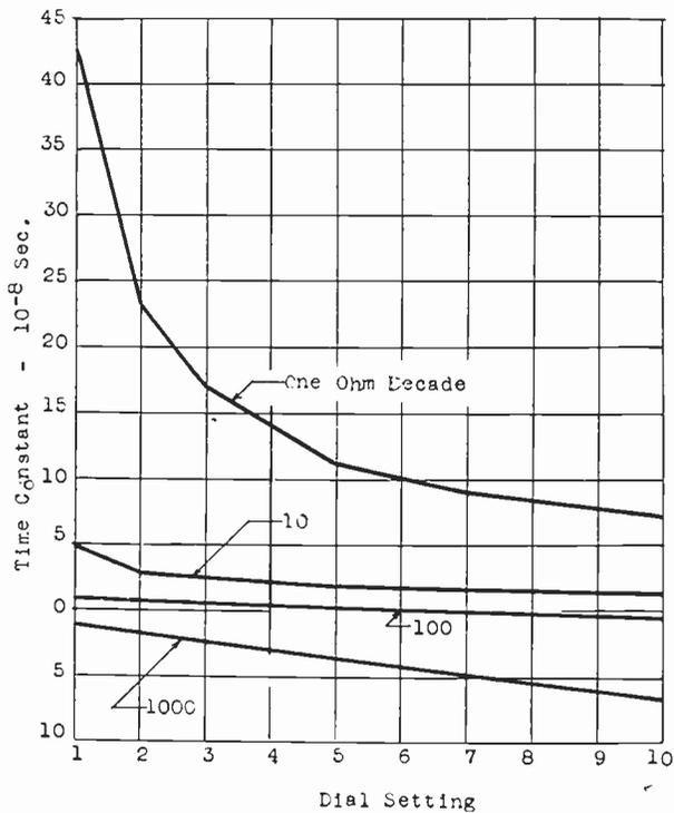
Fig. 3—Characteristics of four-dial unshielded box.
