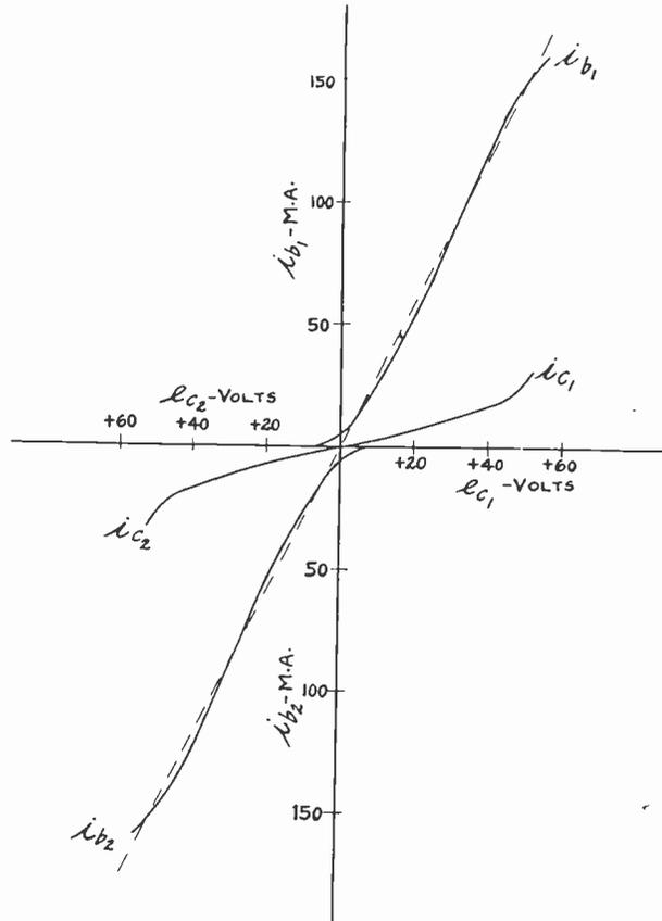
Fig. 3—Load characteristics of two RCA-46 tubes arranged for class B operation.
