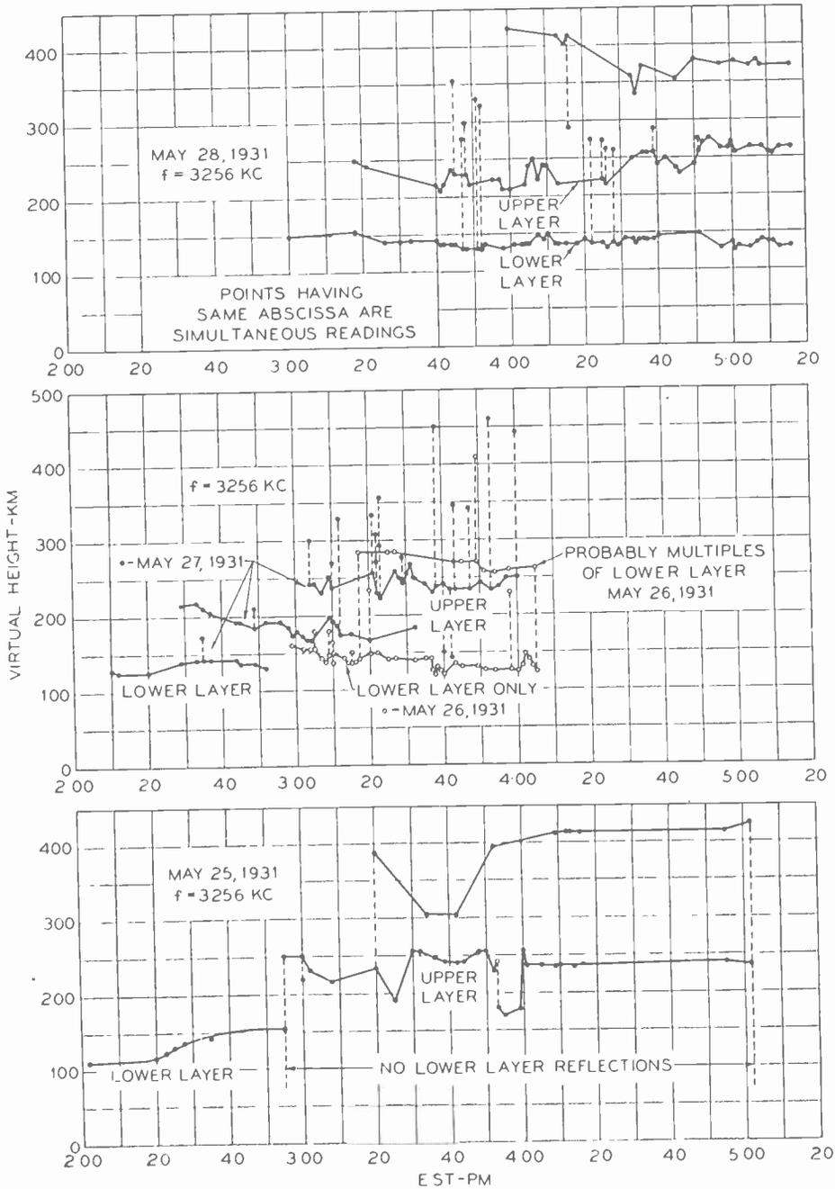
Fig. 4—Virtual-height variations during the afternoon for four successive days, May 25th to 28th, 1931, for a frequency of 3256 kc. Note the lack of duplication in the day-to-day virtual-height values.
