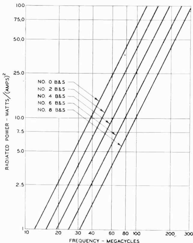
Fig. 9—Calculated power radiated by 600-ohm lines terminated in the characteristic impedance for several common conductor sizes. The line length is a factor of negligible importance for the above spacings and most practical lengths of line.
