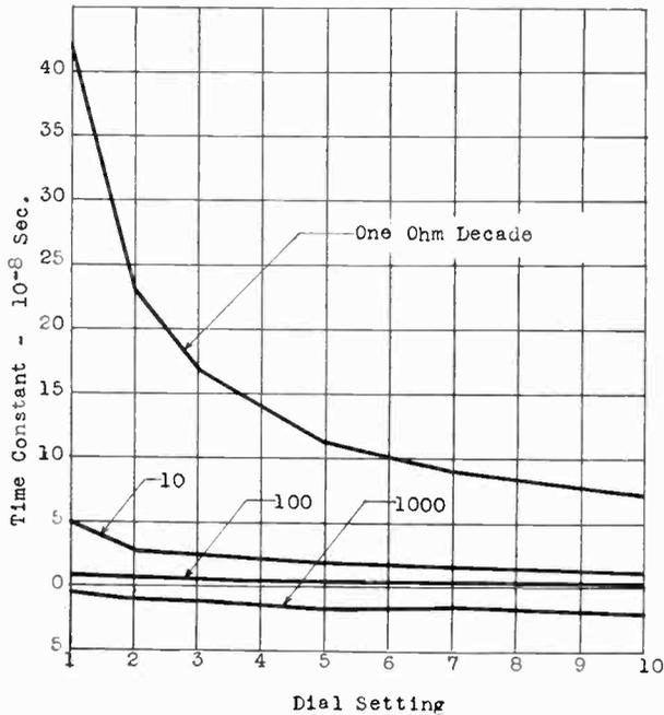
[Fig. 5—Direct resistance characteristics of four-dial shielded box.
