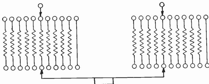
Fig. 7—Decade construction six-dial shielded box.
