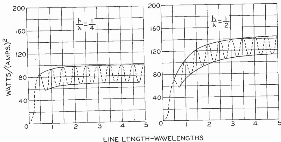
Fig. 10—Approximate power in watts radiated by an unbalanced current of 1.0 r-m-s amperes in a long two-wire line. Also, the power radiated by a single wire parallel to the earth for 1.0 r-m-s ampere line current. Two cases,  $\frac{1}{2}$  and  $\frac{1}{4}$  wavelength above ground are illustrated.
