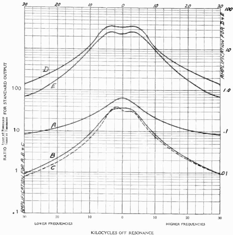
Fig. 4—Theoretical resonance curves.
