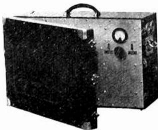
unit housing a rectifier and filter system. The system may be operated wherever 110 volt, 60 cycle lighting circuits are available, and the source of signal may be microphones, phonograph or radio set.
