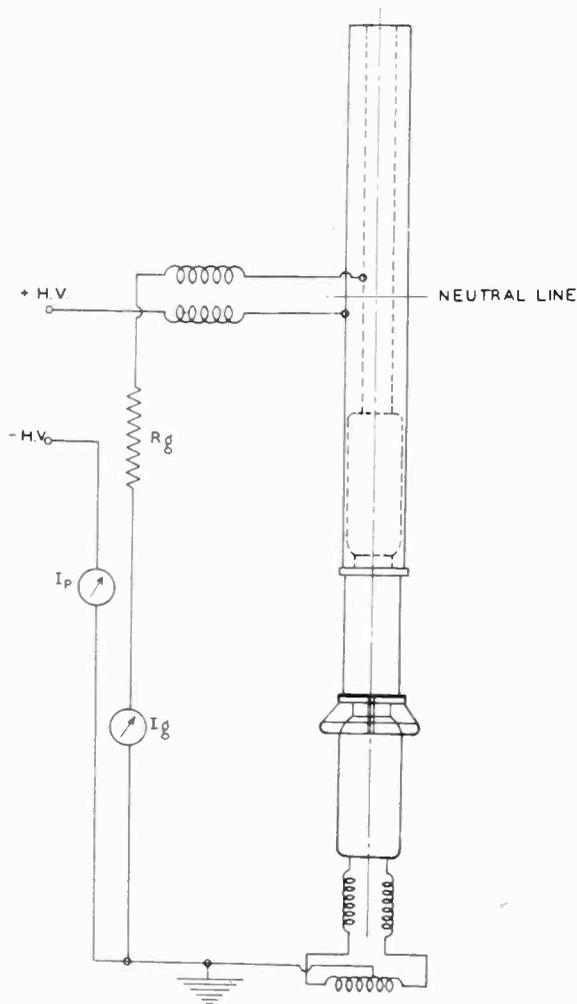
Fig. 7—Oscillating circuit using AW-200 tube.
