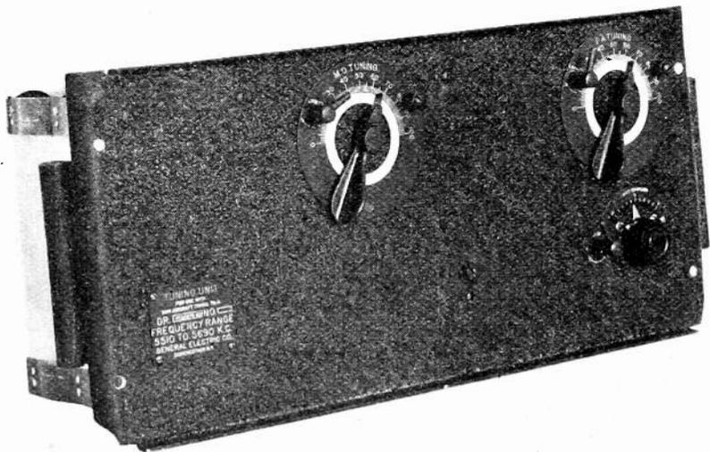
Fig. 6—Tuning unit for RT-76-A transmitter.
