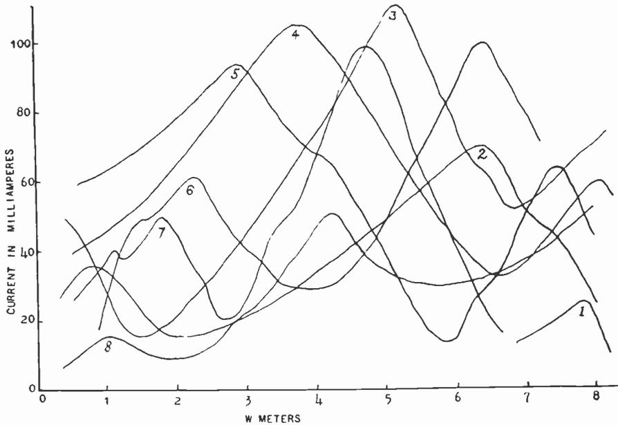
Fig. 10—Variation of received current with width ( $W$ ) of frame aerial.
