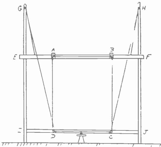
Fig. 7—Mechanical arrangement of adjustable frame aerial.
