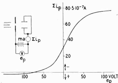
FIG. 12—Total plate current and plate bias.
