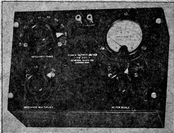
You have always measured audio power output with a resistor, voltmeter, and slide rule. Or perhaps you have discovered the convenience of the General Radio constant-impedance output meter introduced several years ago.
