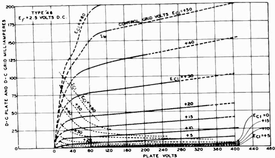
Fig. 12—Average plate characteristics. Class B operation.
