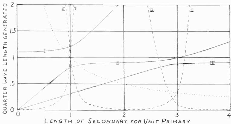
Fig. 4—Theoretical wavelength characteristics (solid lines), damping curves (dashed lines), and excitation curves (dotted lines), of the idealized coupled circuit oscillator with an open-end secondary. The curves are for  $k = 0.1$ . The ordinates for the damping and excitation curves are not given on the figure; they are the same for both sets of curves, and are equal to  $(N - r)/rs_2$  in which  $N$ , the negative resistance, is the variable parameter.
