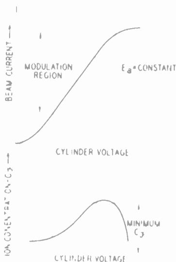
FIG. 5. Wehnelt cylinder luminosity control.
