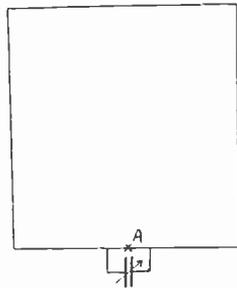
Fig. 8—Electrical circuit of adjustable frame aërial.
