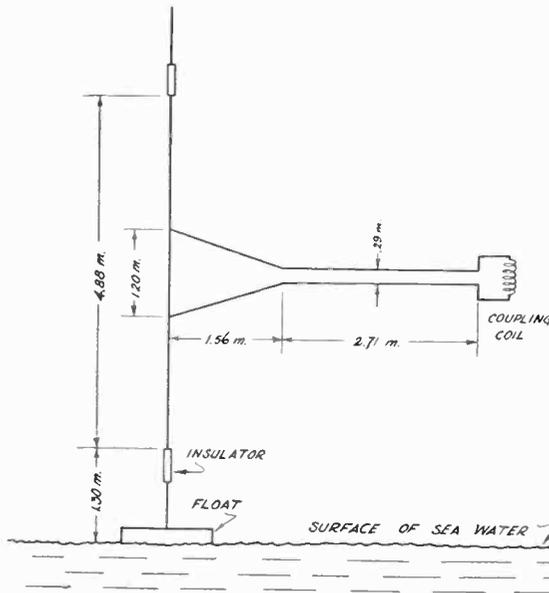
Fig. 1—Details of half-wave, vertical antenna used for the experimental work on 29 megacycles
