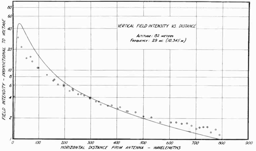
Fig. 4—Theoretical (Strutt) and experimental vertical field intensity vs. horizontal distance from the antenna for altitude of 82 meters.
