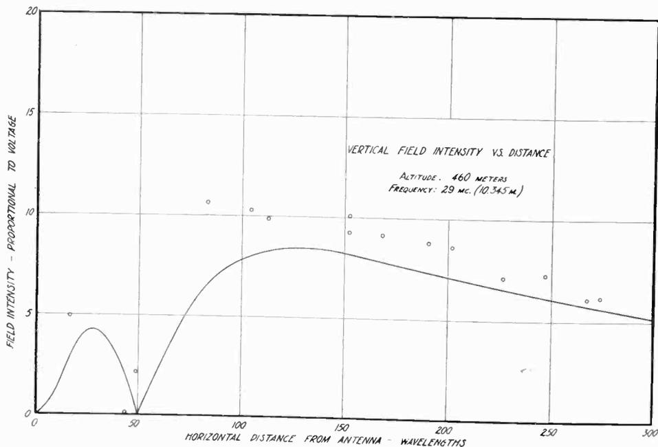
Fig. 14—Detailed theoretical (Strutt) and experimental vertical field intensity vs. horizontal distance from the antenna for altitude of 460 meters.
