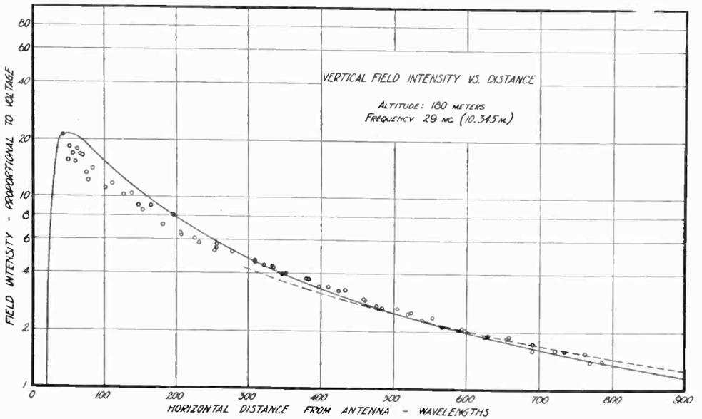
Fig. 5—Theoretical (solid curve: Strutt; dotted curve: Sommerfeld) and experimental vertical field intensity vs. horizontal distance from the antenna for altitude of 180 meters.
