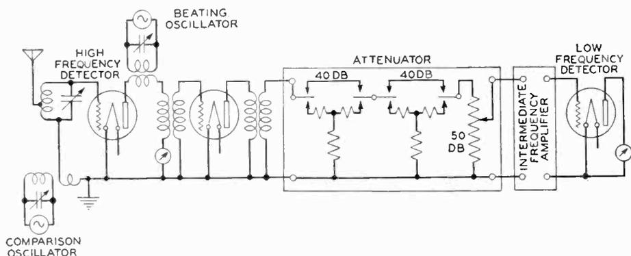
Fig. 1—Schematic diagram of field strength measuring set.
