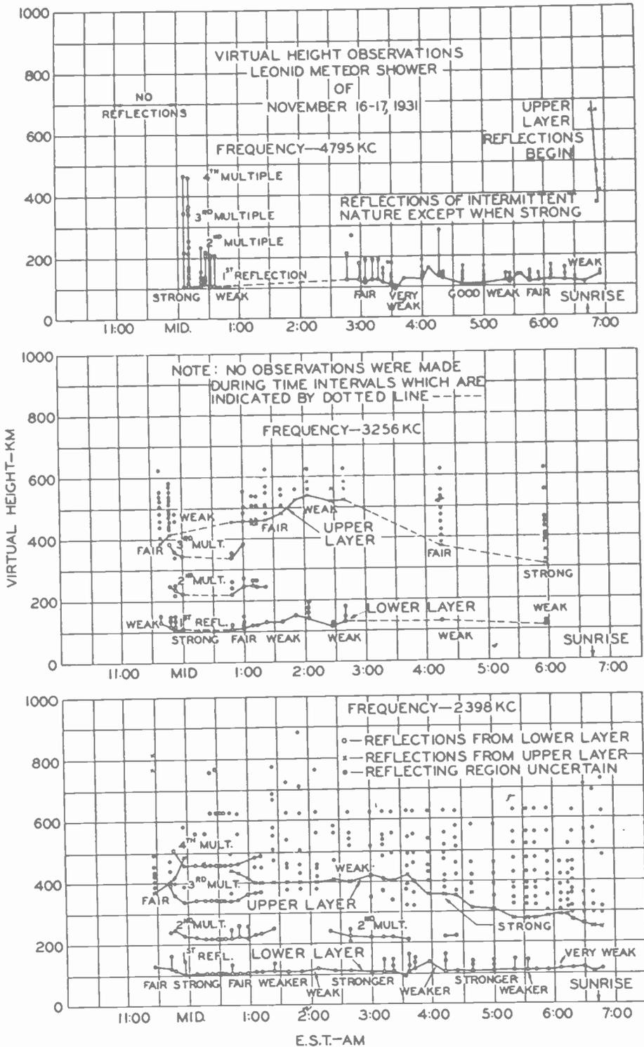
Fig. 1—Virtual height variations during the night of November 16-17, 1931, for frequencies of 2398, 3256, and 4795 kilocycles. Also note the variations in the intensity of reflections. From the behavior of the reflections from the lower layer it appears that there was a large increase in the effective ionization of the lower layer near midnight, and minor increases at about 2:45 and 4:30 A.M.
