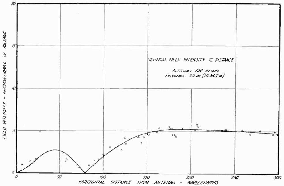
Fig. 17—Detailed theoretical (Strutt) and experimental vertical field intensity vs. horizontal distance from the antenna for altitude of 730 meters.
