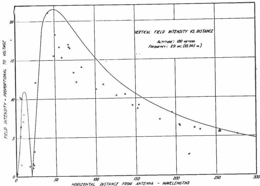
Fig. 12—Detailed theoretical (Strutt) and experimental vertical field intensity vs. horizontal distance from the antenna for altitude of 180 meters.
