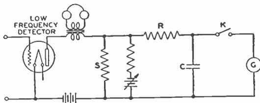
Fig. 4—Final recorder circuit.
