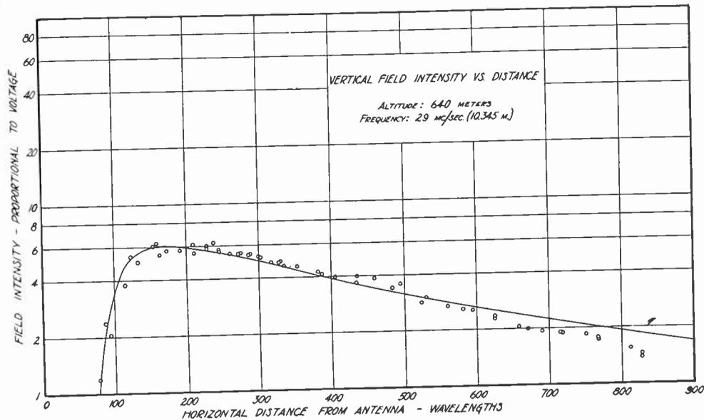
Fig. 10—Theoretical (Strutt) and experimental vertical field intensity vs. horizontal distance from the antenna for altitude of 640 meters.
