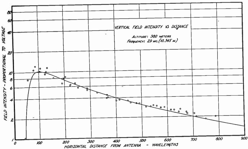
Fig. 7—Theoretical (Strutt) and experimental vertical field intensity vs. horizontal distance from the antenna for altitude of 380 meters.
