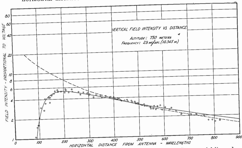
Fig. 11—Theoretical (solid curve: Strutt; dotted curve: Sommerfeld) and experimental vertical field intensity vs. horizontal distance from the antenna for altitude of 730 meters.
