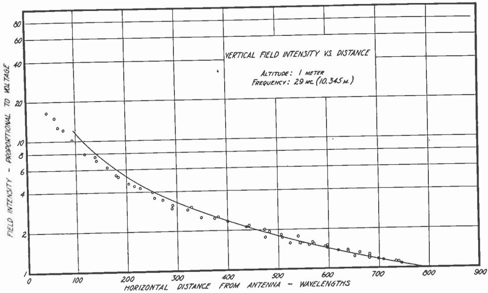
Fig. 2—Theoretical (Sommerfeld) and experimental vertical field intensity vs. horizontal distance from the antenna. Measurements made just over the surface of sea water.
