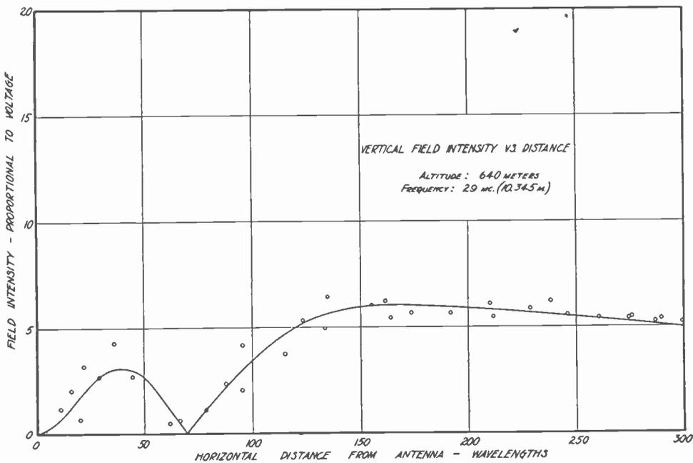
Fig. 16—Detailed theoretical (Strutt) and experimental vertical field intensity vs. horizontal distance from the antenna for altitude of 640 meters.
