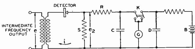
Fig. 3—Schematic diagram of general recorder circuit.
