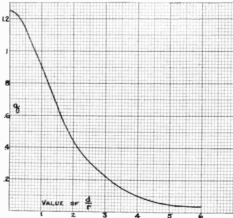
Fig. 6—Field constant for magnetic deflection coils.
