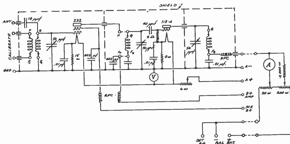
Fig. 20—Wiring diagram of measuring equipment used for determining relative field intensities.
