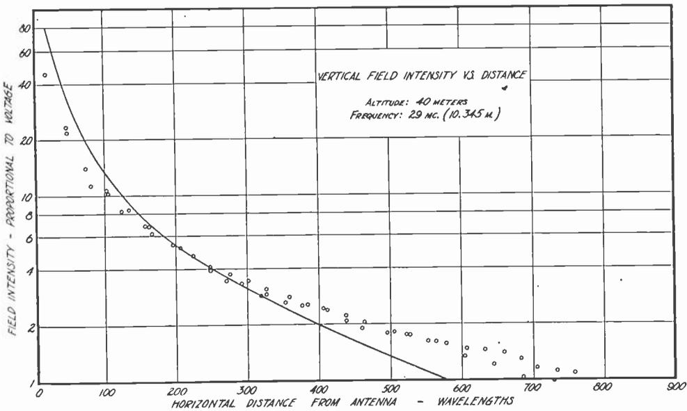
Fig. 3—Theoretical (Strutt) and experimental vertical field intensity vs. horizontal distance from the antenna for altitude of 40 meters.
