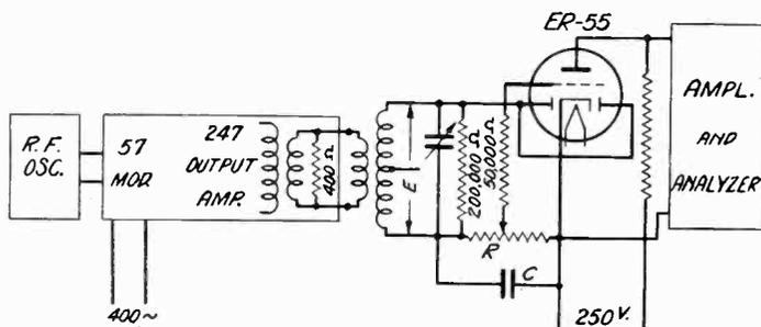
Fig. 1—Schematic diagram of apparatus used to measure detector distortion.
