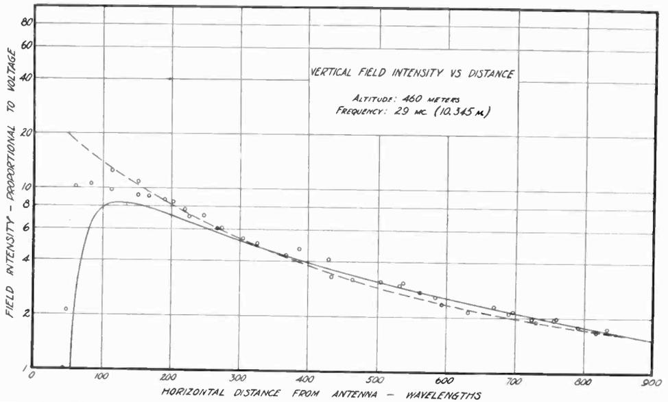
Fig. 8—Theoretical (solid curve: Strutt; dotted curve: Sommerfeld) and experimental vertical field intensity vs. horizontal distance from the antenna for altitude of 460 meters.
