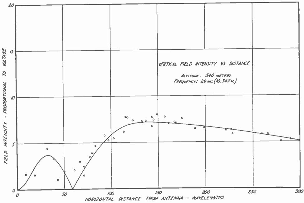
Fig. 15—Detailed theoretical (Strutt) and experimental vertical field intensity vs. horizontal distance from the antenna for altitude of 540 meters.
