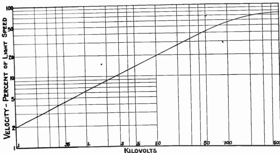
Fig. 3—Velocity curve.
