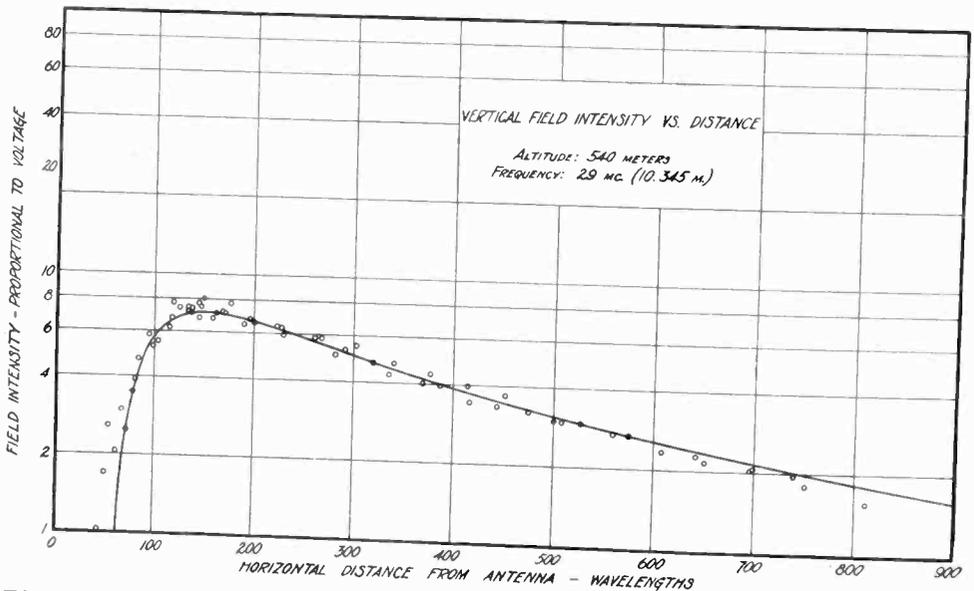
Fig. 9—Theoretical (Strutt) and experimental vertical field intensity vs. horizontal distance from the antenna for altitude of 540 meters.
