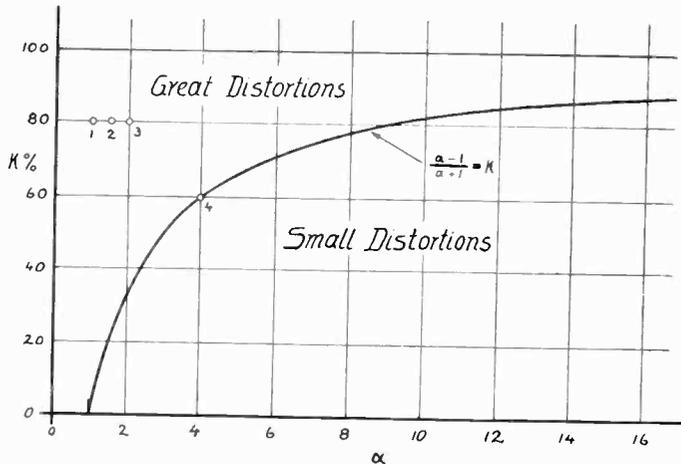
Fig. 6—Relationship between distortions, percentage modulation ( $k$ ), and field strength ratio ( $\alpha$ ). Points 1, 2, 3, and 4 correspond to Figs. 2, 3, 4, and 5, respectively.
