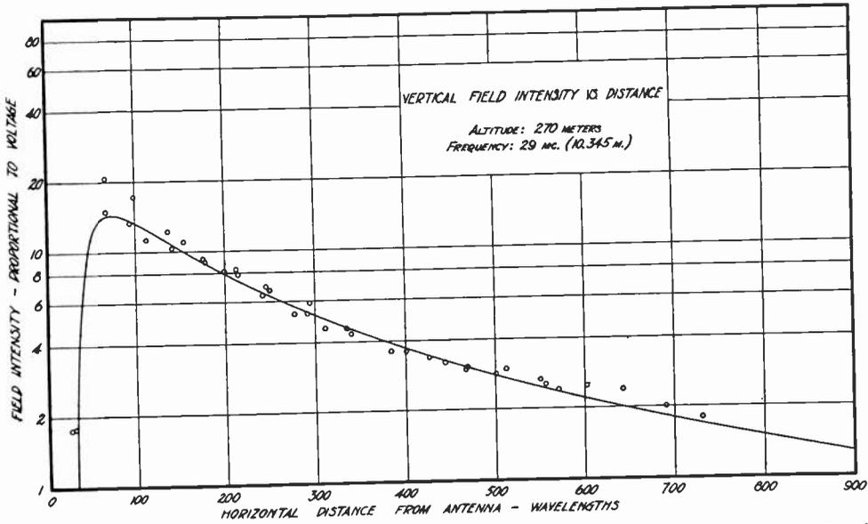
Fig. 6—Theoretical (Strutt) and experimental vertical field intensity vs. horizontal distance from the antenna for altitude of 270 meters.
