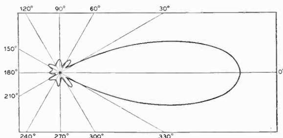
Fig. 3—Directional characteristic of array at 14.6 meters.
