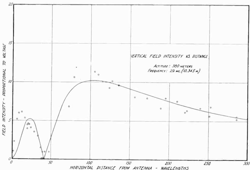
Fig. 13—Detailed theoretical (Strutt) and experimental vertical field intensity vs. horizontal distance from the antenna for altitude of 380 meters.
