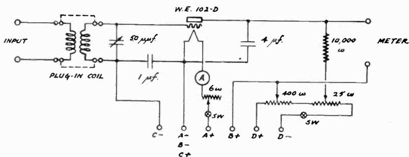
Fig. 23—Wiring diagram of vacuum tube voltmeter used for the calibration of the standard signal generator.
