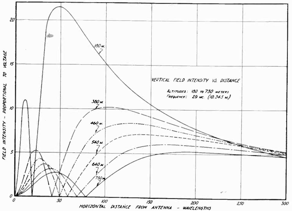
Fig. 18—Composite detailed theoretical (Strutt) vertical field intensity vs. horizontal distance from the antenna, curves for altitudes from 180 to 730 meters.
