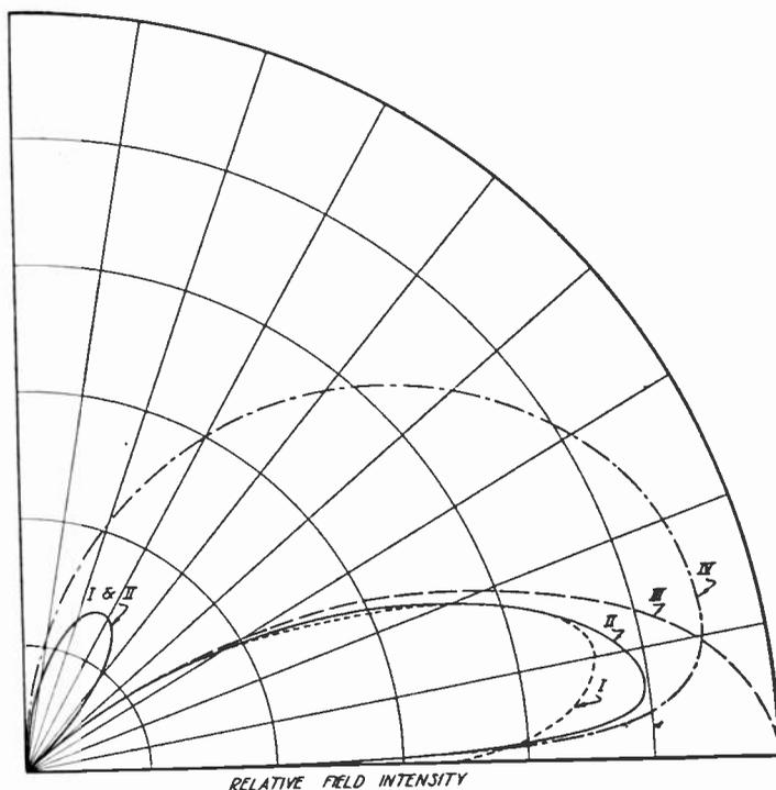
Fig. 19—Theoretical and experimental field intensity characteristics of vertical antenna in the vertical plane.
