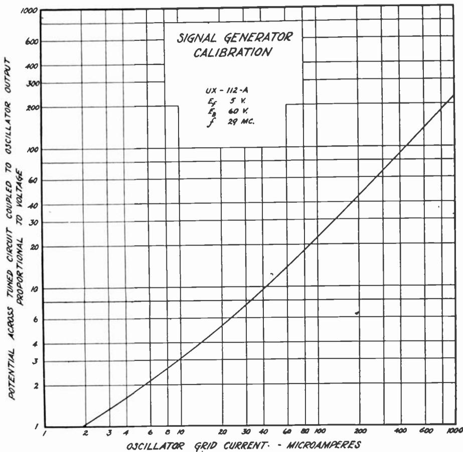
Fig. 22—Typical signal generator calibration curve.
