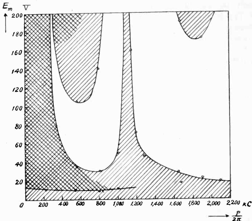
Fig. 10—State of mush (doubly shaded), state of quenching (shaded), and state without self-excitation (unshaded).
