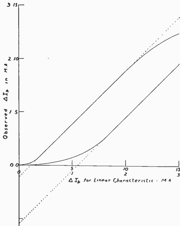
Fig. 9—Low and high range calibration curve of voltmeter.
