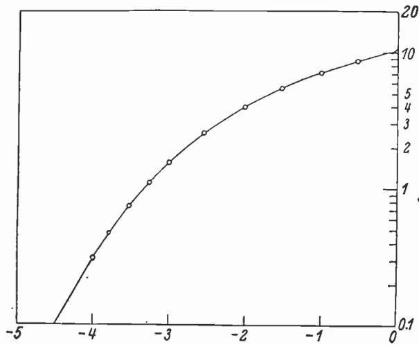
Fig. 4—Anode current  $i$  milliamperes (vertical) versus grid voltage  $V$  (horizontal) for Philips vacuum tube E 446. Points measured, curve calculated from  $i = 11.5 \cdot e^{0.28V} - 1.2e^{0.377V} + 0.18e^{-4.10(V+3.5)}$ ;  $R = 0$ ;  $V_{an} = 200V$ ;  $V_{screen} = 100V$ .
