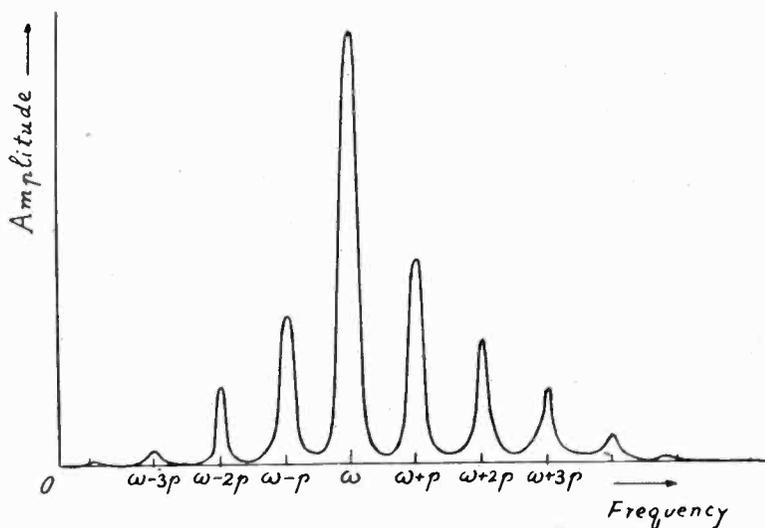
Fig. 5—Multiple resonance curve.
