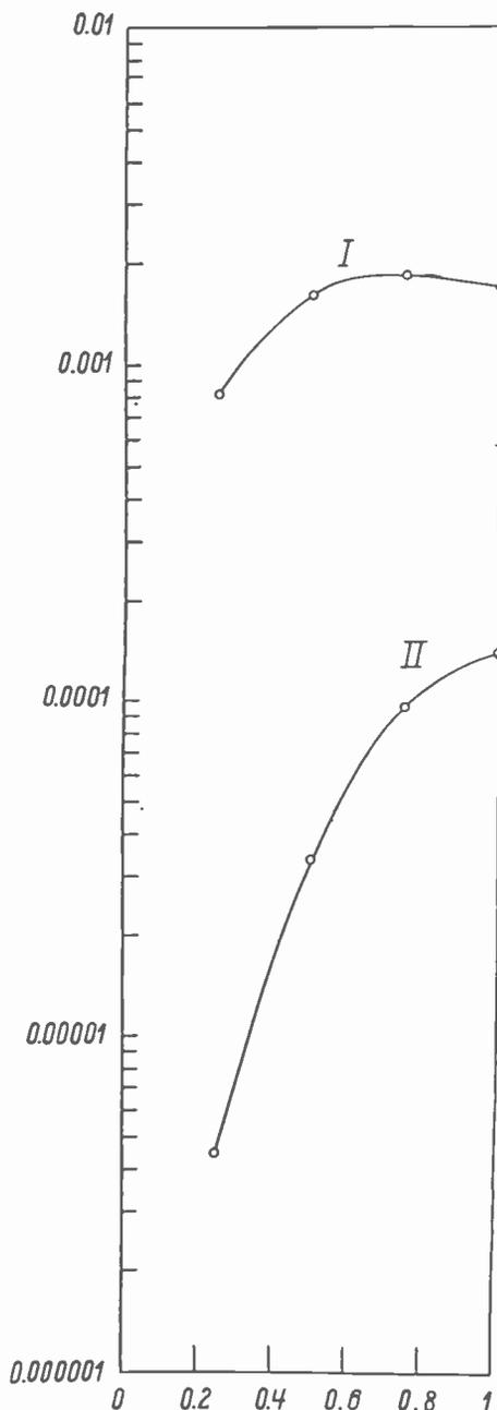
Fig. 7—Vertical axis, curve I = anode current component  $i_{2p}$  for  $M=0.3$ . Curve II = anode current component  $i_{3p}$  for  $M=0.3$ . Both curves related to vacuum tube E 452 T. Points measured, curves calculated. Horizontal axis, input signal amplitude  $E$ , while  $V_0 + 2E = -3.5$  volts.
