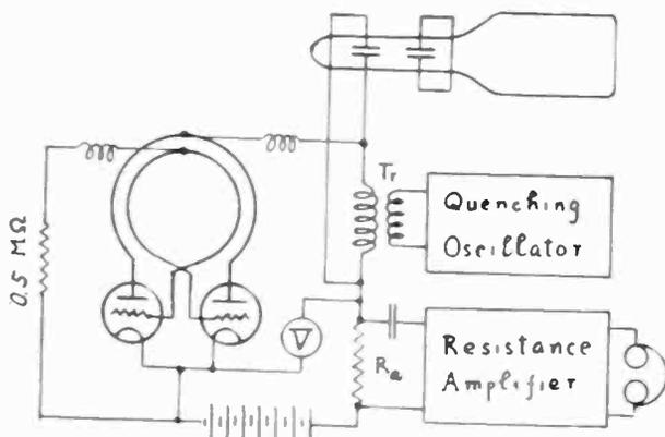
Fig. 7—Experimental arrangements.
