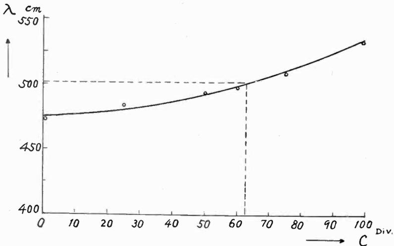
Fig. 18—Range of wave length of the receiver.
