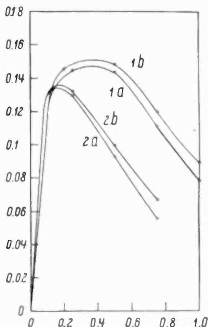
Fig. 6—Vertical axis, detection slope  $S$  divided by  $M$  (ma/volts); horizontal axis; input signal amplitude  $E$ , while  $V_0 + 2E = -3.5$  volts. Points measured, curves calculated. Curves 1 for tube E 452 T. Curves 2 for tube E 446. Curves 1a and 2a for  $M = 0.3$ . 1b and 2b for  $M = 0.8$ . Voltages and resistance as in Fig. 5.
