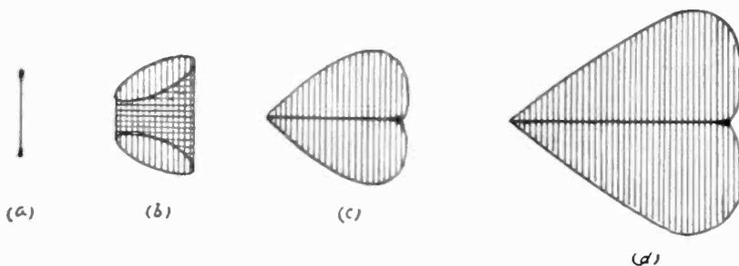
Fig. 14—Lissajous figures at  $E_p = 103V$ ,  $p/2\pi = 550$  kilocycles.
