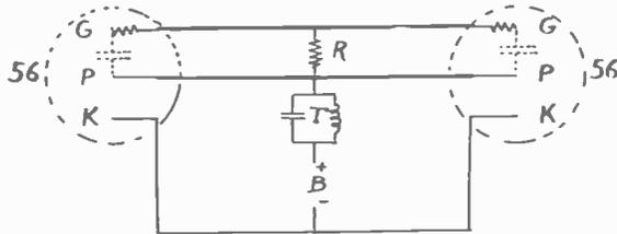
Fig. 3—Schematic circuit diagram of the regenerative oscillator.  $T$  = tuned circuit formed by single turn coil pictured in Fig. 1.  $R$  = 3000-ohm resistance. The operating voltage is from 70 to 100 volts; plate current varies from about 40 to 100 milliamperes. The inductance rods were of telescoping brass, spaced 3 centimeters, and about 20 centimeters long for the 188.8-centimeter wavelength.
