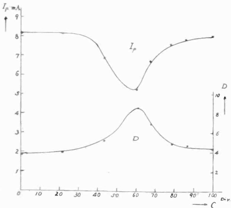
Fig. 27—Synchronization in the superregenerative receiver.
