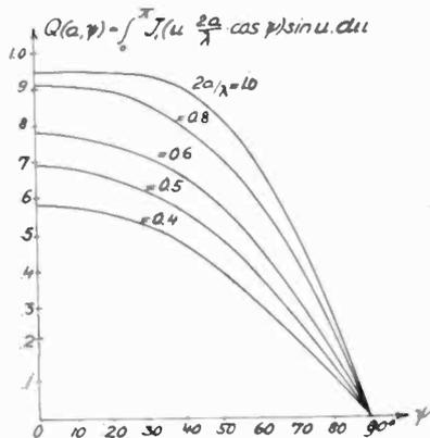
Fig. 8—Plot of the function  $Q(a, \psi) = \int_0^\pi J_1(u \cdot 2a/\lambda \cdot \cos \psi) \sin u \cdot du$ .
