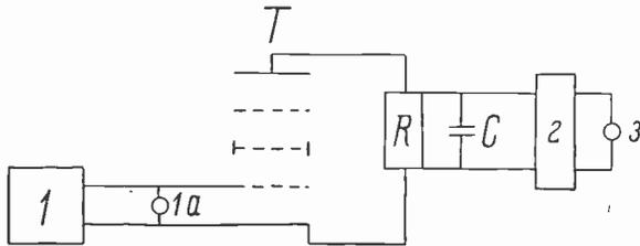
Fig. 2—Experimental set-up for measuring detector tubes. 1 is an oscillator of known depth of modulation. 1a is a voltmeter measuring the radio-frequency input to the tube  $T$ .  $R$  and  $C$  are as in Fig. 1. 2 is a filter circuit, passing only one audio frequency. 3 is a voltmeter for audio frequency.
