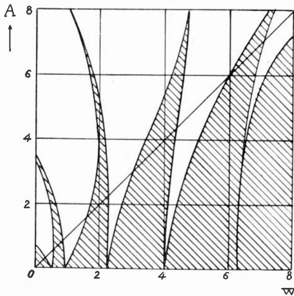
Fig. 2—Stable (shaded) and unstable (unshaded) regions of solution of Mathieu's equation.
