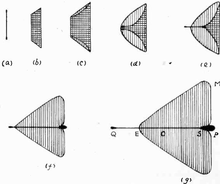
Fig. 12—Lissajous figures at  $E_p = 102V$ ,  $p/2\pi = 90$  kilocycles.
