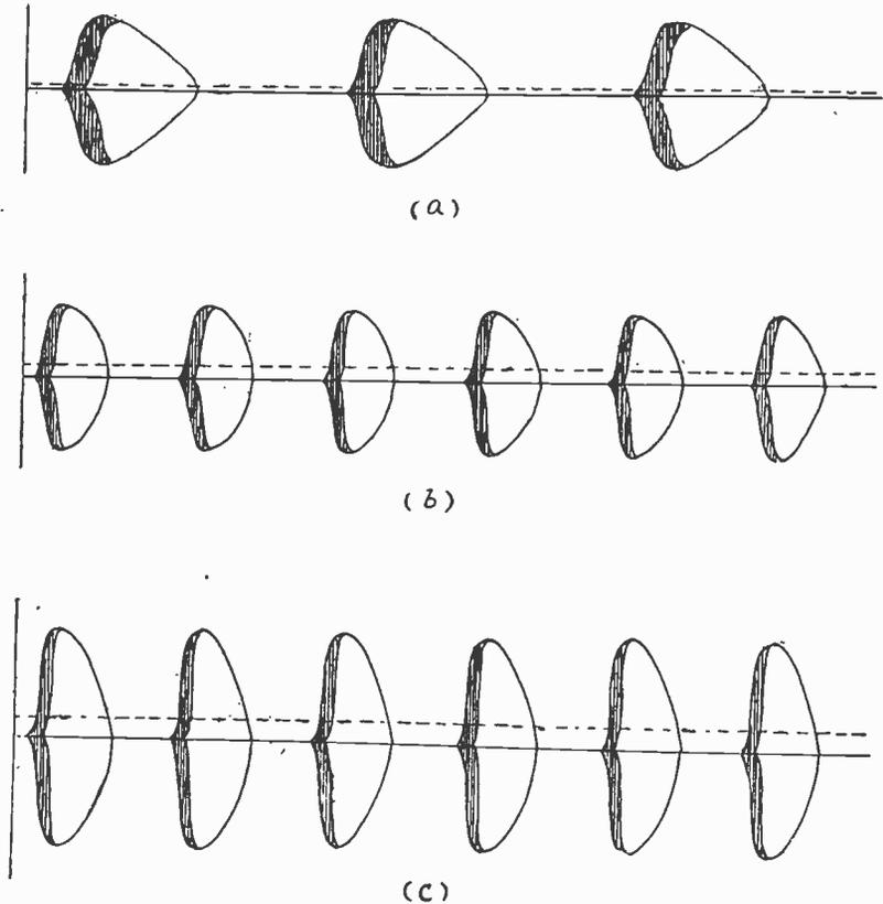
Fig. 39—Various modes of amplification by superregeneration.
