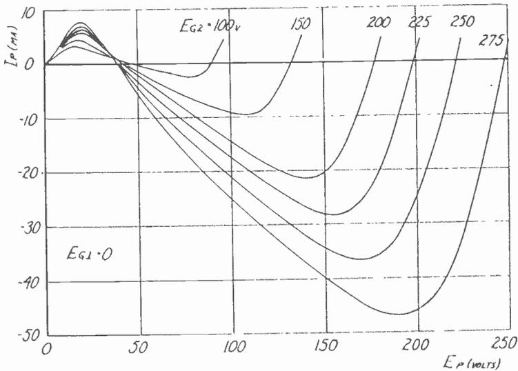
Fig. 3—Plate characteristics of the '65 tube as a dynatron showing the effect of the grid 2 voltage.
