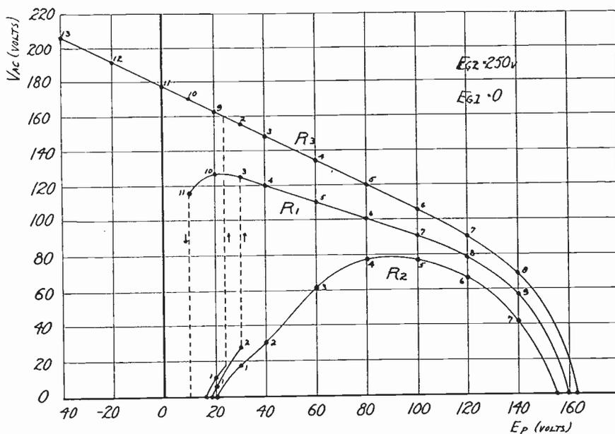
Fig. 19—Variation of oscillation voltage of the  $\mu 65$  for various direct plate voltages. (From Fig. 18.)
