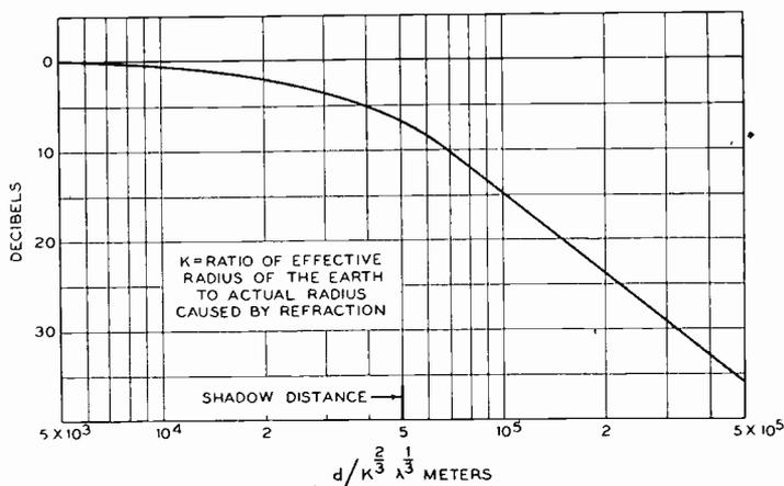
Fig. 10—Additional attenuation caused by the earth's shadow.
