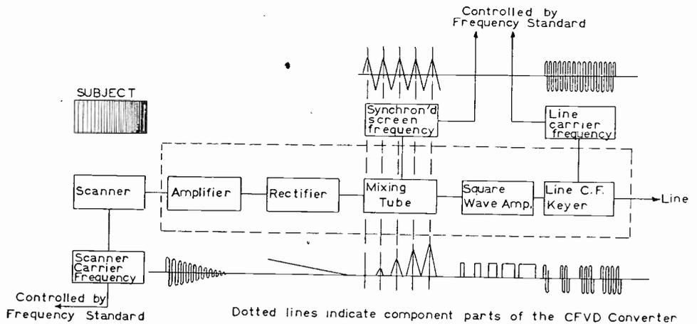
Fig. 14—Block diagram of constant-frequency variable-dot photoradio system.
