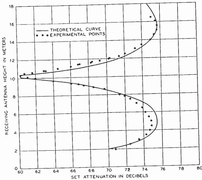
Fig. 5—Variation of received field with antenna height. •
