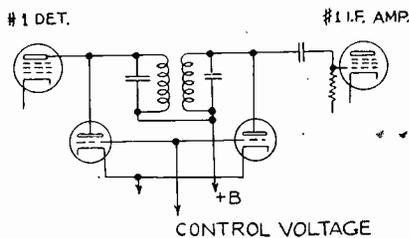
Fig. 3—No. 1 intermediate-frequency transformer.
