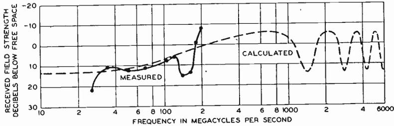
Fig. 19—Frequency characteristic of optical path Beer's Hill to Lebanon, N. J. The experimental points have been corrected to eliminate the effect of local reflections near the terminals as explained in the text.
