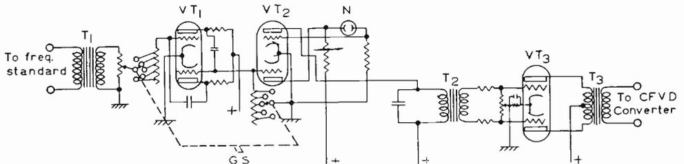
Fig. 16—Schematic diagram of synchronized screen-frequency unit.
