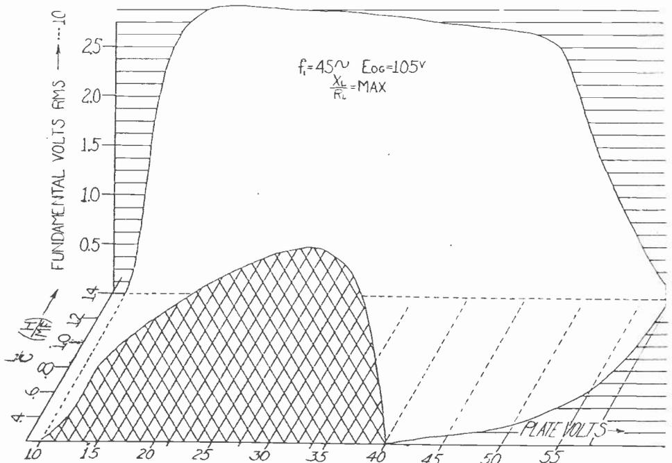
Fig. 28—Actual fundamental oscillation voltages for the '24.
