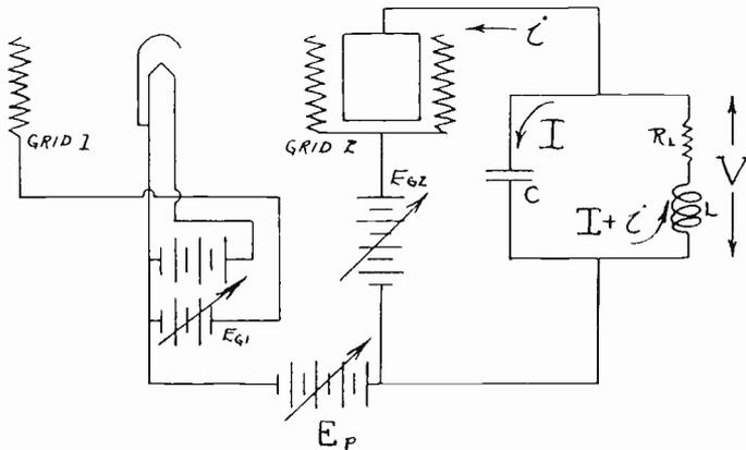
Fig. 1—The tetrode dynatron oscillator circuit.
