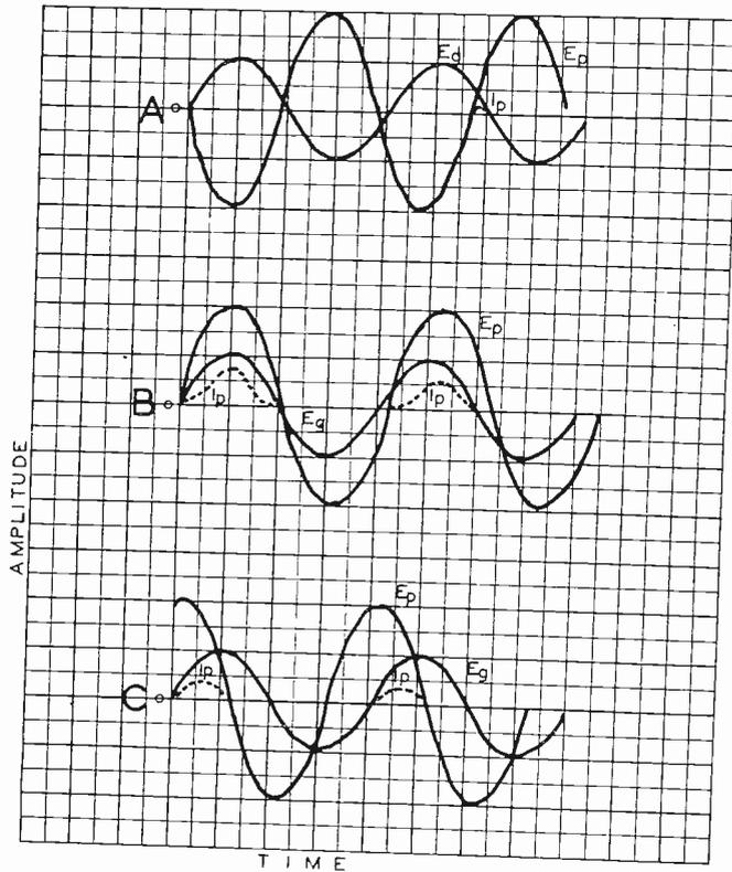
Fig. 7—Characteristic curves for thermionic brake.
