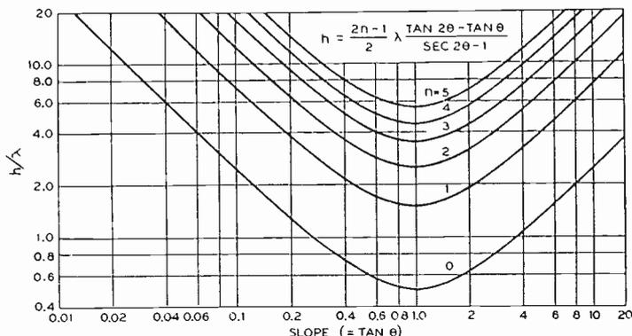
Fig. 14—Optimum heights for antennas above ground having a slope equal to  $\tan \theta$ . *Caution:* For large slopes, this applies only to horizontal antennas.
