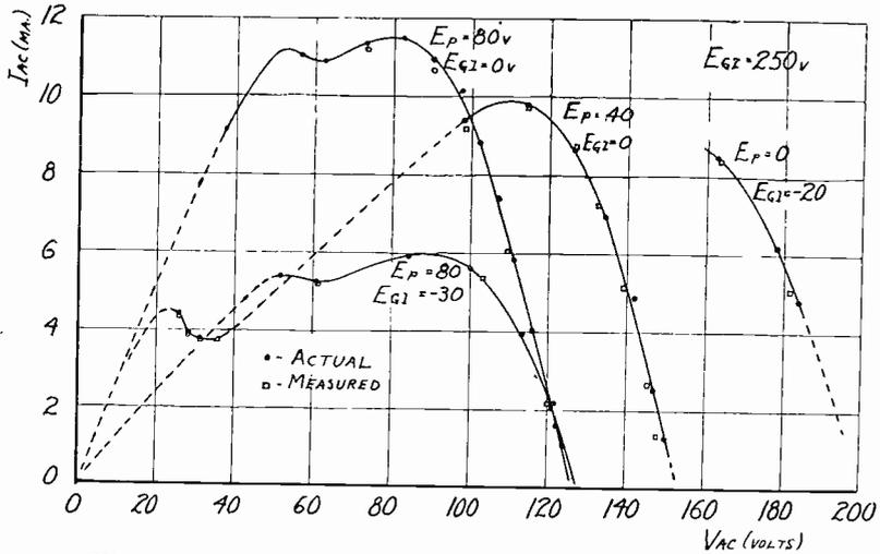
Fig. 26—Actual oscillation voltages with the '65.
