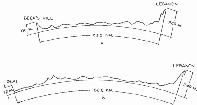
Fig. 15—Profiles of (a) optical path between Beer's Hill and Lebanon, (b) nonoptical path between Deal and Lebanon, (New Jersey).
