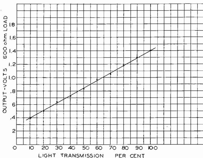
Fig. 12—Light response characteristic of RCAC BGM scanner.
