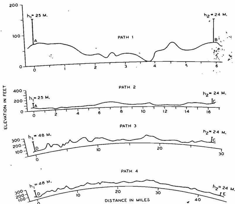
Fig. 3—Profiles of the level-terrain paths.
