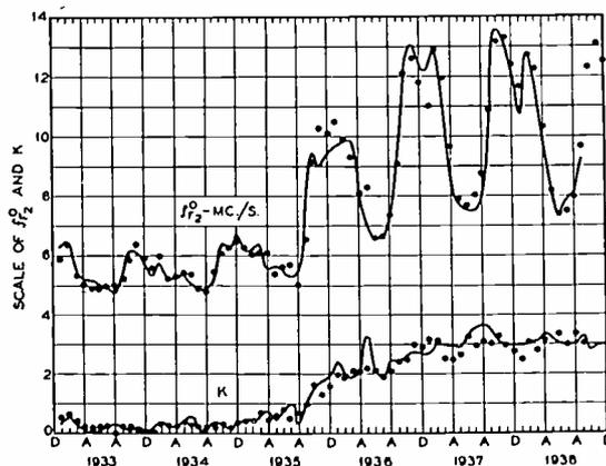
Fig. 2—Expected values of  $f_{F_2}^0$  (for 1300 E.S.T.) and  $K$  are given by curves, data by points.
