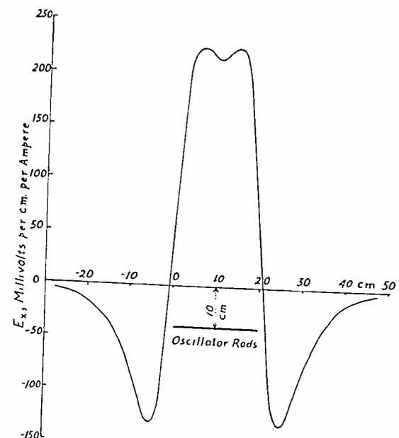
Fig. 3—Theoretical curve of the electric field along a conductor due to a loosely coupled oscillator. The oscillator length is 20 centimeters; the separation of its rods is 2 centimeters; it is coupled 10 centimeters from the parallel line. It is operating at a wavelength of 188.4 centimeters. A cosinusoidal current distribution is assumed.
