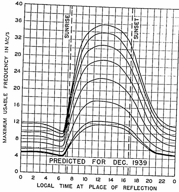
Fig. 4—Predicted maximum usable frequencies for dependable radio transmission via the regular layers, average for undisturbed days, for December, 1939.
