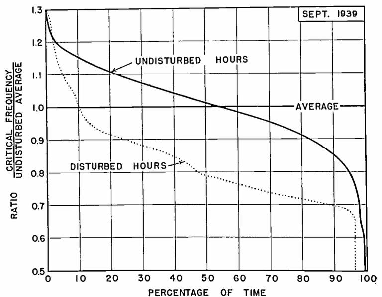
Fig. 3—Distribution of F- and  $F_2$ -layer maximum-wave critical frequencies (and approximately of maximum usable frequencies) about monthly average. Abscissas show percentage of time for which the ratio of the critical frequency to the undisturbed average exceeded the values given by the ordinates. The solid-line graph is for 425 undisturbed hours of observation; the dotted graph is for 59 disturbed hours of observation listed in Table I.
