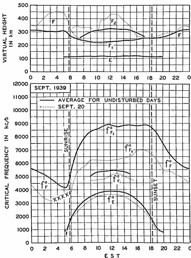
Fig. 1—Virtual heights and critical frequencies of the ionospheric layers, September 1939. The solid-line graphs are the averages for the undisturbed days; the dotted-line graphs are for the ionospheric storm day of September 20. The crosses represent the times on September 20 when the F-layer reflections were so diffuse that the critical frequencies could not be determined.
