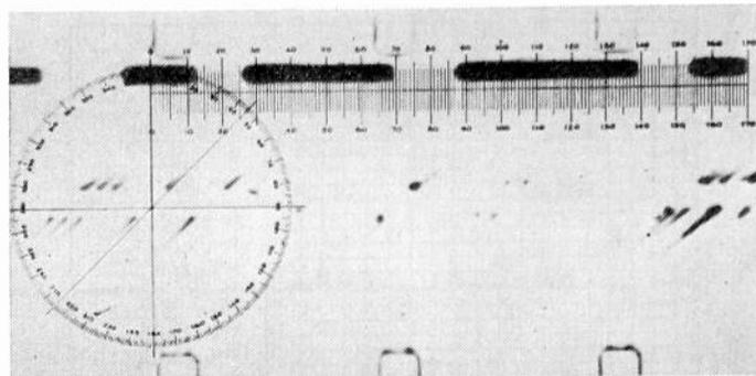
Fig. 3—Section of moving-film record superimposed on a compass rose and scale. Note direction of static crashes and synchronizing signal in continental code.
