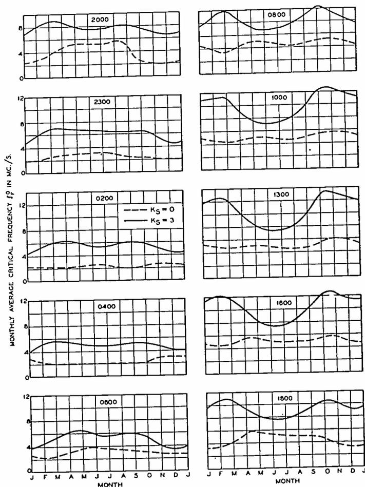
Fig. 6—Expected constant-time curves for hours indicated.  $K_s = 0$  for dashed curves and  $K_s = 3$  for solid curves.
