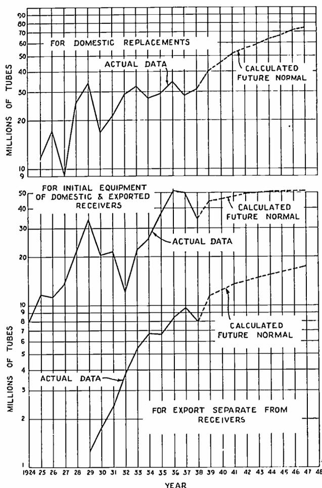
Fig. 7—Annual production of receiving vacuum tubes, for initial equipment, replacements, and export.
