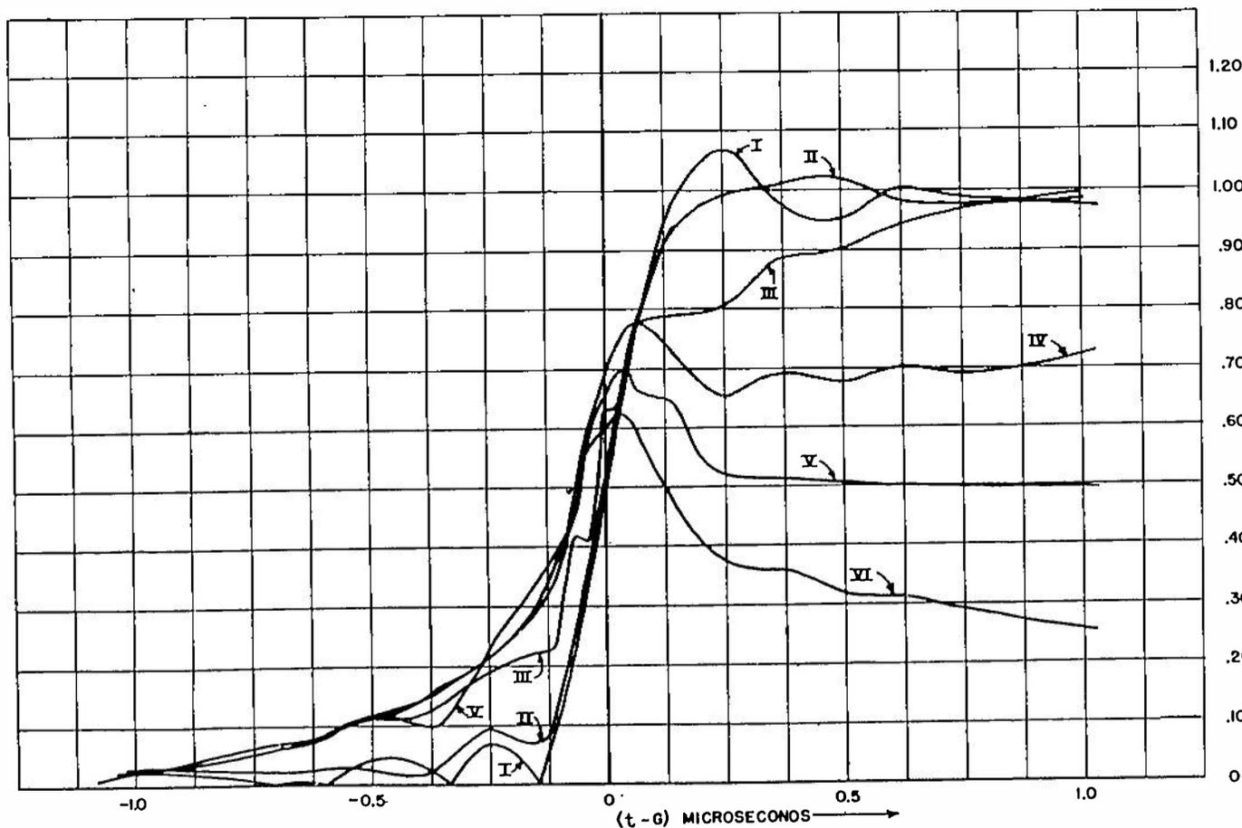
Fig. 5—Response to a unit-function signal.
