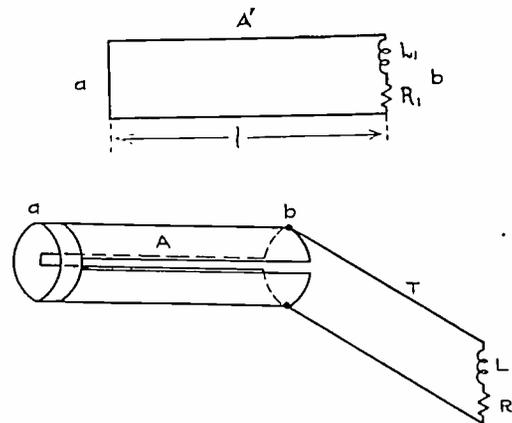
Fig. 2—Anode tank circuit with transmission line and load.
