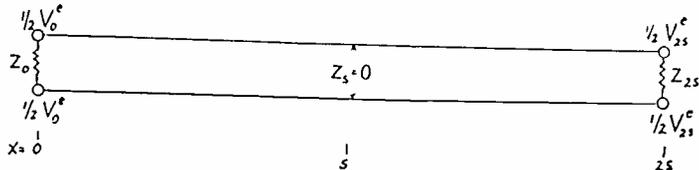
Fig. 2—Schematic diagram of a symmetrical oscillator.
