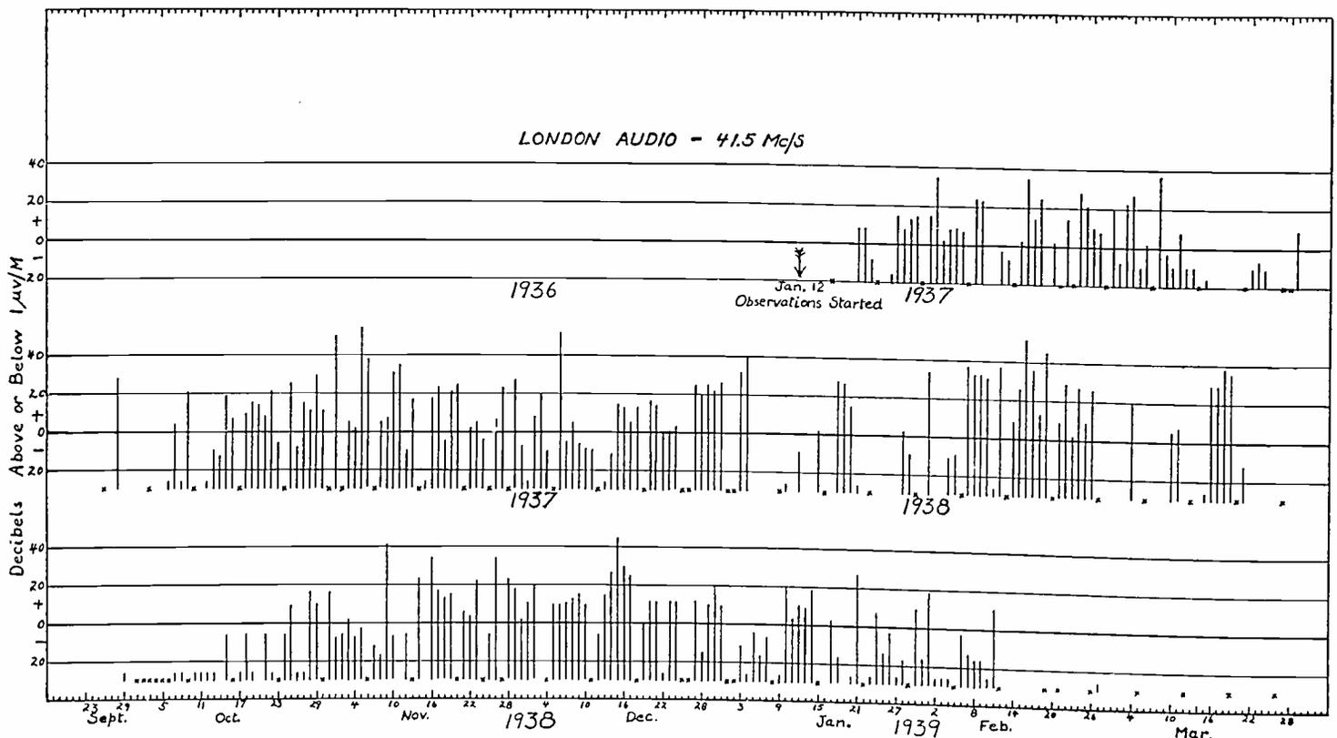
Fig. 5—Maximum signal strengths recorded from the London audio-frequency transmitter since January, 1937. The crosses indicate days on which no observations were made.
