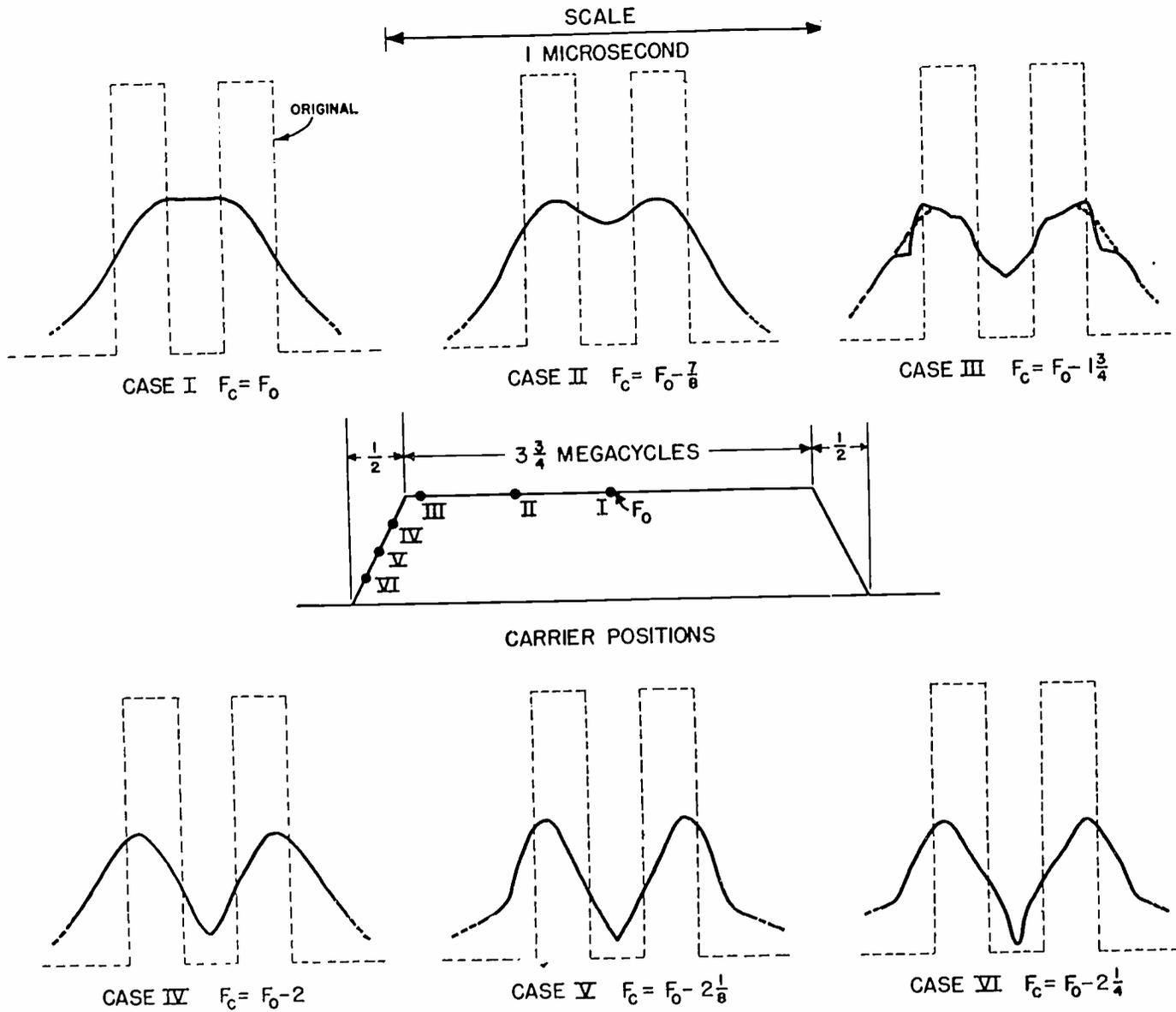
Fig. 8—Effect of carrier positions on the reproduction of detail.
