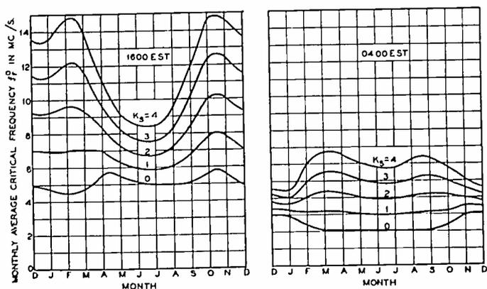
Fig. 5—Expected constant-time curves for 0400 and 1600 E.S.T. based on curves similar to those of Fig. 1 and values of  $K_s$  indicated.
