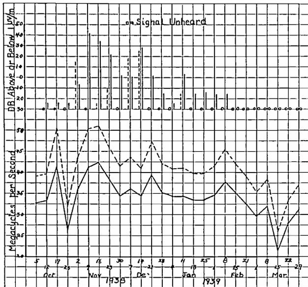
Fig. 3—Comparison of observed signal strengths to maximum usable frequencies interpolated for 2700 kilometers. Vertical solid lines of the upper plot represent maximum signal strengths observed from London on 41.5 megacycles. Broken lines represent the same for 45 megacycles. The broken-line plot represents the maximum-usable-frequency curve after applying the Lorentz correction term.
