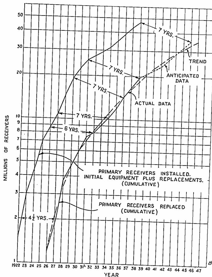
Fig. 3—Primary receivers installed and replaced.
