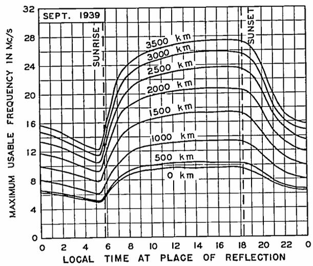
Fig. 2—Maximum usable frequencies for dependable radio transmission via the regular layers, average for undisturbed days for September, 1939.
