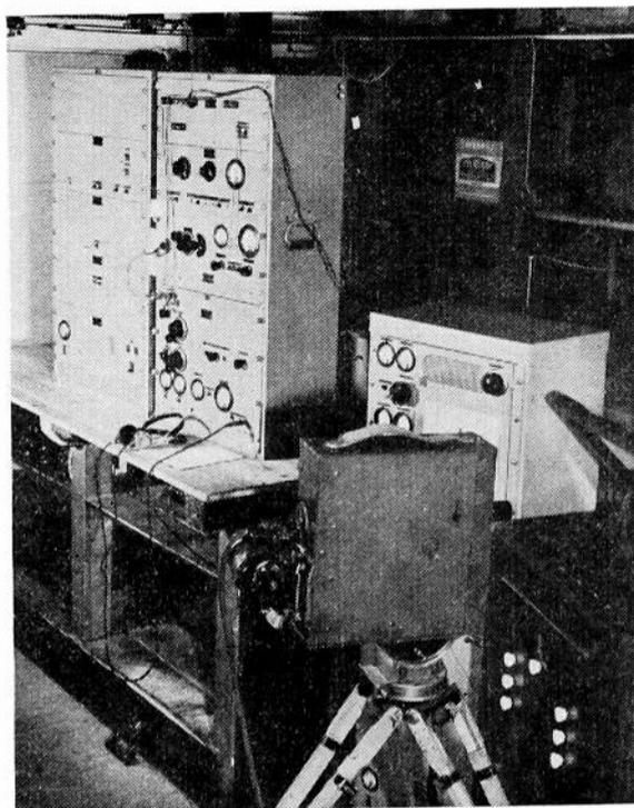
Fig. 1—Ultra-high-frequency receiving equipment used for field-strength measurements and visual monitoring.
