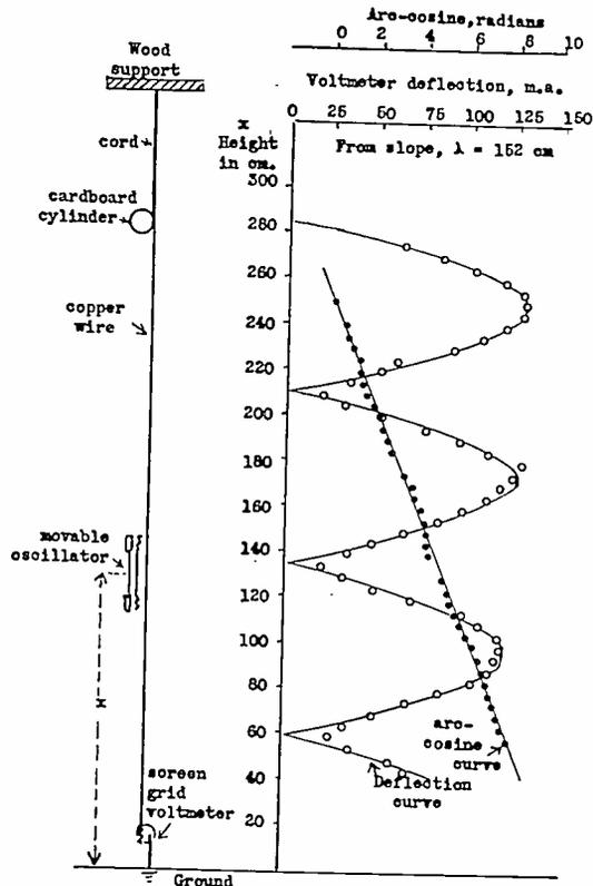
Fig. 6—Deflection of the voltmeter at the base of the vertical antenna as a symmetrical oscillator is hoisted along it.
