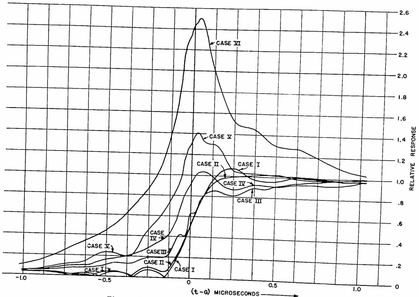
Fig. 6—Normalized response to a unit-function signal.
