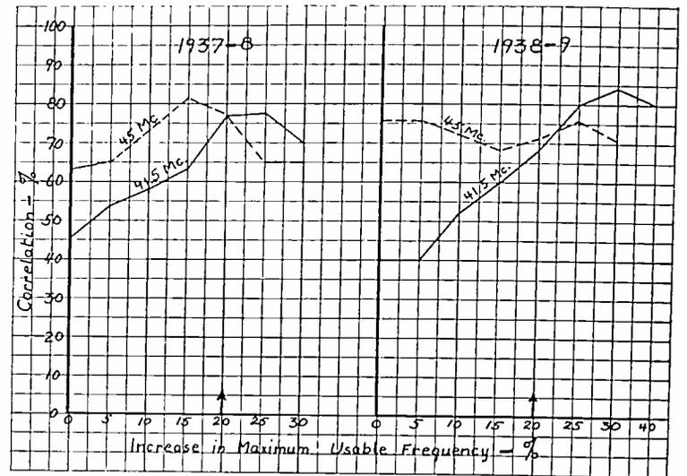
Fig. 4—Per cent correlation obtained by raising the maximum usable frequency curve by 5-per-cent increments. The arrows indicate the value determined from the Lorentz correction term.
