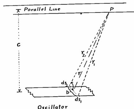
Fig. 4—Diagram to illustrate relative positions of the parallel conductors in the oscillator and in the parallel line. The electric and vector potential fields are to be calculated at  $P$ .
