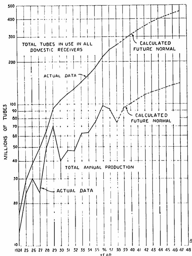
Fig. 6—Total annual production of vacuum tubes for broadcast receivers and total number of tubes in use in all domestic receivers.
