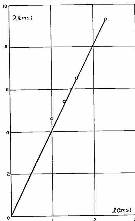
Fig. 8—Variation of wavelength with anode length.
