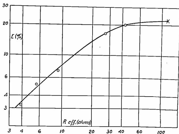
Fig. 9—Variation of efficiency with load resistance.
