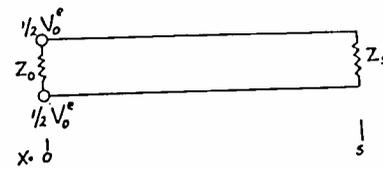
Fig. 1—Schematic diagram of an unsymmetrical oscillator.
