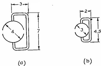
Fig. 1—Typical tank circuits for older type magnetrons.
