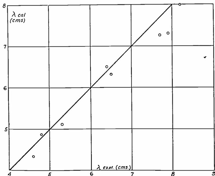
Fig. 7—Comparison of observed and calculated values of wavelength.
