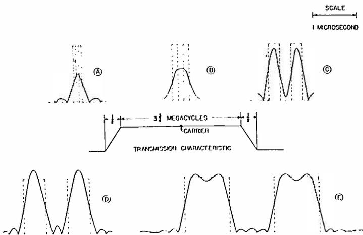
Fig. 9 - Scale drawing showing improved detail as spacing is increased. Carrier at center of pass band.
