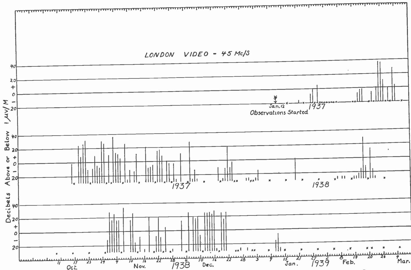
Fig. 6—Maximum signal strengths recorded from the London video-frequency transmitter since January, 1937. The crosses indicate days on which no observations were made.
