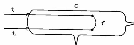
Fig. 6—Hydrogen-filled load lamp.
