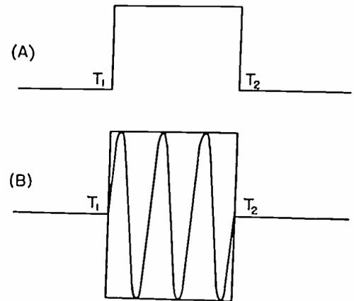
Fig. 2—The fundamental pulse (A) As video frequency. (B) As modulating a radio-frequency carrier.
