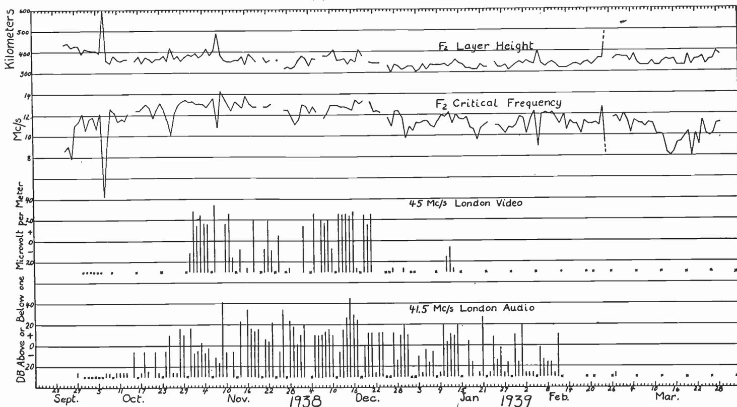
Fig. 2—Comparison of  $F_2$ -layer height and critical frequency to observed maximum signal strengths from London television audio- and video-frequency channels. The crosses indicate days on which no observations were made.
