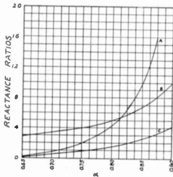
Fig. 10—Reactance ratios for the networks of Figs. 8 and 9 plotted as a function of  $\alpha = X_{L1}/X_{C1}$ ; A is a plot of  $X_4/X_{L1}$ ; B is a plot of  $X_2/X_{L1}$ ; and C is a plot of  $X_3/X_{L1}$ .
