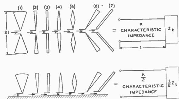
Fig. 2—The input impedance of a conical antenna of any size is equal to the input impedance of a uniform transmission line with a certain "output" impedance  $Z_i$ . The input impedance of a thin antenna of any shape may be similarly represented, except that the characteristic impedance will be variable.
