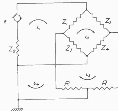
Fig. 5—The bridge or lattice type of balancing network.
