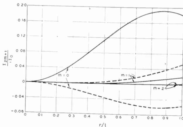
Fig. 17—Secondary current waves for  $K=1000$  and  $l=\lambda/2$ . The solid curves show the components in phase with the dominant current  $I_0 \sin \beta(l-r)$ , and the dotted curves show the quadrature components.
