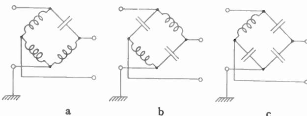
Fig. 7—Various lattice types of balancing networks.
