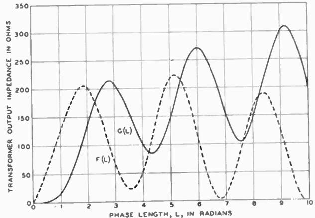
FIG. 9—The real and the imaginary parts of the "transformed" output impedance  $K^2/Z_i = G(L) + iF(L)$ , where  $L = 2\pi l/\lambda$ .
