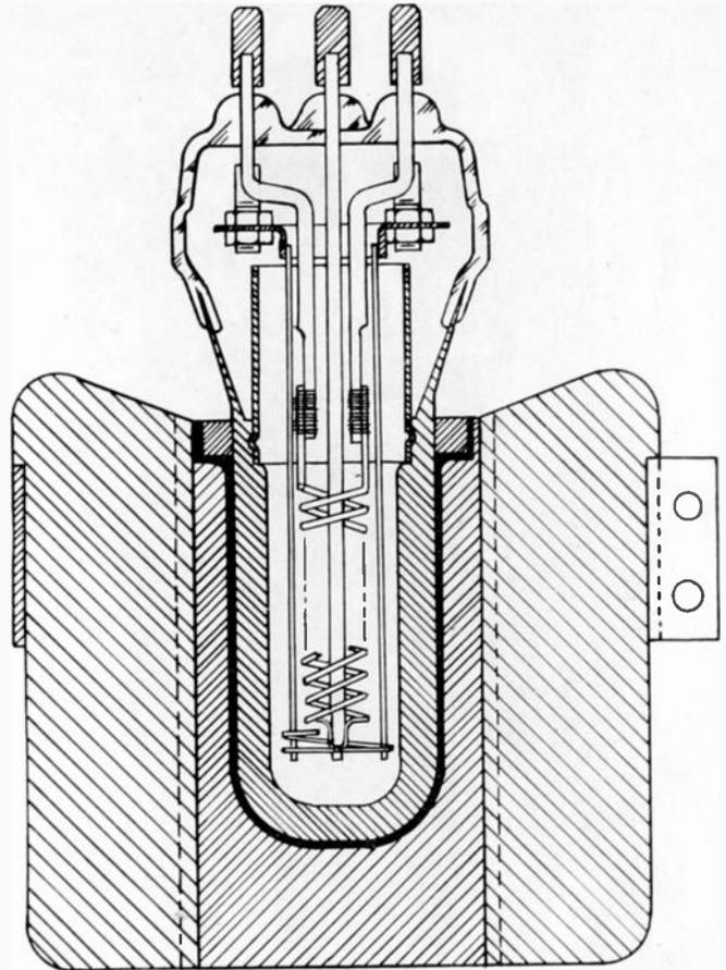
Fig. 3—GL-8002-R—transmitting tube, cross-sectional view, full scale.
