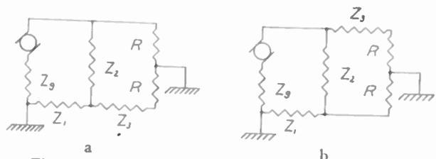
Fig. 2—Alford networks for matching a single-ended generator to a balanced load.
