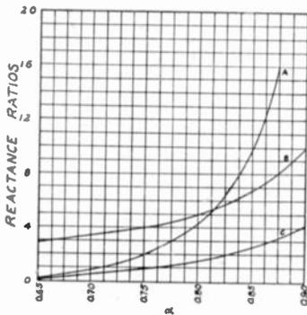
Fig. 10—Reactance ratios for the networks of Figs. 8 and 9 plotted as a function of  $\alpha = X_{L1}/X_{C1}$ ; A is a plot of  $X_4/X_{L1}$ ; B is a plot of  $X_2/X_{L1}$ ; and C is a plot of  $X_3/X_{L1}$ .
