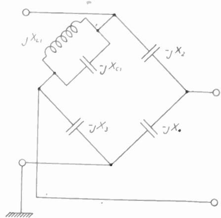
Fig. 8—Lattice type of balancing network adapted for use in the plate circuits of class C amplifiers.
