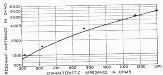
Fig. 26—The resonant impedance of cylindrical antennas is a function of  $K$ , when  $l$  is in the vicinity of  $\lambda/2$ .
