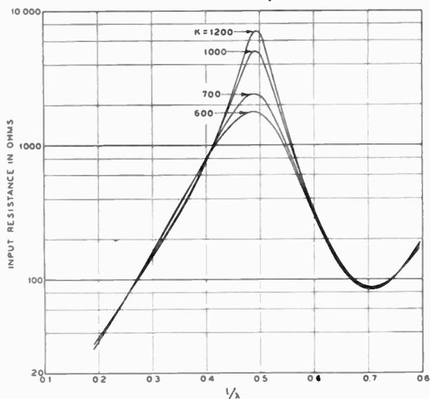
Fig. 13—The input resistance of conical antennas.
