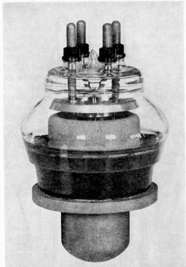
Fig. 7—GL-880—transmitting tube.
