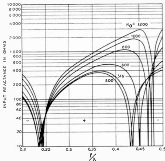
Fig. 24—The input reactance of cylindrical antennas in free space. For vertical antennas over a perfectly conducting ground divide the ordinates  $K_a$  by 2.
