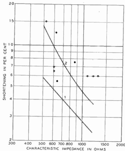
Fig. 27—The resonant length of cylindrical antennas in free space. Curve 1 is for the principal resonance. Curve 2 is for the second resonance. The ordinates represent the required shortening in per cent.
