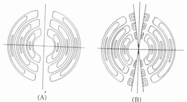
Fig. 6—Electric lines for the first-order transverse magnetic spherical waves: (A) lines in free space; (B) lines in the presence of two coaxial conical conductors.
