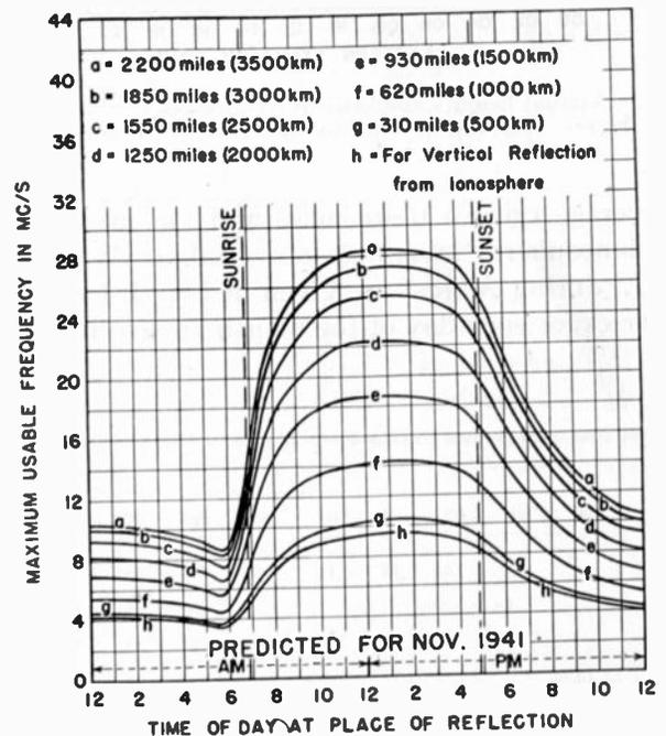
Fig. 2—Predicted maximum usable frequencies for dependable radio transmission via the regular layers average for undisturbed days, for November, 1941. For information on use in practical radio transmission problems, see the pamphlets "Radio transmission and the ionosphere" and "Distance ranges of radio waves," obtainable from The National Bureau of Standards, Washington, D. C., on request.
