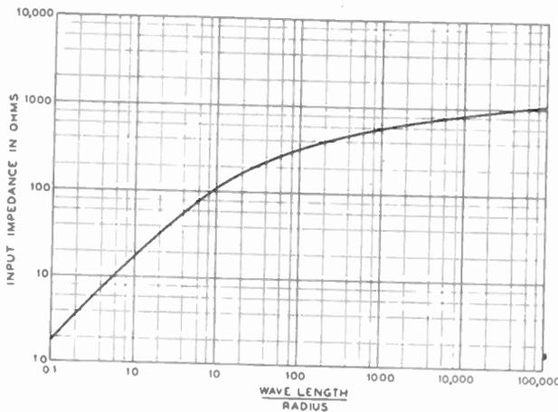
Fig. 22—The input impedance of the infinitely long cylindrical wire. For  $0.1 < \lambda/2a \leq 3$ , this curve has been computed by numerical integration from (164); for  $\lambda/2a \geq 500$ , the curve has been computed from the approximate equation (165); then, the two curves have been freely joined together.
