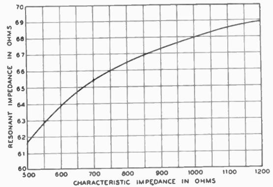
Fig. 25—The resonant impedance of cylindrical antennas as a function of  $K$ , when  $l$  is in the vicinity of  $\lambda/4$ .
