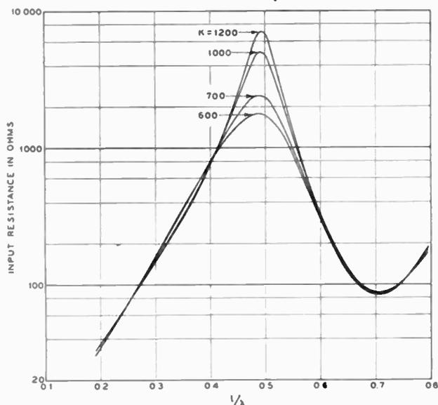
Fig. 13—The input resistance of conical antennas.
