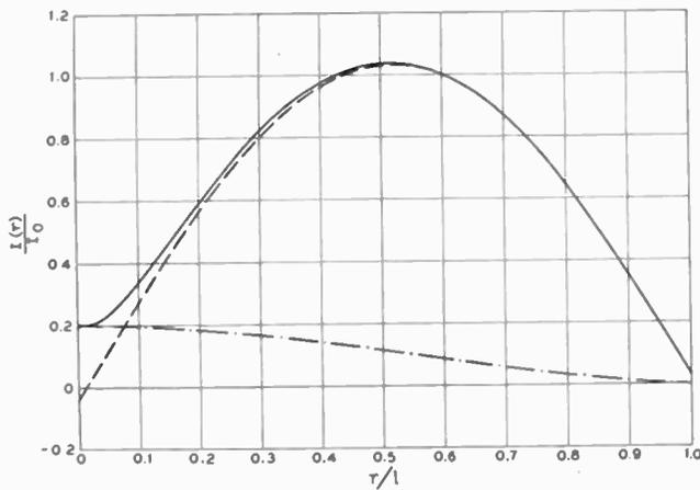
Fig. 18—The total current in the antenna of length  $2l = \lambda$ ;  $K = 1000$ . The solid curve represents the amplitude of the total current; the dash curve represents the amplitude of the component in phase with  $I_0$  and the dash-dot curve is the amplitude of the quadrature component.
