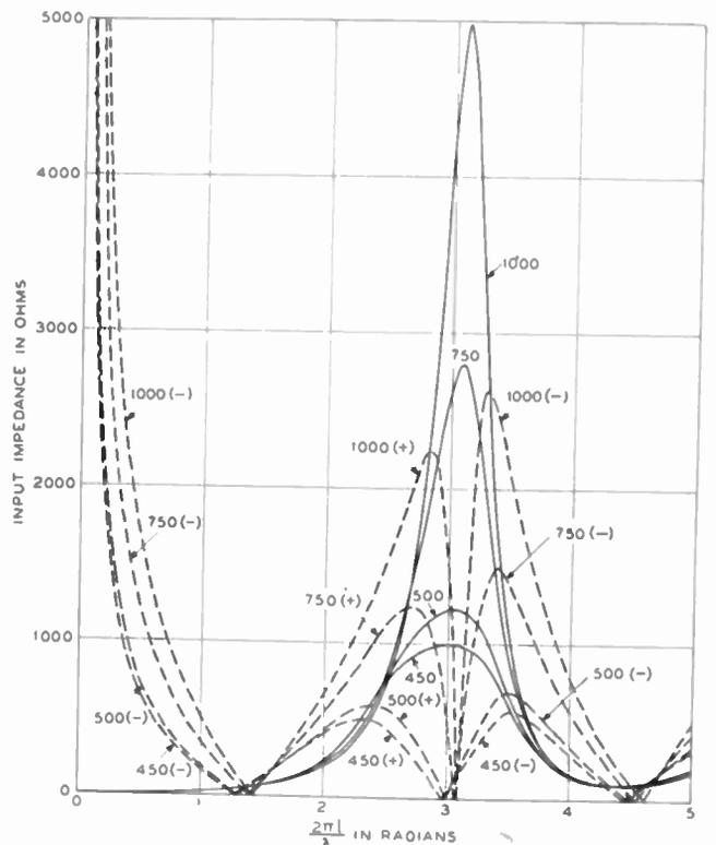
Fig. 12—The input impedance of conical antennas as a function of  $2\pi l/\lambda$  and  $K$ . Solid curves represent the real component and the dotted curves the imaginary.
