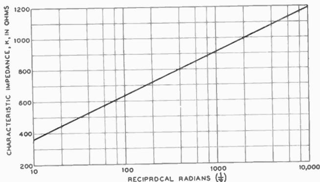
Fig. 4—The characteristic impedance of conical antennas of types shown in Fig. 3(B) as a function of the reciprocal cone angle  $\psi = a/l$ , where  $l$  is the length of the cone and  $a$  is its maximum radius.
