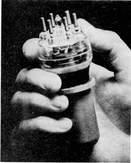
Fig. 1—GL-8002—transmitting tube.
