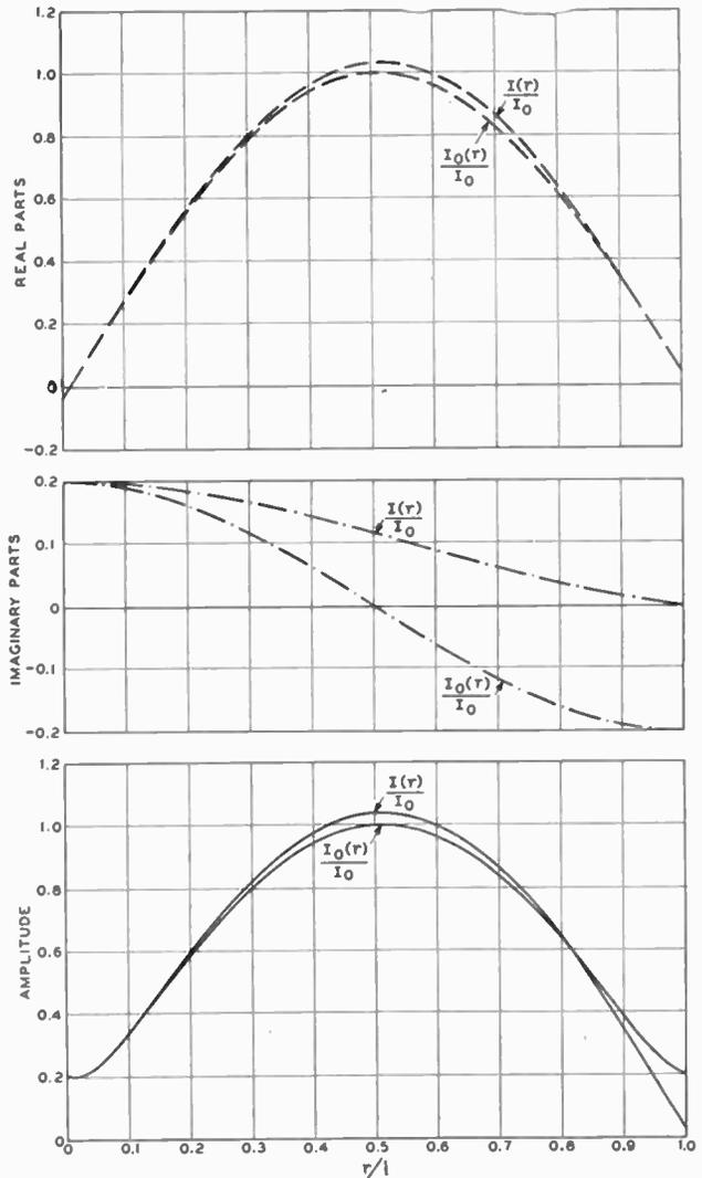
Fig. 19—Curves for the total current and the principal current.
