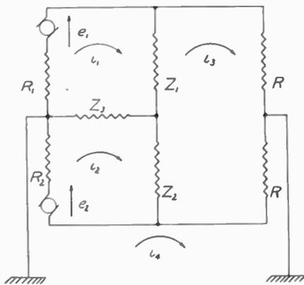
Fig. 3—Method of obtaining balanced voltages across a balanced load where the generator is partly unbalanced.
