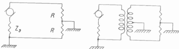
Fig. 1 (a) Incorrect method of connecting a single-ended generator to a balanced load. (b) Correct method.
