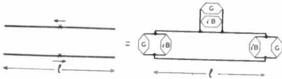
Fig. 32—The equivalent circuit for two parallel wires, open at both ends and energized in push-pull.
