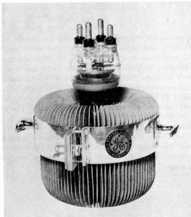
Fig. 6—GL-889-R—transmitting tube.
