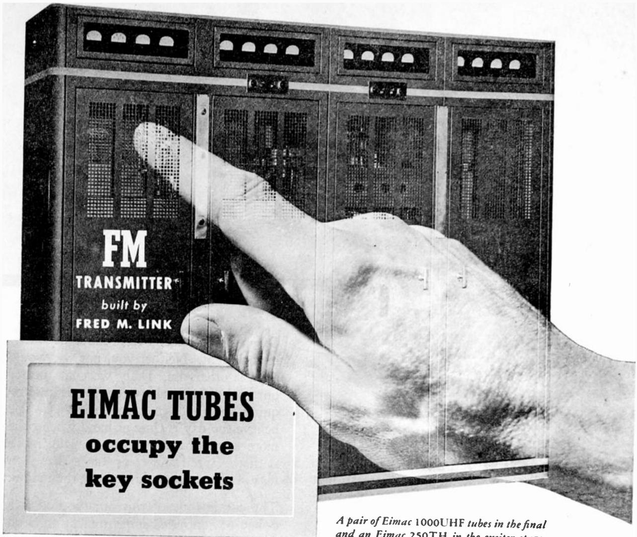
*A pair of Eimac 1000UHF tubes in the final and an Eimac 250TH in the exciter stage.*
