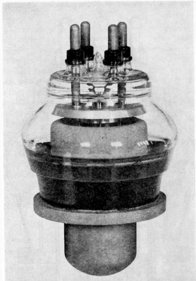
Fig. 7—GL-880—transmitting tube.
