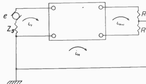
Fig. 4—General 4-terminal network for obtaining balanced voltages across a balanced load when the generator is single-ended; the network must satisfy the requirement that  $i_n = 0$ .
