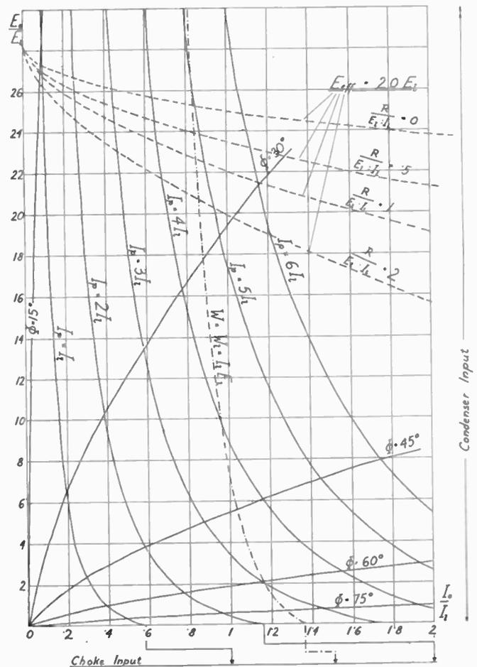
Fig. 2—Universal diagram showing the dynamic characteristics and permissible limits of output for full-wave condenser-input rectifiers.
