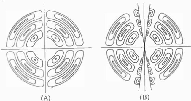
Fig. 7—Electric lines for the second-order transverse magnetic spherical waves: (A) lines in free space; (B) lines in the presence of two coaxial conical conductors.
