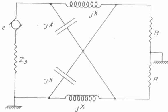
Fig. 6—The symmetrical lattice type of balancing network. The output from this network is balanced for any degree of generator unbalance.
