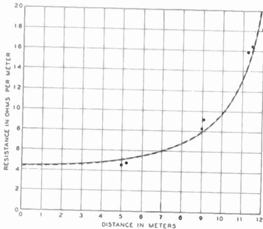
Fig. 29—Distribution of radiation resistance in the current-charge transmission equations. The calculated curve is for  $2l = \lambda/2$ ; the experimental points, obtained from Feldman, are for  $2l \approx 2.5\lambda$ .
