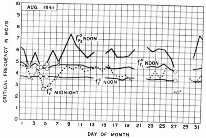
Fig. 4—Midnight and noon critical frequencies for each day of August. Open circles indicate critical frequencies observed during ionospheric storms. Sizes of circles represent approximately the severity of the storms.
