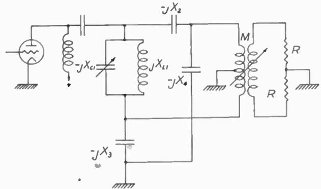
Fig. 9—The balancing network of Fig. 8 incorporated in the plate circuit of a class C amplifier.
