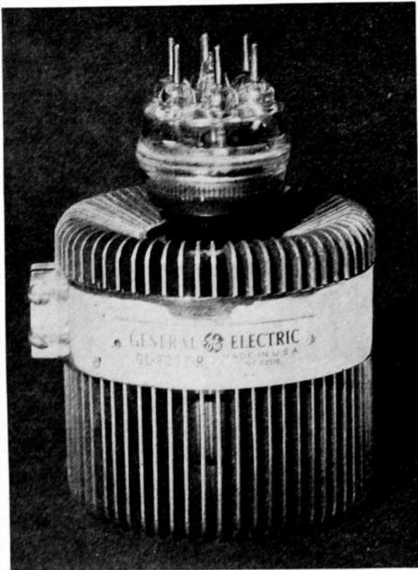
Fig. 2—GL-8002-R—transmitting tube.
