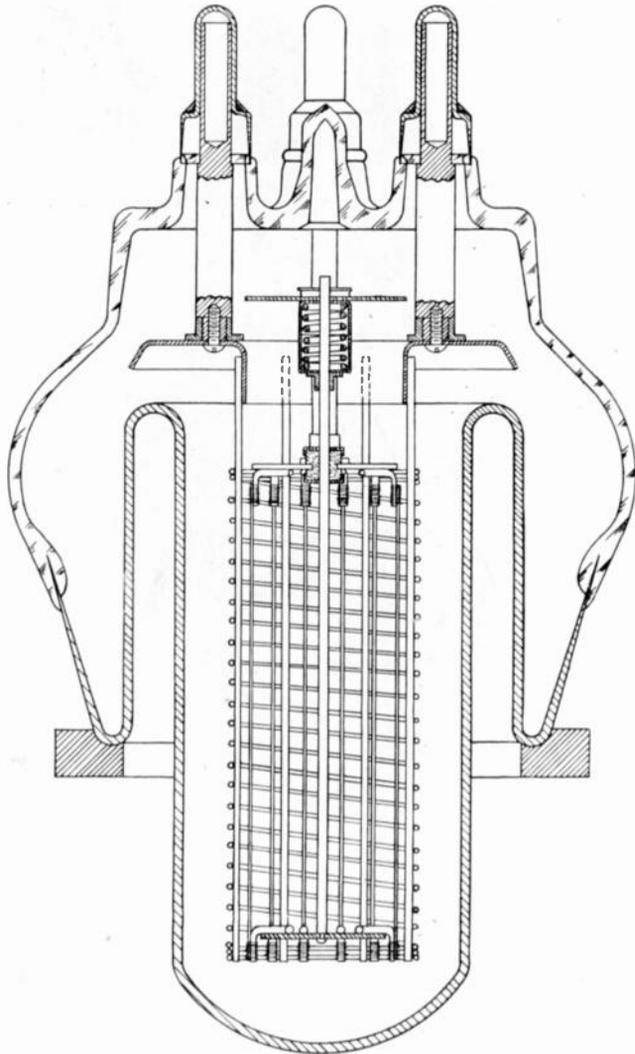
Fig. 8—GL-880—transmitting tube, cross-sectional view, full scale.
