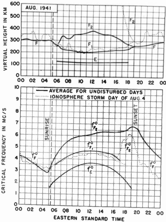
Fig. 3—Virtual heights and critical frequencies of the ionospheric layers, observed at Washington, D. C., August, 1941.
