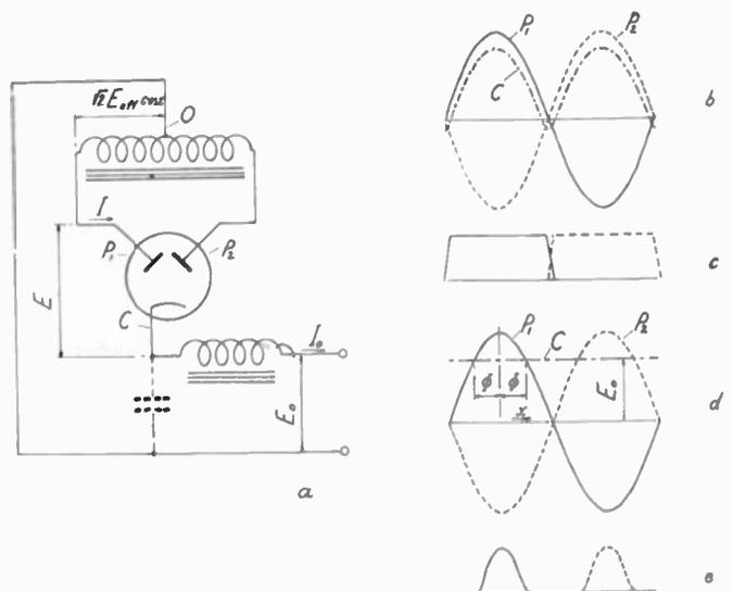
Fig. 1—Fundamentals. a. Schematic of double-wave rectifier (in choke input the dotted condenser is disconnected). b. Time curves of voltage in choke-input service. c. Time curves of valve currents in choke-input service. d. Time curves of voltages in condenser-input service. e. Time curves of valve currents in condenser-input service.
