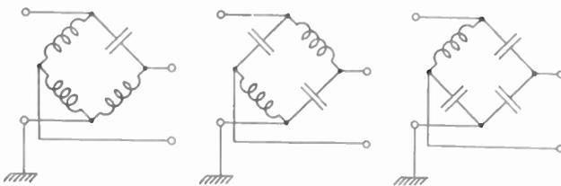
Fig. 7—Various lattice types of balancing networks.
