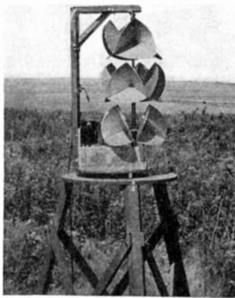
Fig. 8—Triple-turret reflector, in which each turret rotates with a predetermined speed. The result in the receiver is that particular reeds in the frequency meter become excited.
