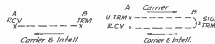
Fig. 1—A comparison between conventional direct-power communication (a) and the new reflected-power communication (b), in which reradiation provides the carrier for the signal.
