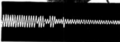
Plot made on Type 314 of starting current of small synchronous motor. (Note variation in current as the rotor "hunts" for its synchronous speed).
