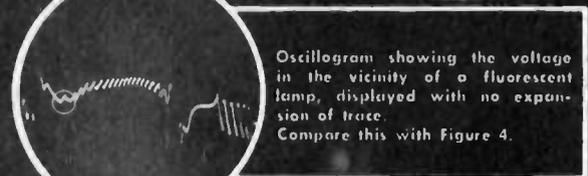
Oscillogram showing the voltage in the vicinity of a fluorescent lamp, displayed with no expansion of trace. Compare this with Figure 4.
