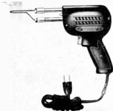
Previously held to 135 watts, due to bulk and weight of the transformer, the new guns have a 250-watt capacity by use of a machine that winds the transformer core from strip steel onto the primary and secondary coils.
