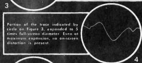
Portion of the trace indicated by circle on Figure 3, expanded to 5 times full-screen diameter. Even at maximum expansion, no on-screen distortion is present.
