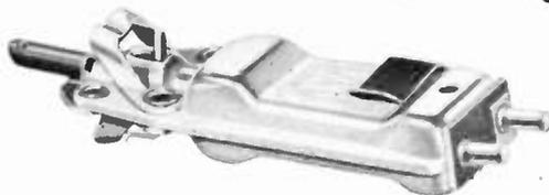
The model F-16 is an all-purpose crystal cartridge employing two separate needles to permit playing both fine-cut and standard records . . . with a single tone arm and three-speed turntable. The cartridge can be rotated 180° in the arm to bring the proper needle into playing position. The model F-16 is a quality cartridge with ideal response characteristics.
