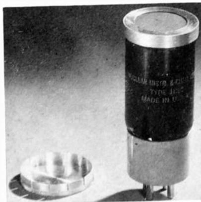
The D31 has a plateau length of 200 to 300 volts, with a slope of only 3 per cent per hundred volts. Threshold voltage is between 1,050 and 1,300 volts, and counting life is at least 10<sup>6</sup> counts.
