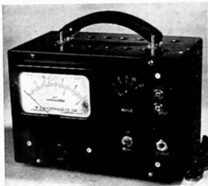
Incorrectly described in our August issue, the Type 100 has an input resistance of 50 ohms and a sensitivity of 1 microampere full scale. Input may be overload 1/4 ampere without damage.
