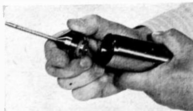
This instrument will directly measure sound pressure from a few to several million dynes/cm<sup>2</sup> in a range from 50 cps to 250 kc. The output signal is delivered by a 25-foot cable at an impedance level of 500 ohms. Extension cables have no appreciable effect on the frequency characteristic of the system.
