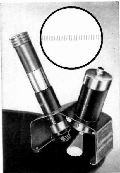
Magnification of either 20 or 40 times is offered. For calculation of lines per inch, width of groove, or groove-to-land ratio, a reticle has been incorporated for direct measurement with divisions of 0.004 inch or 0.002 inch for the respective powers.
