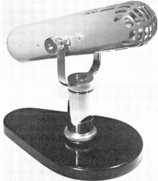
Fig. 18 - The uniaxial microphone mounted on a desk stand.
