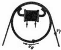
Fig. 3 - The basic principles of rotating playback head by using four playback gaps 90° apart and magnetic commutator.
