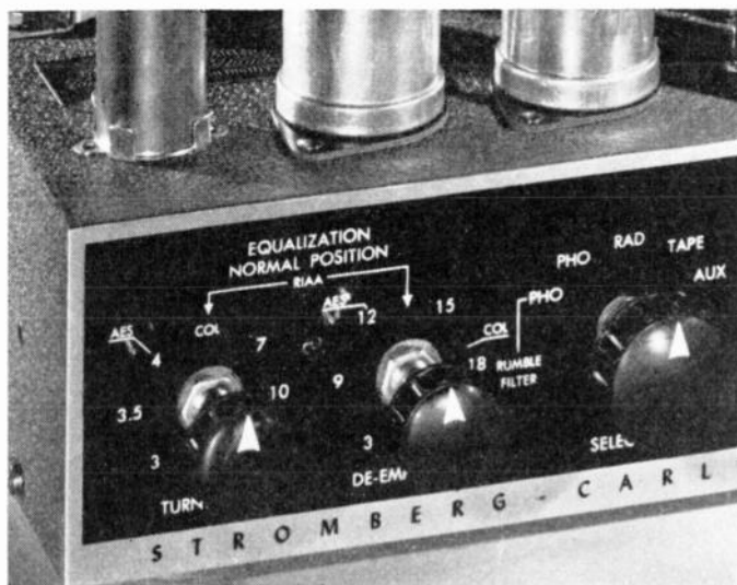
Fig. 2—The AR-420 amplifier, using continuously variable equalization.
