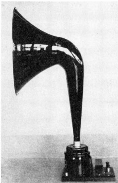
Fig. 2—Photograph of Magnavox R-3 loudspeaker (Pridham and Jensen, 1921).
