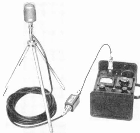
Fig. 2—Altec Type 633 Dynamic Microphone shown mounted on a tripod with connecting cable to a microphone-to-grid transformer connected to the input of a sound-level meter.
