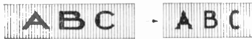
(a) ANALOGY OF SIGN PAINTED ON BOARD FENCE. DISCARDING EVERY OTHER BOARD AND PUTTING REMAINDER TOGETHER STILL LEAVES IT READABLE
