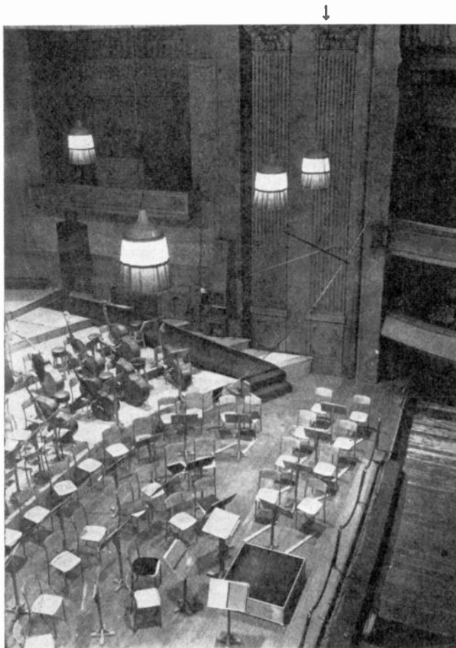
Fig. 5—The stage in the "Gebouw voor Kunsten en Wetenschappen" in The Hague. The line microphone (rod with ten condenser microphones) is indicated by two arrows. (Other microphones visible in the photograph were for broadcasting and had nothing to do with stereo reverberation.)
