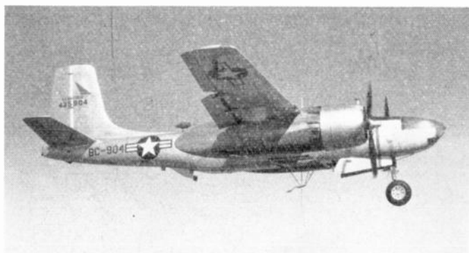
Fig. 12—B-26 in flight with sound system and suspended microphone.
