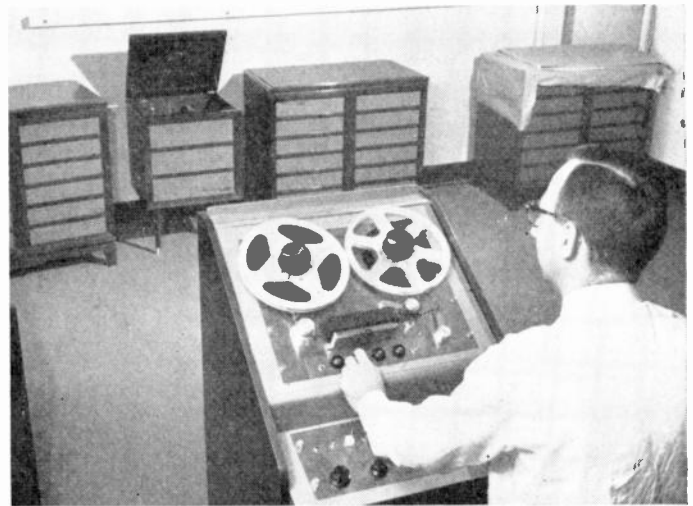
Fig. 3—Special tapes have been made to test loudspeakers. The author is shown using recordings of tone bursts to test the transient response of several loudspeakers. Other tapes contain specially selected passages, such as organ music, for testing low-frequency response, and cymbals and triangles for use in high-frequency tests.
