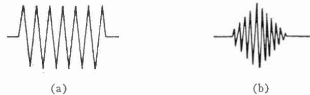
Fig. 17—Example of the reproduction of a sinusoidal wave train by an electrodynamic cone loudspeaker. (a) Wave shape of the sinusoidal voltage applied to the loudspeaker voice coil. (b) Wave shape of the electrical signal produced by a microphone located in front of the loudspeaker.
