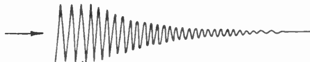
Fig. 19—Decay curve of the sound pressure produced by a loudspeaker, as a function of time, after sudden interruption of the signal (test signal=85 cps). Resonant frequency of the loudspeaker cone = 85 cps. Decay time = about 300 milliseconds.
