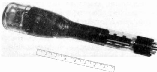
Fig. 1 - The IBM-93 cathode-ray storage tube.
