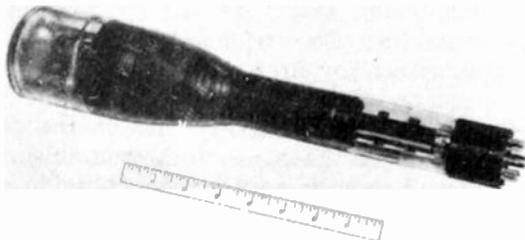
Fig. 1 - The IBM-93 cathode-ray storage tube.
