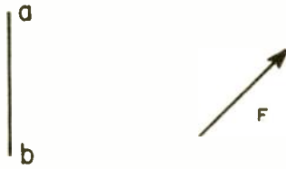
Fig. 1—Electromagnetic waves incident on a wire with electric field intensity vector not parallel to the wire.
