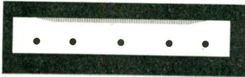
Fig. 11—Actual size reproduction of photographic transparency used in etching halves of slotted wall for space-harmonic traveling-wave tube structure of Fig. 10. The slots are resonant near 66,000 mc.
