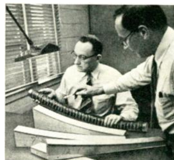
New type waveguide is bent on wooden forms for study of effect of curvature on transmission. The waveguide itself is here covered with a protective coating.
