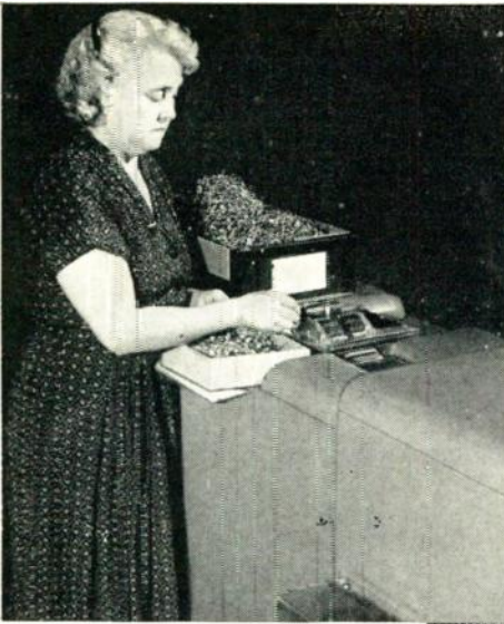
Here rectifiers are automatically tested and inspected in mass quantities.
