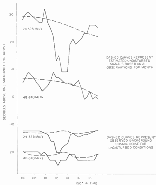
Fig. 31—Signal and background cosmic noise behavior during a polar blackout observed at Barrow on May 19, 1953.
