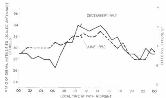
Fig. 18—Diurnal variation of frequency-dependence observed by comparing transmissions at 49.8 and 107.8 Mc/s.
