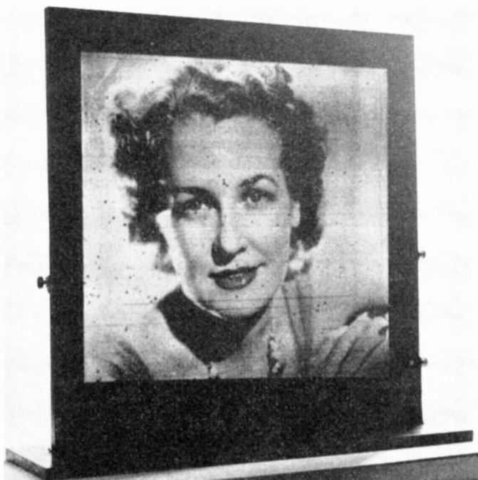
Fig. 7—Photograph of grooved-photoconductor type light amplifier showing amplified picture resulting from a projected image.
