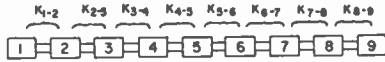
Fig. 2—The general case of a filter having a number of very high- Q resonant elements all tuned to the same frequency and having equal coupling coefficients, K , between adjacent resonant elements.
