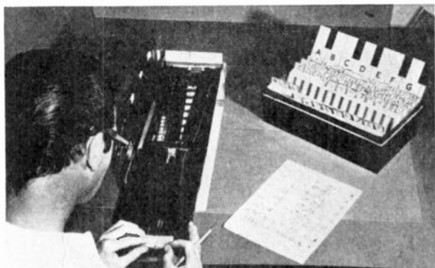
Fig. 18—One of the animated sound techniques developed by Norman McLaren of The Natl. Film Board of Canada. A series of variable density patterns seen in the card file at the right of the figure are photographed through an adjustable mask seen at the left. (Photograph courtesy of The Natl. Film Board of Canada.)
