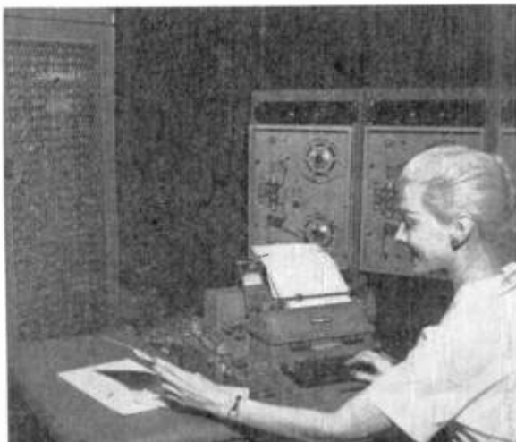
Above —Shown enlarged next to a match is a midget hermetically-sealed electric condenser, \frac{1}{8} " in diameter by \frac{1}{4} " in length, to be used in the miniaturized electronic circuits of guided missiles. Below —This electronic memory system reduces the contents of sixteen thousand conventional file cabinet drawers to less than three cubic feet of space by automatically sequencing, selecting, collating and separating information recorded on magnetic tape. The tape is fed to a companion electronic computer.
