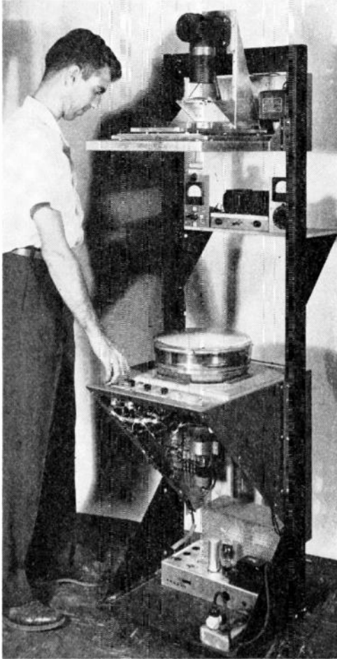
Fig. 7—Optical test stand to check Deflectron circularity.
