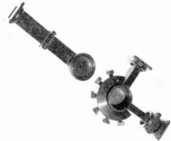
Fig. 6—Circularly-polarized cavity, TE_{112} mode, excited by two linear waves in space and time quadrature. The 1.25-mm ferrite sphere is suspended in exact center by nylon thread.
