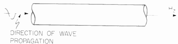
Fig. 12—Infinite plane wave being propagated along axis of an infinitely long magnetized ferrite cylinder.
