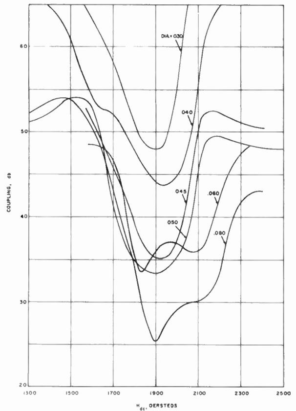
Fig. 8—Coupling vs H_{dc} as a function of diameter. General Ceramics R-1. Frequency, 9000 mc.
