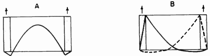
Fig. 3—Electric field patterns for ferrite modes in rectangular waveguide. (Reproduced from Lax and Button. 16,17 )
