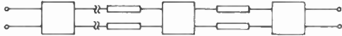
Fig. 13—Generalized circulator composed of alternate directional couplers and pairs of nonreciprocal transmission lines.
