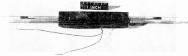
Fig. 8—Ferrite isolator with coil to vary the magnetic field.
