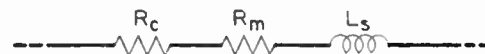
Fig. 8—Representation of core loss R_m as a series resistance. R_c = winding resistance; R_m = effective series resistance due to magnetic core; L_s = series inductance; R_s = R_c + R_m = effective resistance of inductor;
