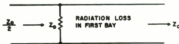
Fig. 8 Impedance matching for probe.
