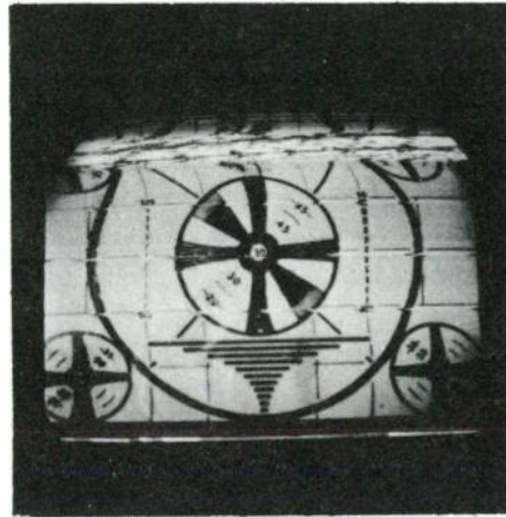
Fig. 5 Picture monitor displaying the signal of Figure 4 showing resultant tearing and pulling.
