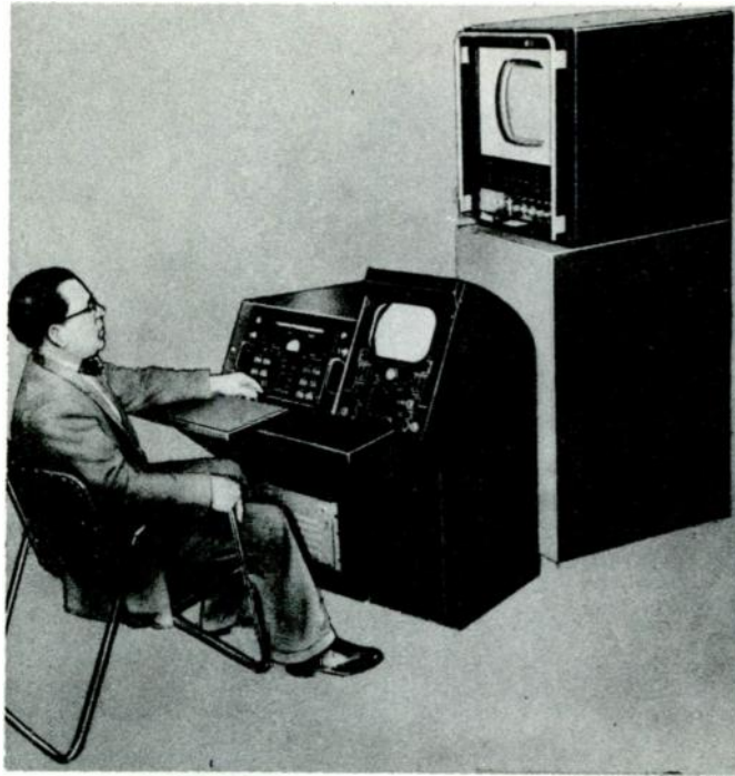
Fig. 5 Color camera control console and color monitor
