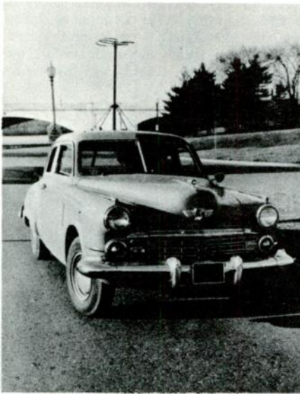
Fig. 7 TV Receiving Antenna and Field Car
