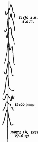
Fig. 12—Three-helix lobe-sweeping array patterns obtained during transit of source on March 14, 1957. Horizontal chart width corresponds to lobe displacement of  $20^\circ$  either side of meridian (vertical line). East of the meridian is to the right and west to the left.
