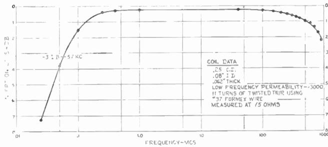
Fig. 10—1:1 Reversing transformer. Insertion loss vs frequency.
