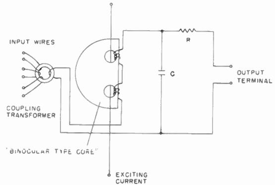
Fig. 20—The circuit of a parametron with a "binocular type core" and a series type coupling transformer.
