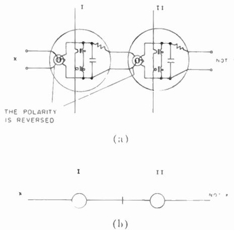
Fig. 9—(a) A “not” circuit. (b) The schematic diagram of the “not” circuit (a).
