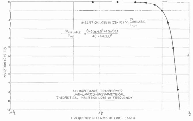
Fig. 16—Theoretical insertion loss vs frequency.
