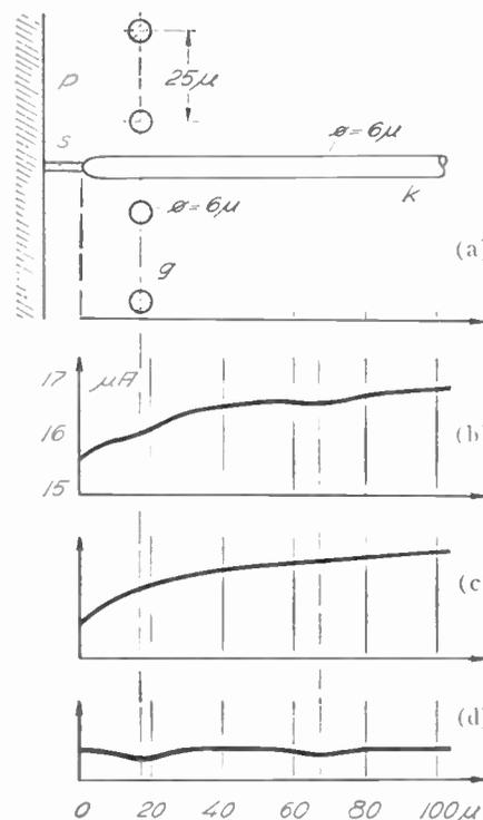
Fig. 1—Electrode arrangement and essential dimensions. Further, the relationship between the avalanche current and the position of the grid is shown.
