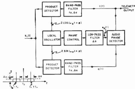
Fig. 2—Sideband (DSB) phase-lock system.
