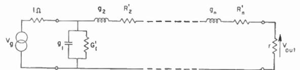
Fig. 3—Dissipative low-pass prototype filter.
