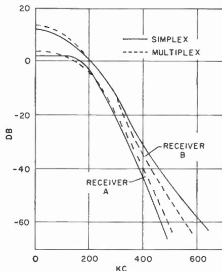
Fig. 2—Permissible signal-to-interference ratio (for three per cent cross talk) as a function of carrier separation.
