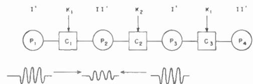
Fig. 15—Coupling system for two-subclock excitation.
