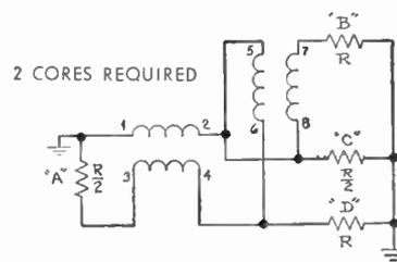
Fig. 8—Hybrid with equal conjugate impedances. Each arm single ended.
