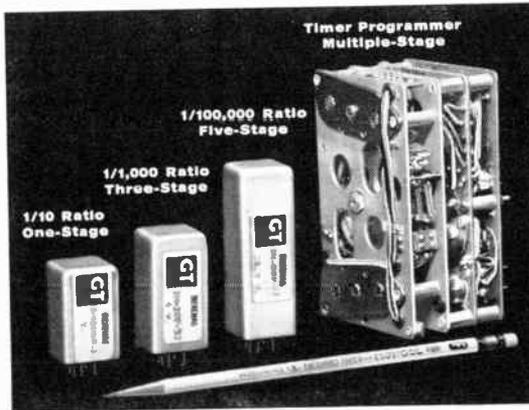
Max. counting rate: 100,000 pps, Max. counts per stage: 16. As many stages as required. ±15% voltage tolerance, -55°C to +125°C temp.
