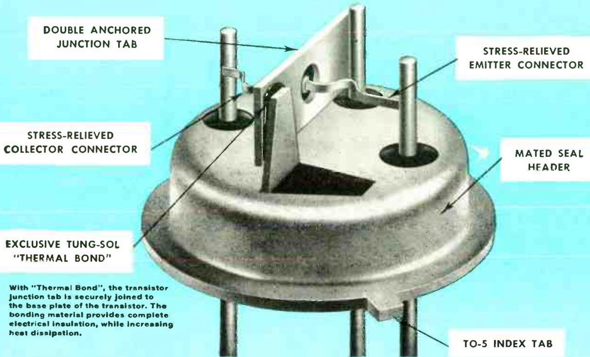
With "Thermal Bond", the transistor junction tab is securely joined to the base plate of the transistor. The bonding material provides complete electrical insulation, while increasing heat dissipation.
