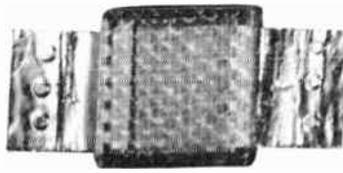
**High temperature capacitor** New high temperature dielectric. Up to 10,000 uuf. DCWV of 300 V at 300°C. Q better than 500 at 300°C. Especially suitable for missiles and aircraft. Highly resistant to nuclear radiation.
