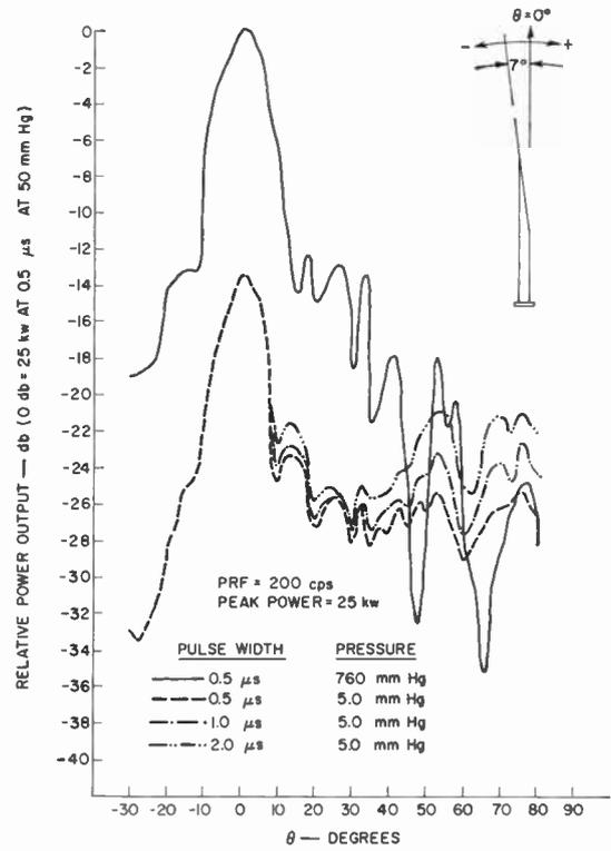
Fig. 10—*E*-plane radiation pattern for 20-dB traveling-wave antenna under breakdown conditions.
