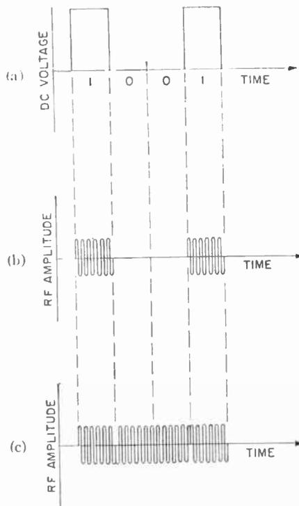
Fig. 5—Three types of script to represent binary information. (a) DC pulse script, (b) RF pulse script, (c) RF phase script.
