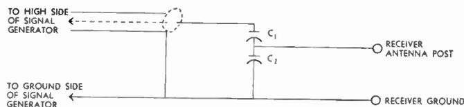
Fig. 3—Capacitance divider connections for simulated antenna.
