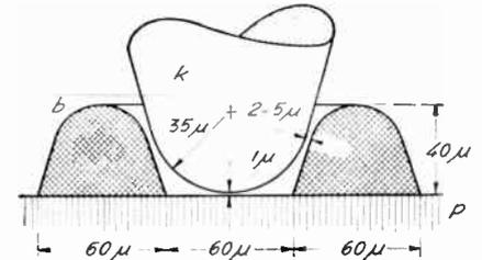
Fig. 2—A corona discharge results in the formation of a circular embankment  $b$  fastened on the anode  $p$  and surrounding the cathode  $k$ .
