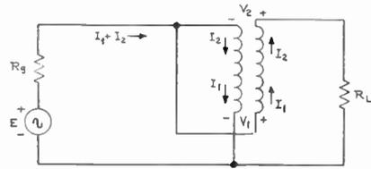
CHARACTERISTIC IMPEDANCE OF BIFILAR WINDING =  $Z_0$
