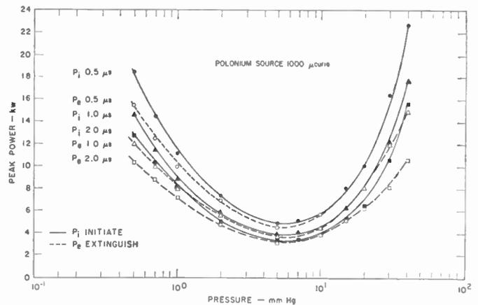
Fig. 3—Breakdown power as a function of pressure for a 20-db X-band traveling-wave slot antenna.
