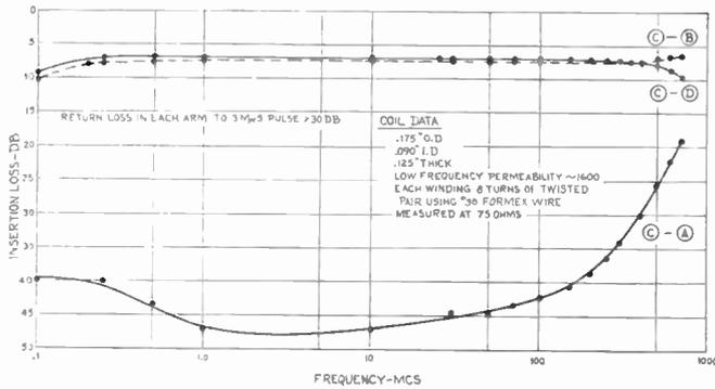
Fig. 14—Matched resistance hybrid. Insertion loss vs frequency.
