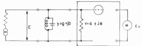
Fig. 13—Susceptance neutralization.
