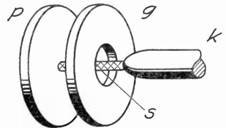
Fig. 6—Suggested arrangement for high impedance control of the current in a small semiconductor element  $s$  between an anode  $p$  and a pointed cathode  $k$ ,  $g$  being the control electrode.
