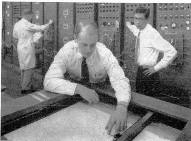
**ANALOG COMPUTER** installation used to simulate missile trajectory, ground control and terminal guidance. Boeing missile assignments are available on BOMARC, the nation's longest-range supersonic defense missile, and on Minuteman, an extremely advanced solid-propellant intercontinental ballistic missile system.
