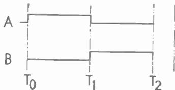
**-hp- 219C Digital Pulse Duration Unit** produces a high power pulse with digitally controlled delay and duration. Pulse duration either  $T_0$  to  $T_1$ , or  $T_1$  to  $T_2$ . Both polarities available simultaneously; amplitude variable 0 to 20 v (from 90 ohms impedance) or 100 v (from 500 ohms). Rise or decay time 0.03  $\mu$ sec (90 ohms). \$350.00.
