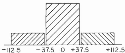
Fig. 4—Sweep pattern with fifty per cent each on audio and 75-kc subcarrier.
