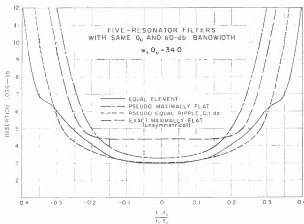
Fig. 5—Pass-band insertion-loss curves for four different five-resonator filter designs.
