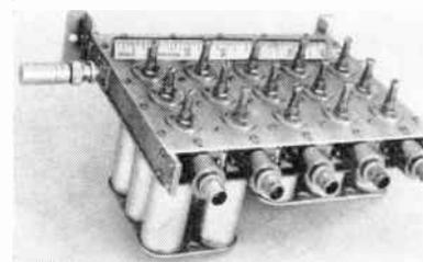
Figure 4—480-1000 Mc., 5 channels (5 1/2 x 7 3/8 x 3 3/4 inches, 2 lbs.)
