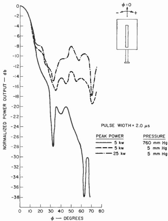
Fig. 8—Normalized *H*-plane radiation pattern of 20-dB traveling-wave antenna under breakdown conditions.
