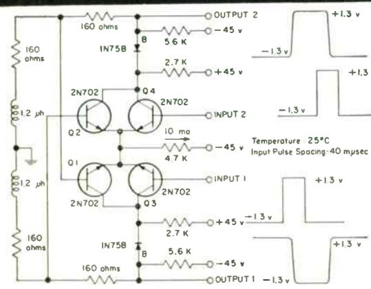
TYPICAL CIRCUITRY FOR OBTAINING 25-MC REP RATE IN NON-SATURATED FLIP-FLOP
