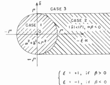
Fig. 22—Classification of the three cases of singular points in  $(\alpha, \delta)$  plane.
