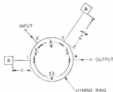
Fig. 9—Circuit for separating input and output of subharmonic oscillators. A = subharmonic oscillator.
