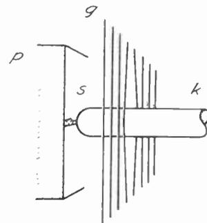
Fig. 5—Evidence of the generation of submillimeter waves is obtained by this arrangement, in which  $k$  is a tungsten cathode, diameter 30 microns;  $s$  is a particle from an embankment;  $p$  is an anode; and  $g$  is a grid consisting of gold-plated tungsten wires, diameter 5 microns, stretched with a c-c distance of 25 microns. The grid  $g$  may be slid along the cathode  $k$  by means of a micromanipulator.
