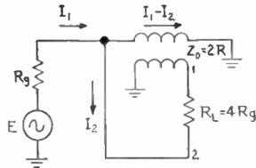
Fig. 5—Balanced—unbalanced 4:1 impedance transformer.
