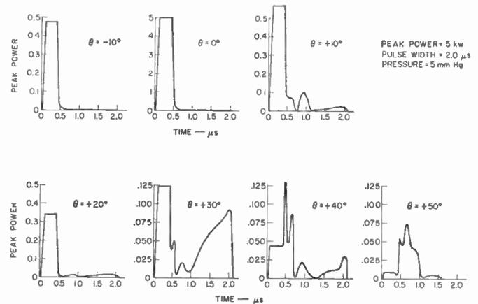
Fig. 13—Pulse shapes radiated by 20-db traveling-wave antenna under breakdown conditions.
