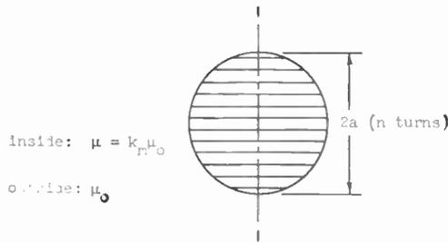
Fig. 7—Spherical inductor.
