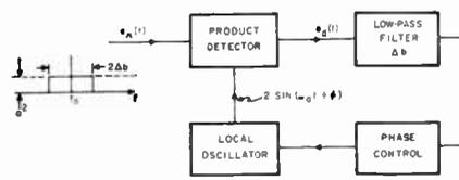
Fig. 1—Carrier-lock system.
