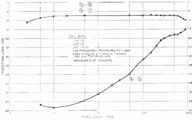
Fig. 13—Hybrid of Fig. 8. Insertion loss vs frequency.
