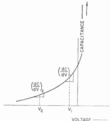
Fig. 2—Capacitance vs voltage characteristic of a diode.
