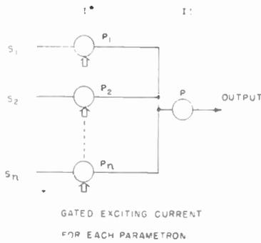
Fig. 17—Channel-selecting circuit using gated excitation.
