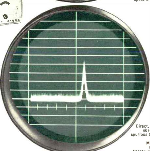
Direct, immediate observation of spurious transmitter radiation.
