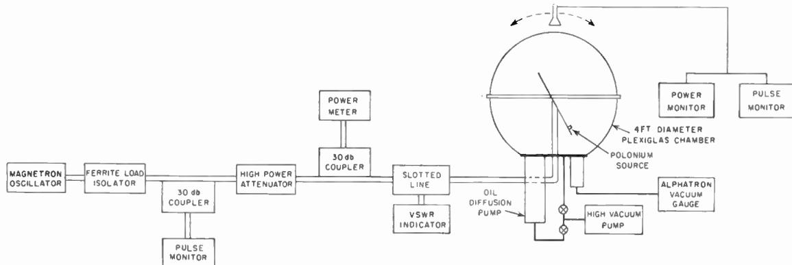
Fig. 1—Experimental set-up used for X-band voltage-breakdown measurements.
