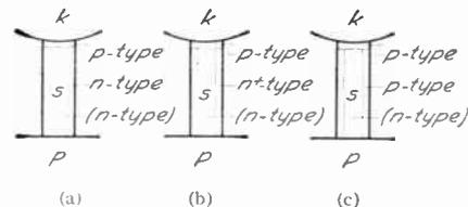
Fig. 6—Variations in surface states by changes of surrounding gas ambients. The embankment particle  $s$  is placed between a cathode  $k$  and an anode  $p$ .
