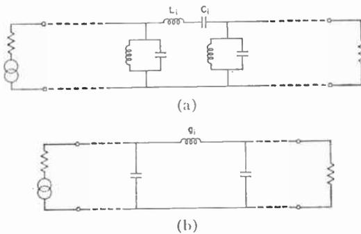
Fig. 7—(a) Nondissipative lumped-constant band-pass filter, and (b) equivalent low-pass prototype filter.
