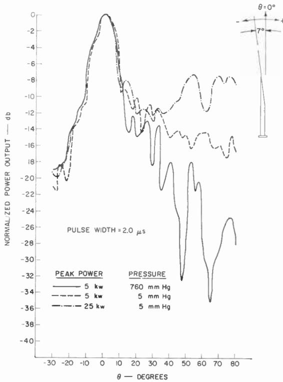
Fig. 7—Normalized *E*-plane radiation pattern of 20-dB traveling-wave antenna under breakdown conditions.
