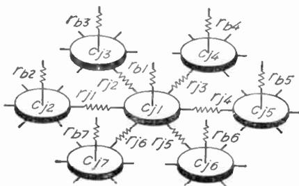
Fig. 4—Semiconductor capacitances and resistances at reverse bias.
