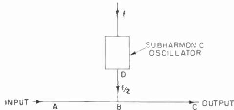
Fig. 8—Circuit used for forced switching with gain.
