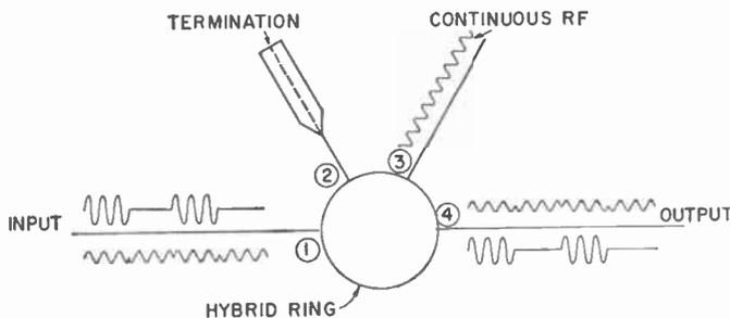
Fig. 6—Hybrid circuit for converting pulse script to phase script, or vice versa.
