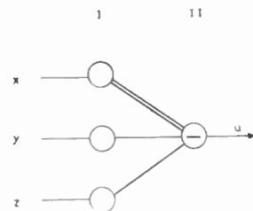
Fig. 14—A circuit for "x and (y or z)."
