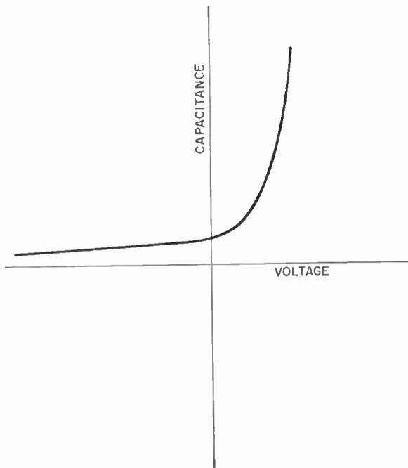
Fig. 2—Typical diode capacitance-voltage characteristics.
