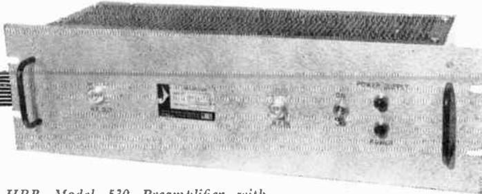
HRB Model 530 Preamplifier with power supply in relay rack mounting enclosure.
