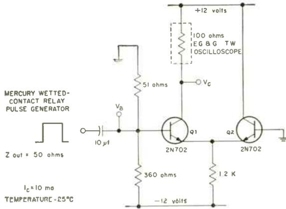
TYPICAL NON-SATURATED LOGIC SWITCHING CIRCUIT
