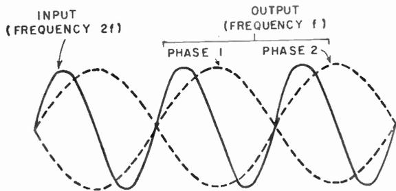
Fig. 4—Two equally probable output phases which can be generated by a subharmonic oscillator.
