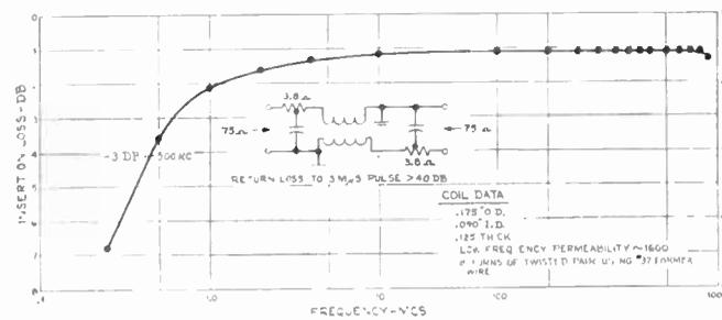
Fig. 11—Matched reversing transformer. Insertion loss vs frequency.
