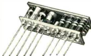
This shows still another type module packaging which uses A-B Type CB 1/4 watt composition resistors.
