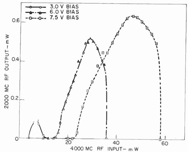
Fig. 3—RF power output vs RF power input for subharmonic oscillator.
