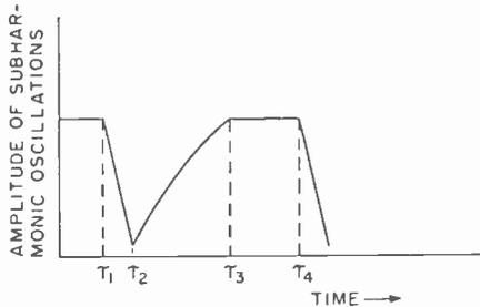
Fig. 7—Diagram illustrating the application of subharmonic oscillators to the amplification of trains of binary digits coded in RF phase script.
