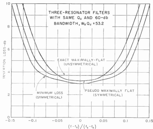
Fig. 4—Pass-band insertion-loss curves for three different three-resonator filter designs.
