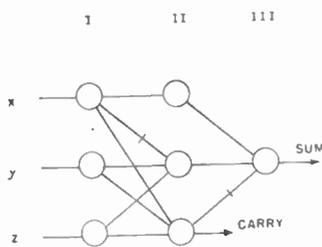
Fig. 12—A binary full-adder circuit.
