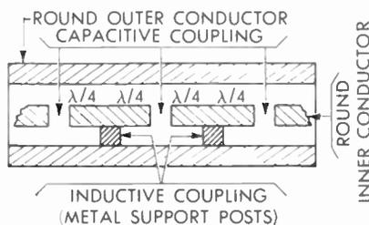
Figure 2—Four axially aligned resonators (cross-section)
