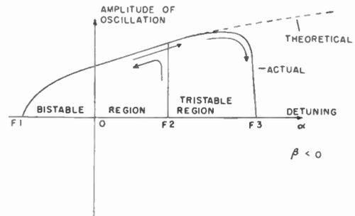
Fig. 25—Amplitude to detuning characteristic of a parametron.
