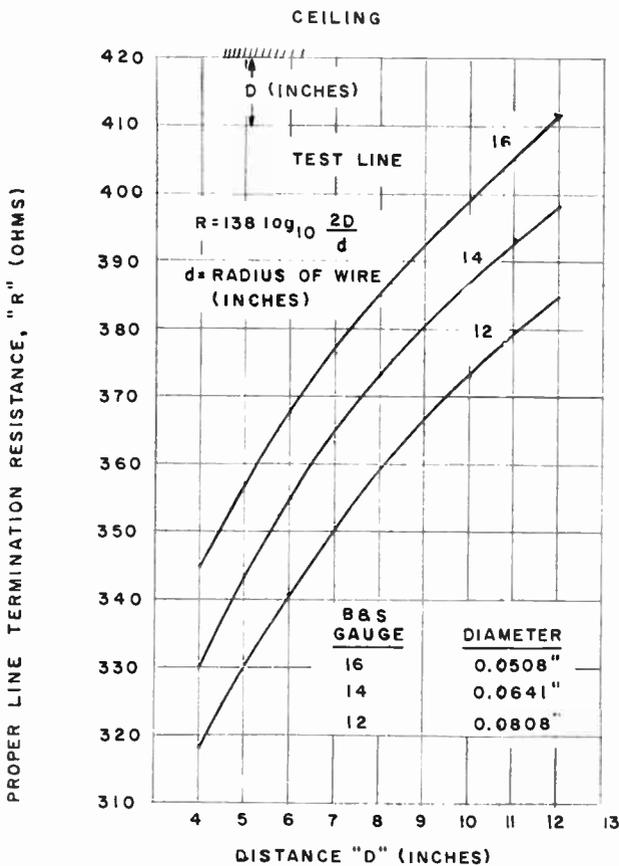
Fig. 2—Terminating resistance for test line.
