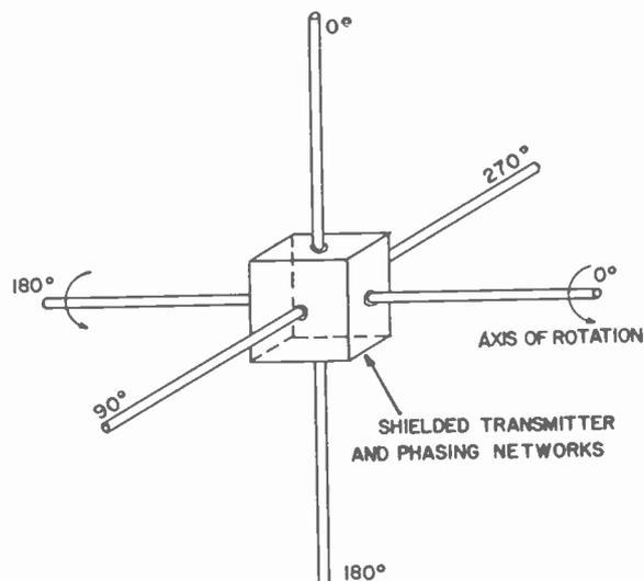
Fig. 8—Transmitter for determining standard wave error.
