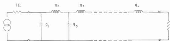
Fig. 2—Nondissipative low-pass prototype filter.
