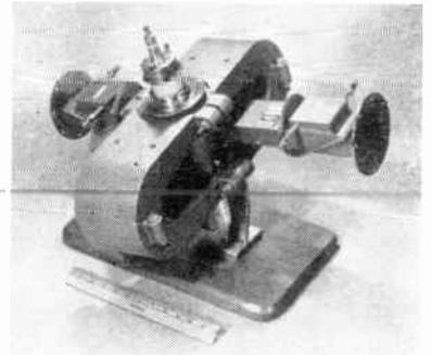
The QK622 can be operated at reduced peak power level to serve as a driver stage. High efficiency is retained at a peak power output of 600 kw and gain of 10 db.
