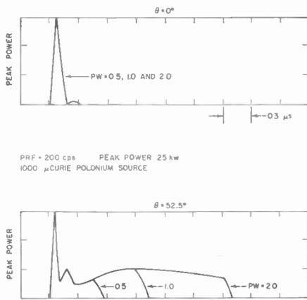
Fig. 11—Pulse shapes radiated by 20-db traveling-wave antenna under breakdown conditions.
