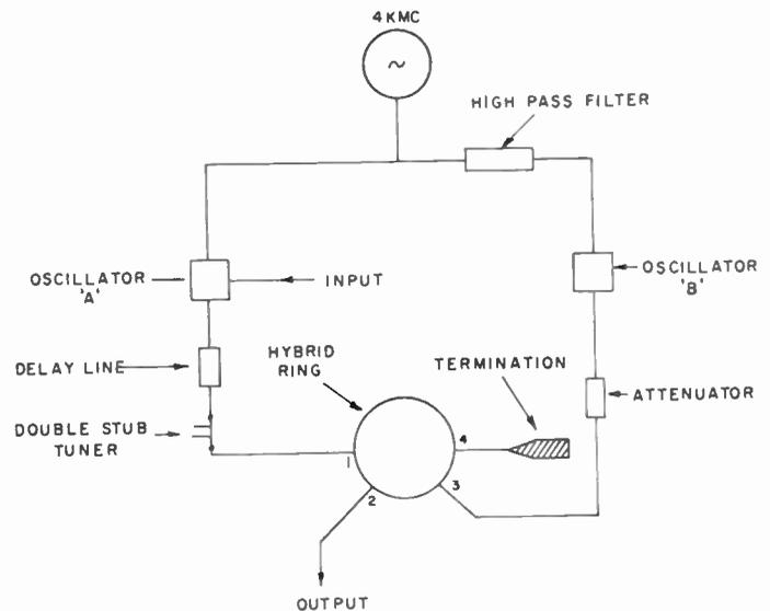
Fig. 11—Schematic diagram of scale-of-two circuit.
