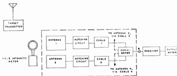
Fig. 4—Typical "DF antenna system."
