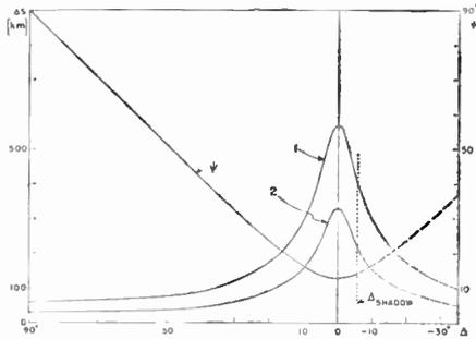
Fig. 2.—Absorption path length  $\Delta s$  and reflection angle  $\psi$  as a function of the elevation angle  $\Delta$ ;  $h_A = 40$  km,  $h_L = 250$  km,  $R_{eff} = 7972.5$  km. Absorbing layer: 1) 60–120 km. 2) 60–90 km.
