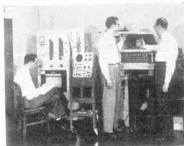
The impetus for this module cooling test fixture development came during the revision of MIL-E-19600A (Aer) specification for the Bureau of Aeronautics, under a U. S. Naval Air Development Center contract. The need for a new type of test equipment for simulating flight operational conditions was foreseen for the development of modules in order to predict the penalty on the airframe in terms of amount and inlet temperature of the cooling air supplied by the airframe.
