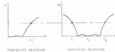
Fig. 1—Correspondence between low-pass prototype response and equivalent band-pass response.
