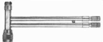
Used to optimize the power output of microwave oscillators by matching the impedance of the source and the load; to tune out reflections in a coaxial transmission system; to maintain a low VSWR on a transmission line for maximum power transfer within a system; as an impedance transformer; to provide a DC return for crystal holders or other devices where DC returns are needed.
