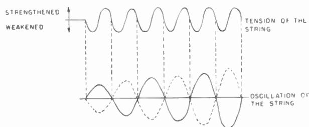
Fig. 2—Build up of oscillation of the string.
