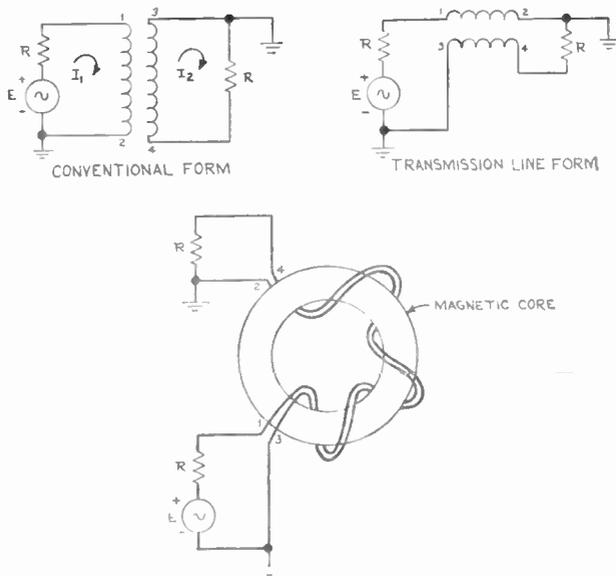
Fig. 1—Reversing transformer.
