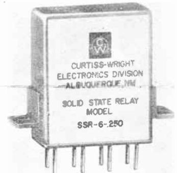
Known as Model SSR-6-250, this unit has a pickup time of 2 microseconds and a dropout of 5 microseconds. First of a complete line of 6, 12, and 28 volts relays, the device can withstand shocks of 1000 g. The relay may be used as a current limiting device to protect power sources from over loads.
