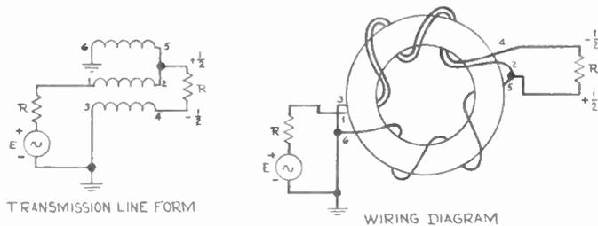
Fig. 2—Unbalanced to balanced transformer.
