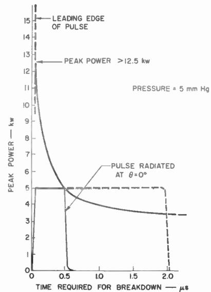
Fig. 12—Time required for breakdown as a function of peak power for 5 mm Hg pressure.
