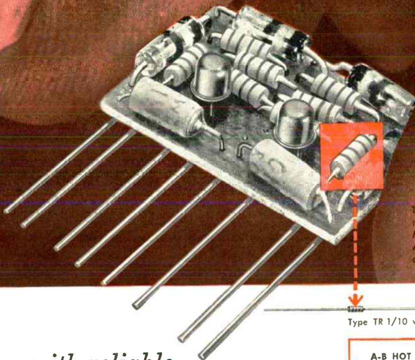
This microminiature binary divider module made by the Cleveland Metal Specialties Co. packs eight A-B Type TR resistors and nine other parts into 0.077 cu. in.!
