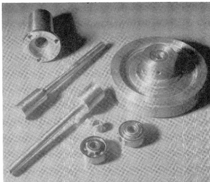
Fig. 6—A closeup view of the stabilizer flywheel and drum assembly parts. The bearings support, shown in the upper left-hand corner, was machined from a solid piece of cold-rolled steel. A hole was drilled through the center for mandrel shaft clearance. The bearing support was then mounted on a mandrel and turned between centers for the outside shoulder and the inside bearing race surfaces. In the photograph, the upper mandrel shaft and stabilizer drum was first made by joining two pieces with heat, but proved unsatisfactory since concentricity could not be maintained in the process. The lower shaft and drum was machined from a solid piece and turned in a lathe between centers where it maintained very close tolerances. The little collar is placed on the mandrel shaft between the rear bearing race and the flywheel proper, as a spacer. The flywheel was machined all over from a solid bronze casting, drilled and tapped for a 5-40 Allen set screw.
