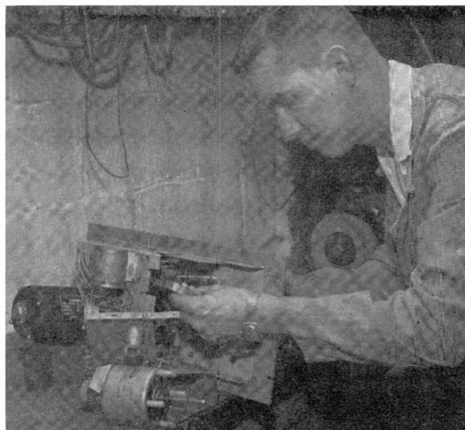
Fig. 7—The author mounting the flywheel on the mandrel shaft of the modified Magnecord PT63AH tape transport mechanism. The extension bracket on the erase-bias oscillator can be seen. The rewind motor assembly was dismounted during the modification process to permit access into the machine superstructure.
